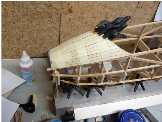
Left: Basic fuselage construction starts on the 'Bridson' jig. | Right: Top decking of the nose comprises off planks of 1.5mm ply.
