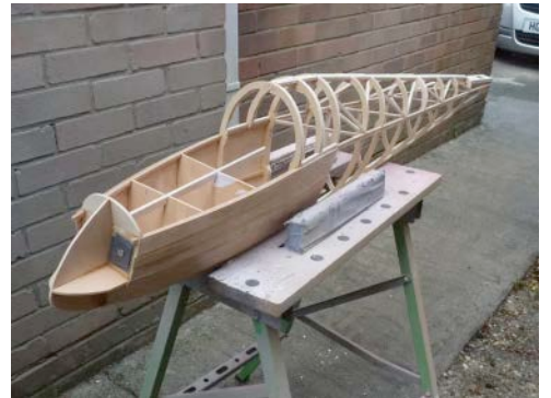
Left: View of the tailplane mount. | Centre: Basic tailplane assembly. | Right: Inner fuselage structure completed, now for all the plywood skinning The temporary formers have yet to be removed.
