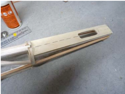
Left: View of the tailplane mount. | Centre: Basic tailplane assembly. | Right: Inner fuselage structure completed, now for all the plywood skinning The temporary formers have yet to be removed.
