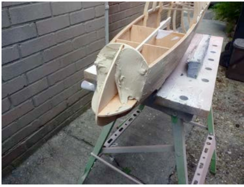
Left: The nose block is made up from polyester filler. | Centre: The front end complete and smoothed with filler. The temporary formers will be removed and the interior glassed with wing joiner tape and polyester resin. | Right: The components of the joiner box for the fuselage.
