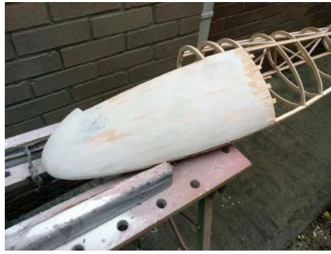
Left: The nose block is made up from polyester filler. | Centre: The front end complete and smoothed with filler. The temporary formers will be removed and the interior glassed with wing joiner tape and polyester resin. | Right: The components of the joiner box for the fuselage.
