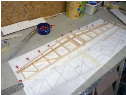
Left: View of the tailplane mount. | Centre: Basic tailplane assembly. | Right: Inner fuselage structure completed, now for all the plywood skinning The temporary formers have yet to be removed.
