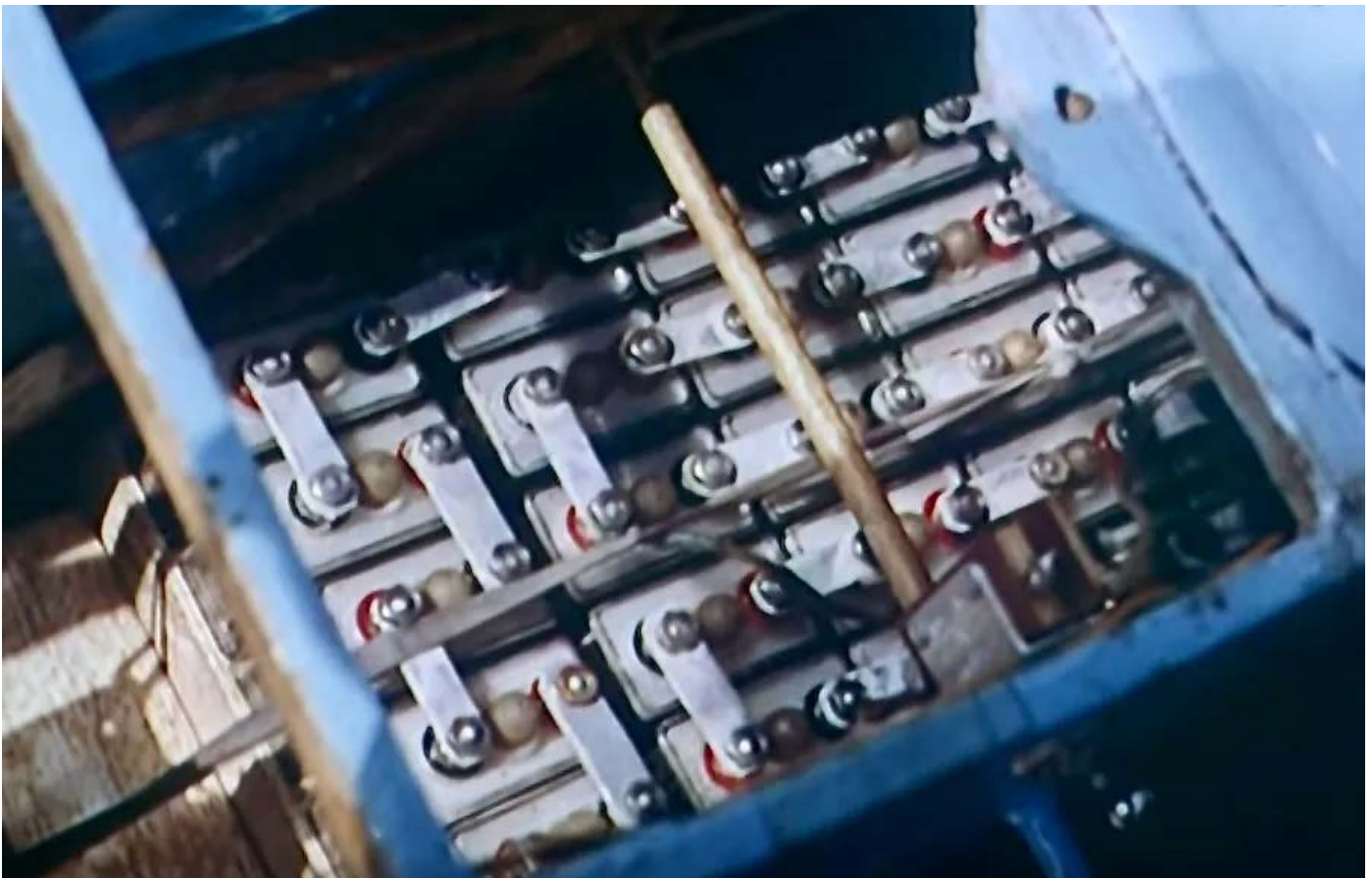
Twenty-five silver zinc cells powered Taplin's 'Radio Queen'. (credit: British Pathé)
