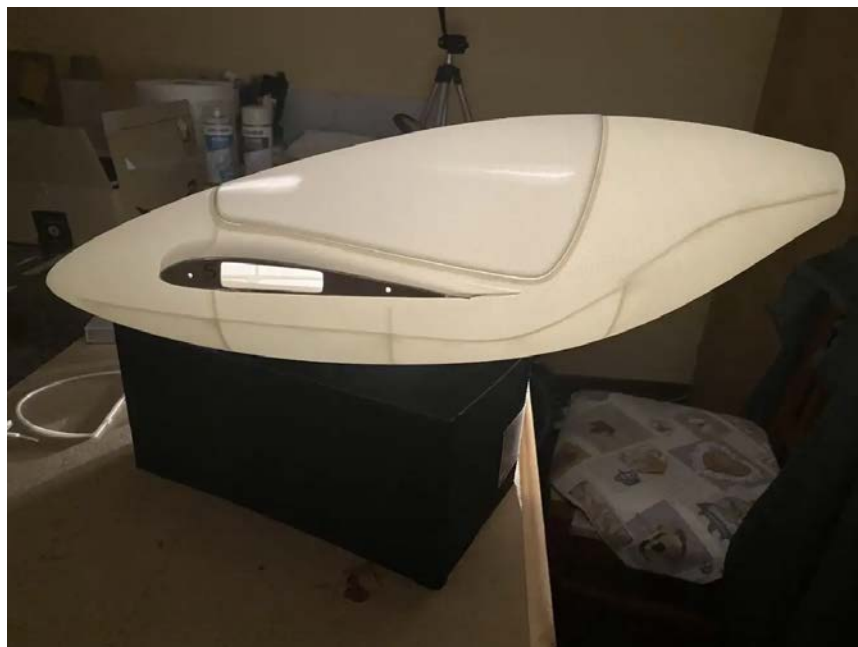
Internal stiffening structure components, as printed and glued inside the fuselage.
