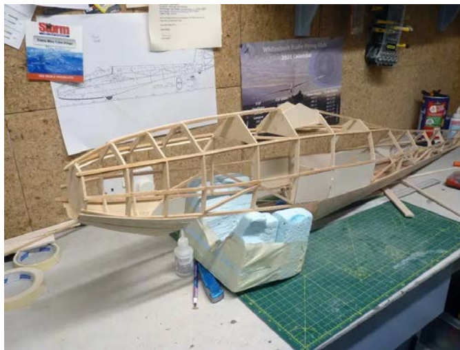
Left: Basic fuselage construction starts on the 'Bridson' jig. | Right: Top decking of the nose comprises off planks of 1.5mm ply.
