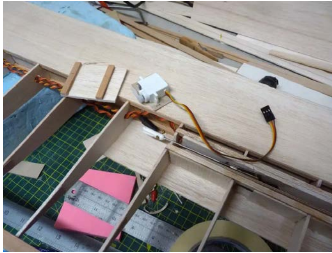
Left: Basic airbrake assembly. | Right: Airbrake installed in the wing.
