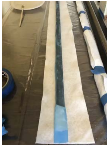
Left: Cutting the spar core. | Centre: Wrapping with glass fibers. | Right: Preparing for vacuum bagging with perforated film and breather.
