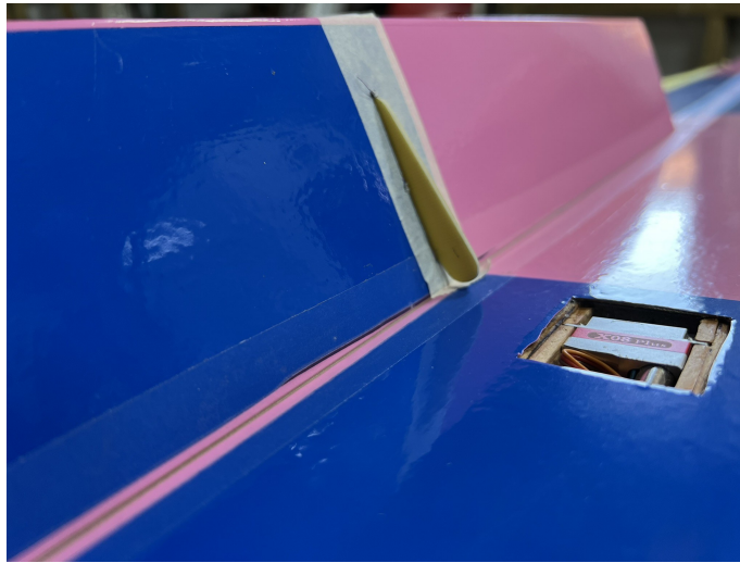
Slot for the horn, full flap travel.
