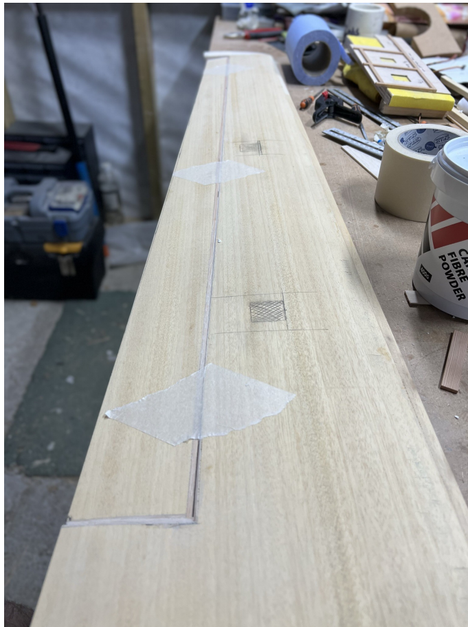
Servo thoughts, Savox out, KST in. Pocket locations transferred to the panel.
