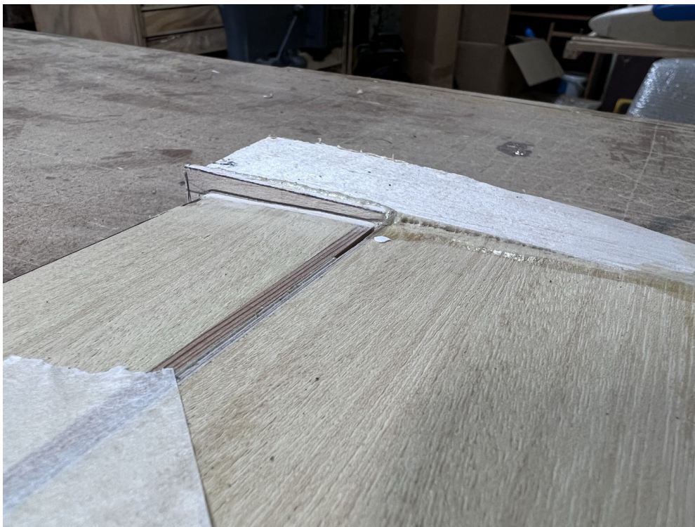
Hardwood false spars, balsa caps and the balsa block tips in place, ready to trim.
