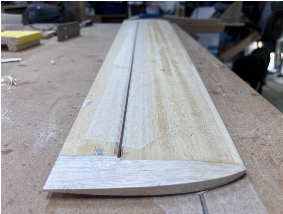
Wing tips joined and shaped. Surfaces cut and capped.
