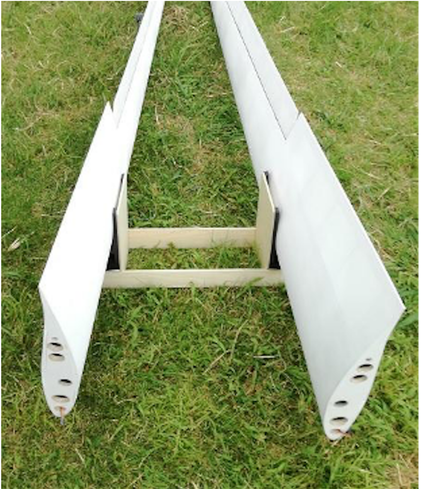
Photo 283: Jig for carrying out wings.
