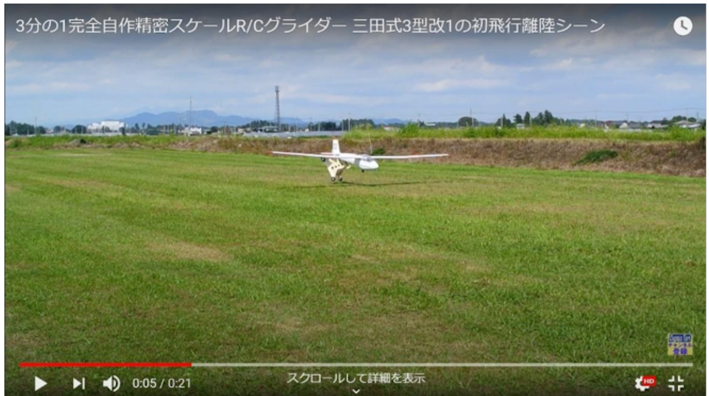
Photo 300-3: The dolly is pulled down and the nose of the aircraft is lowered more and more.
