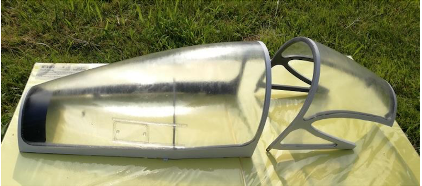
Photo 273: The completed canopy.
