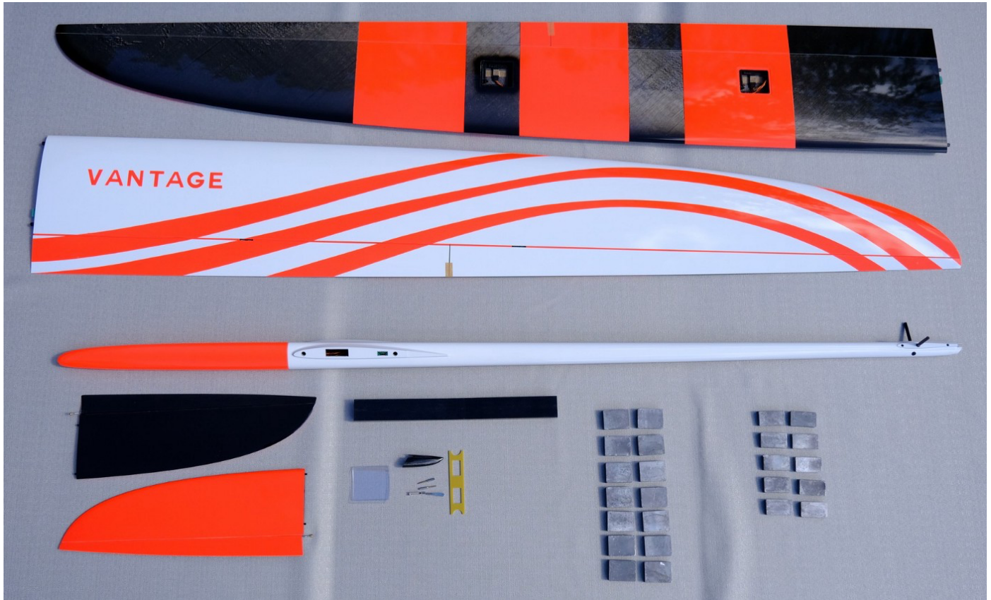
Photo 9: The kit arrives complete and highly preassembled. Just missing the spacers.
