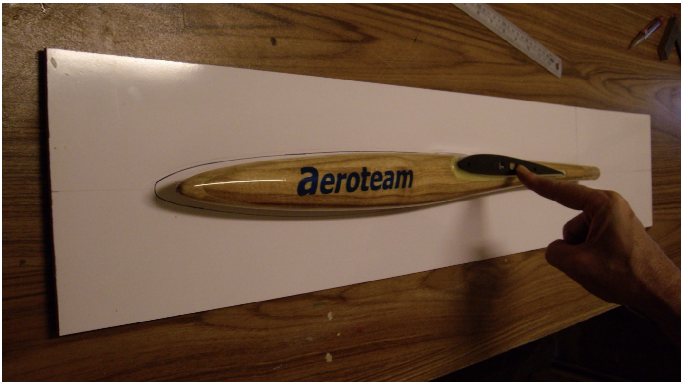
Shinobi fuselage plug is placed on the parting board and the cutting outline has been drawn.
