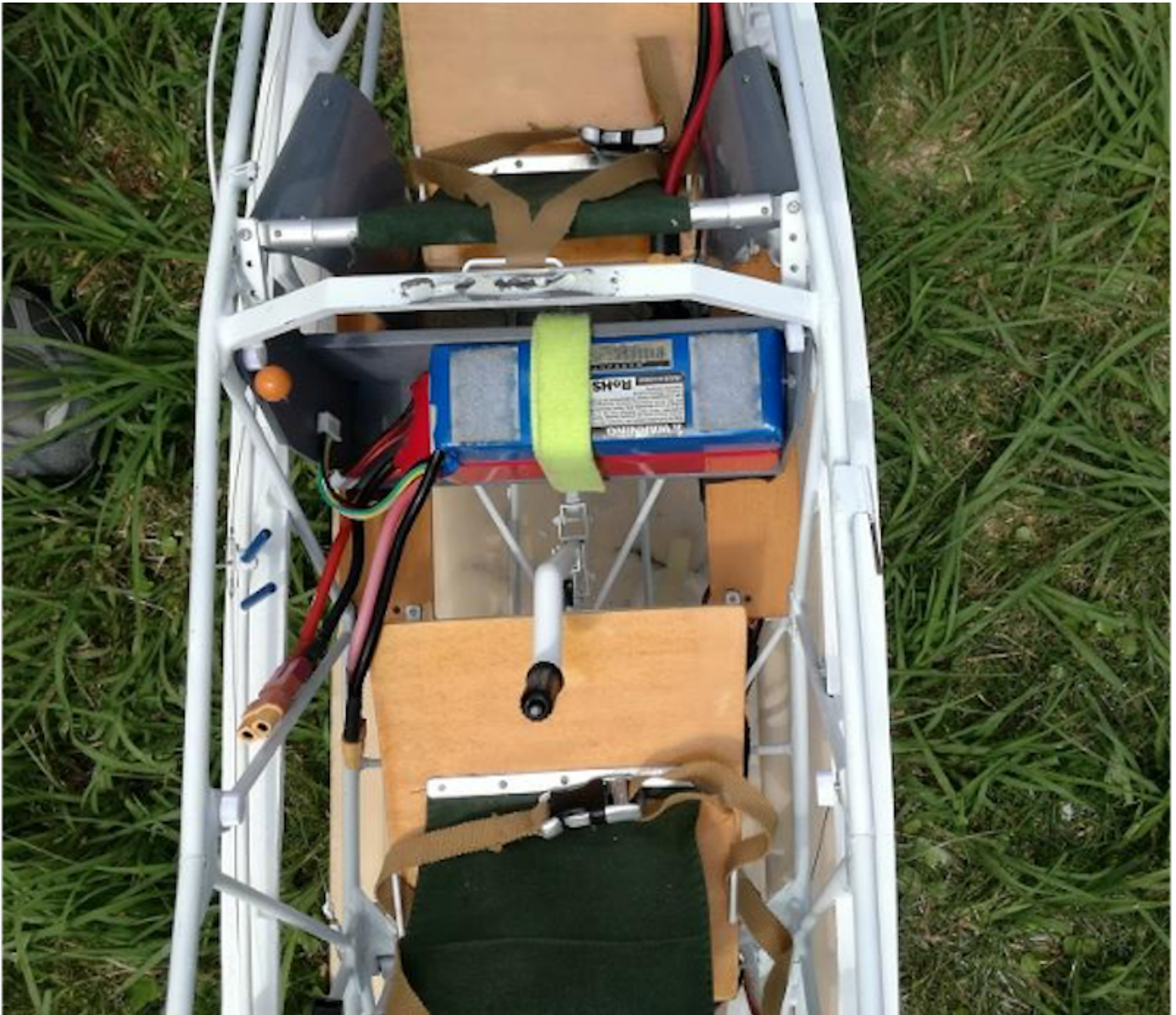
Photo 266: LiPo tray installed: from the side (left), from the top (right).
