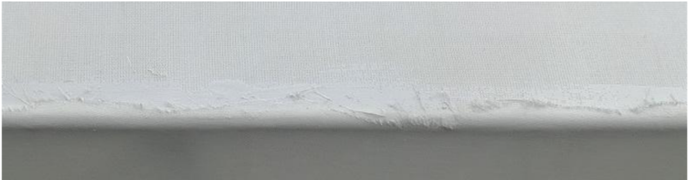
Photo 268: KOVERALL film edge cut with a razor blade.
