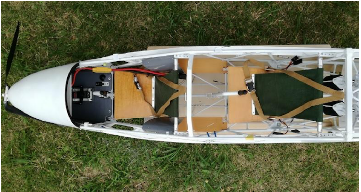
Photo 251: The fuselage with the electrical wiring completed
