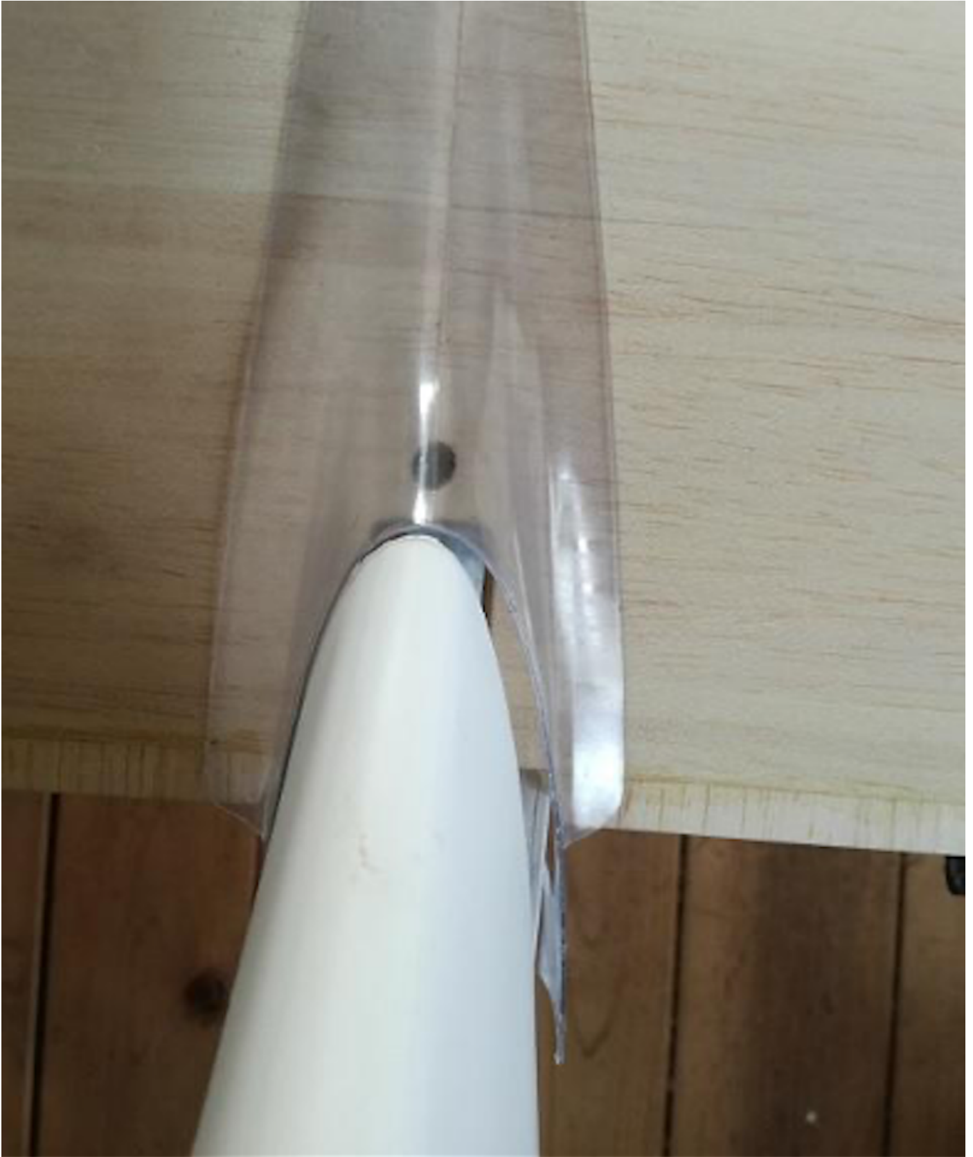
Photo 244: Checking the fit with the vertical tail fin
