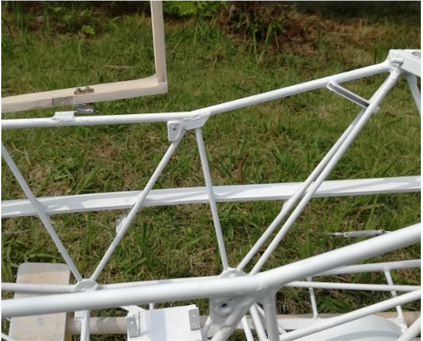
Photo 240: Rear canopy mounting mechanism
