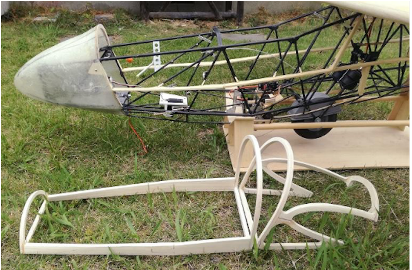
Photo 226: Completed canopy frame
