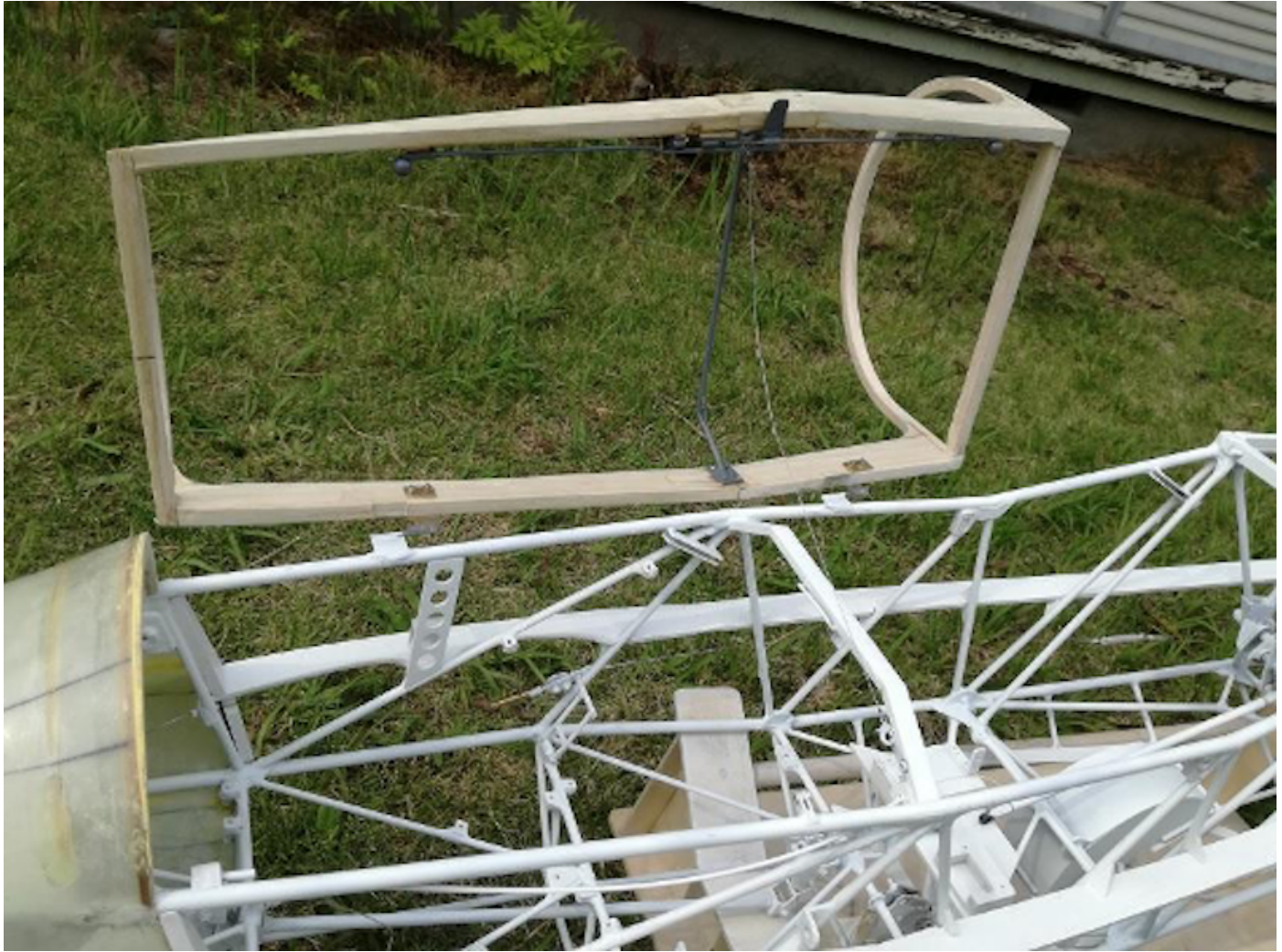
Photo 239: Holding mechanism when the canopy is open
