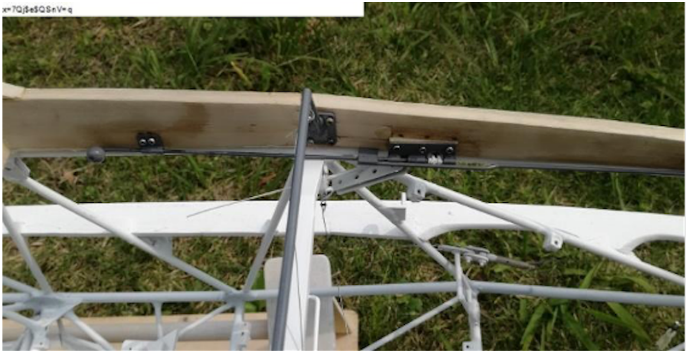
Photo 235: Canopy locking mechanism
