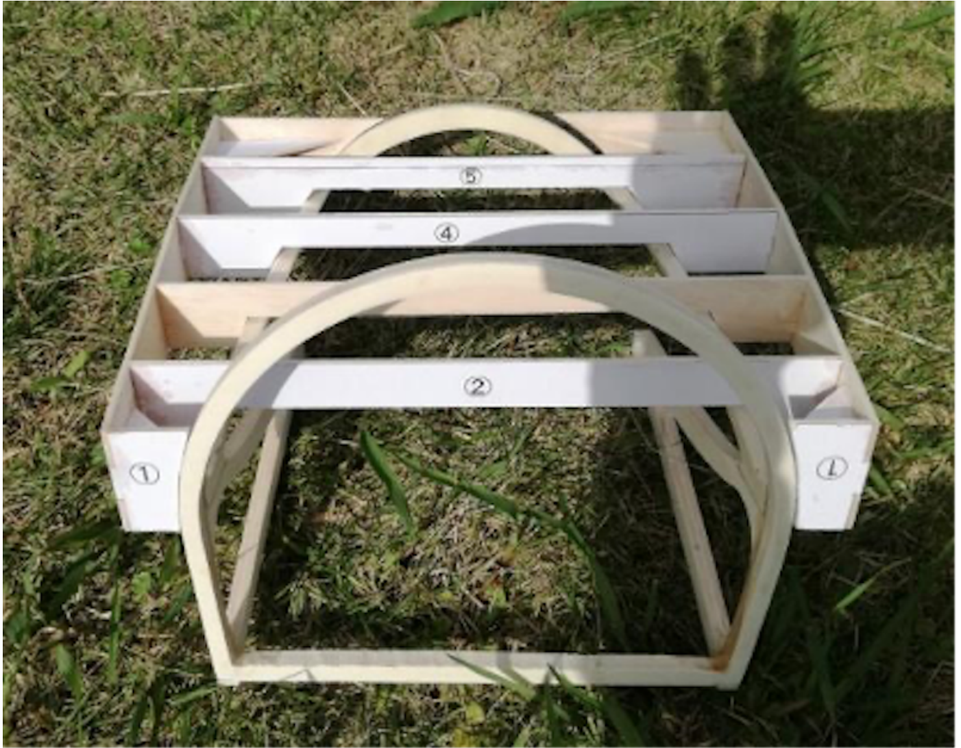
Photo 225: Jig for shaping the longitudinal members of the rear frame
