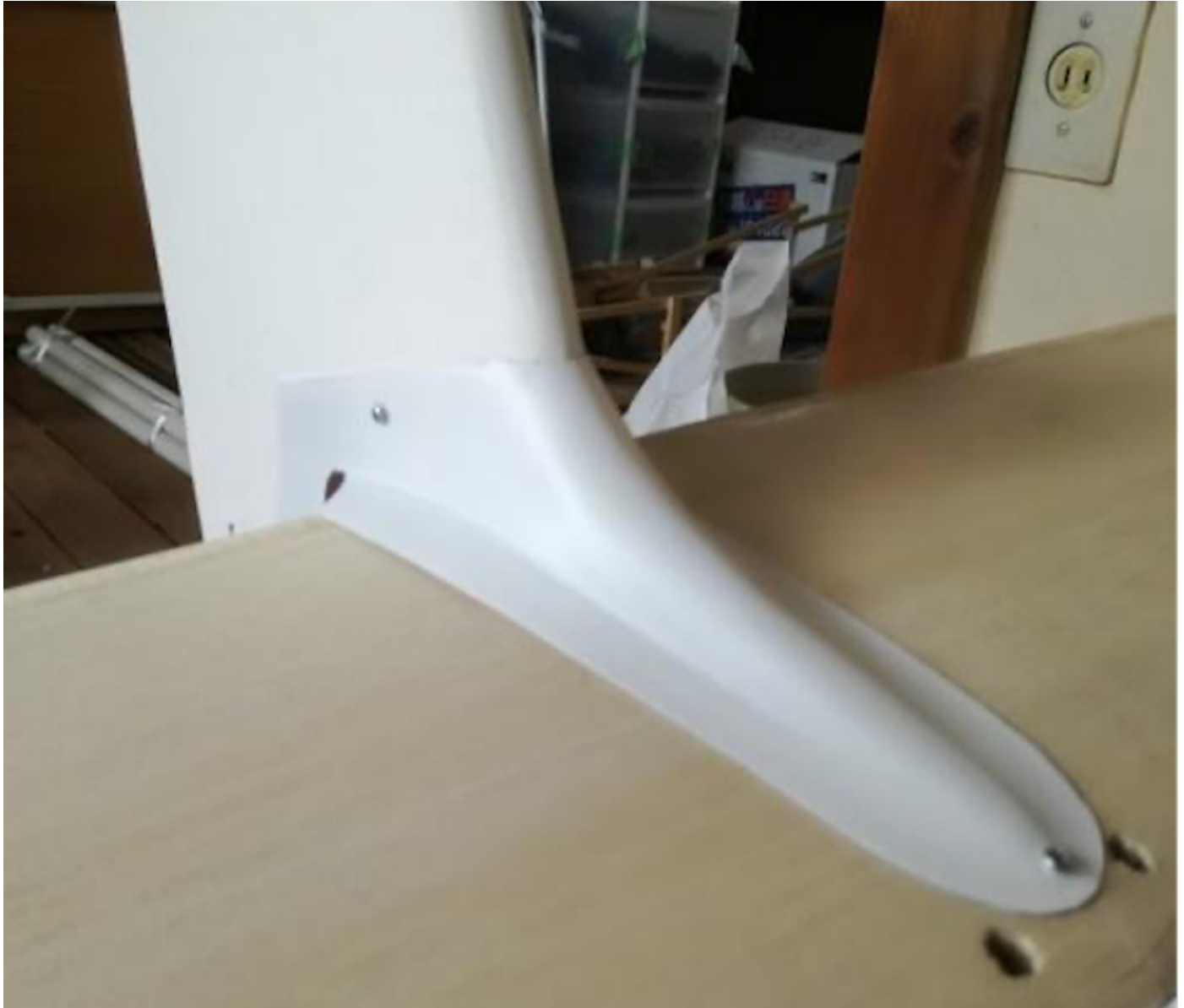
Photo 245: Installation of the tail wing fairing
