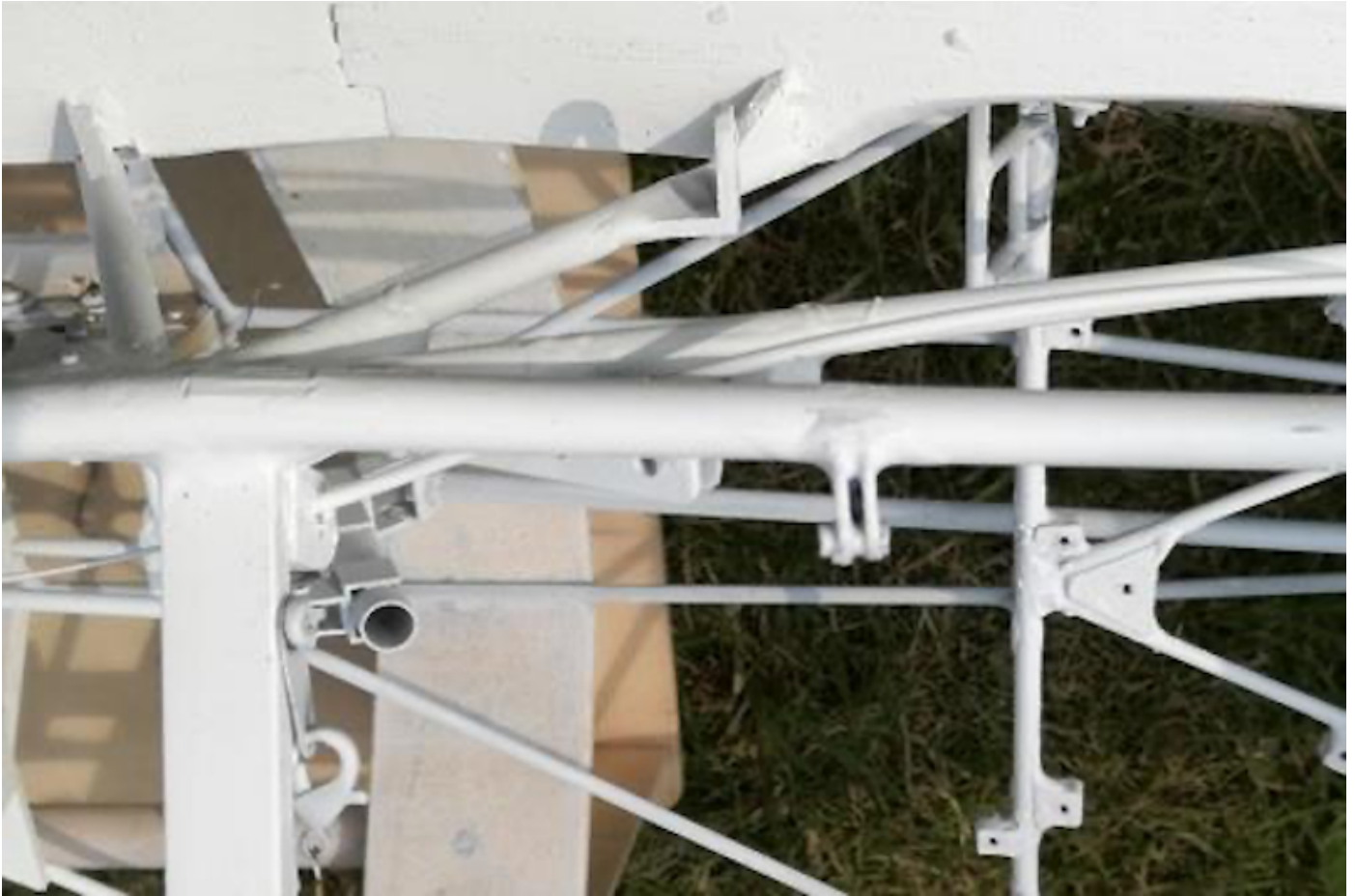
Photo 237: The conduit for the lock mechanism attached to the fuselage side
