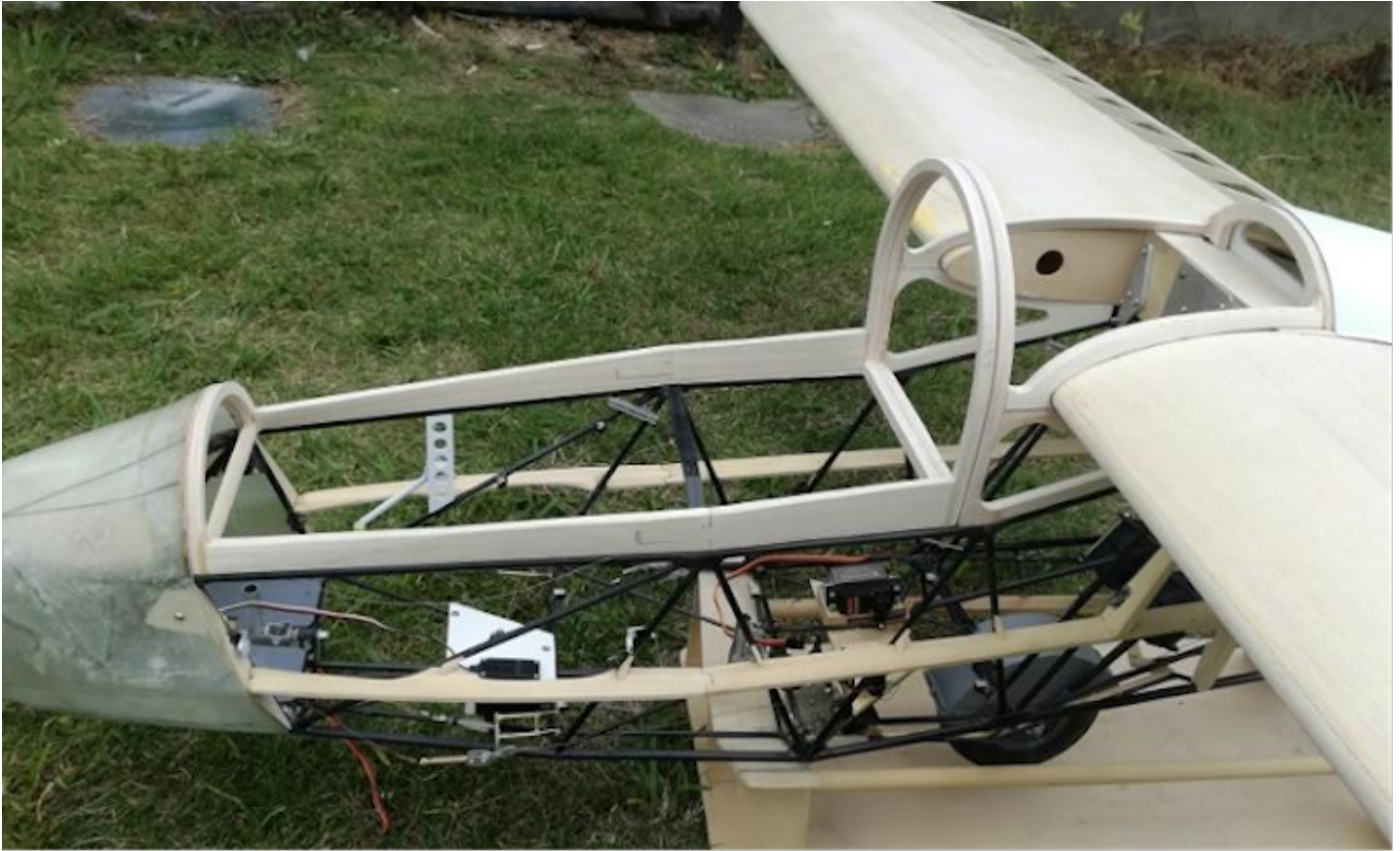
Photo 227: Putting the frame on the fuselage
