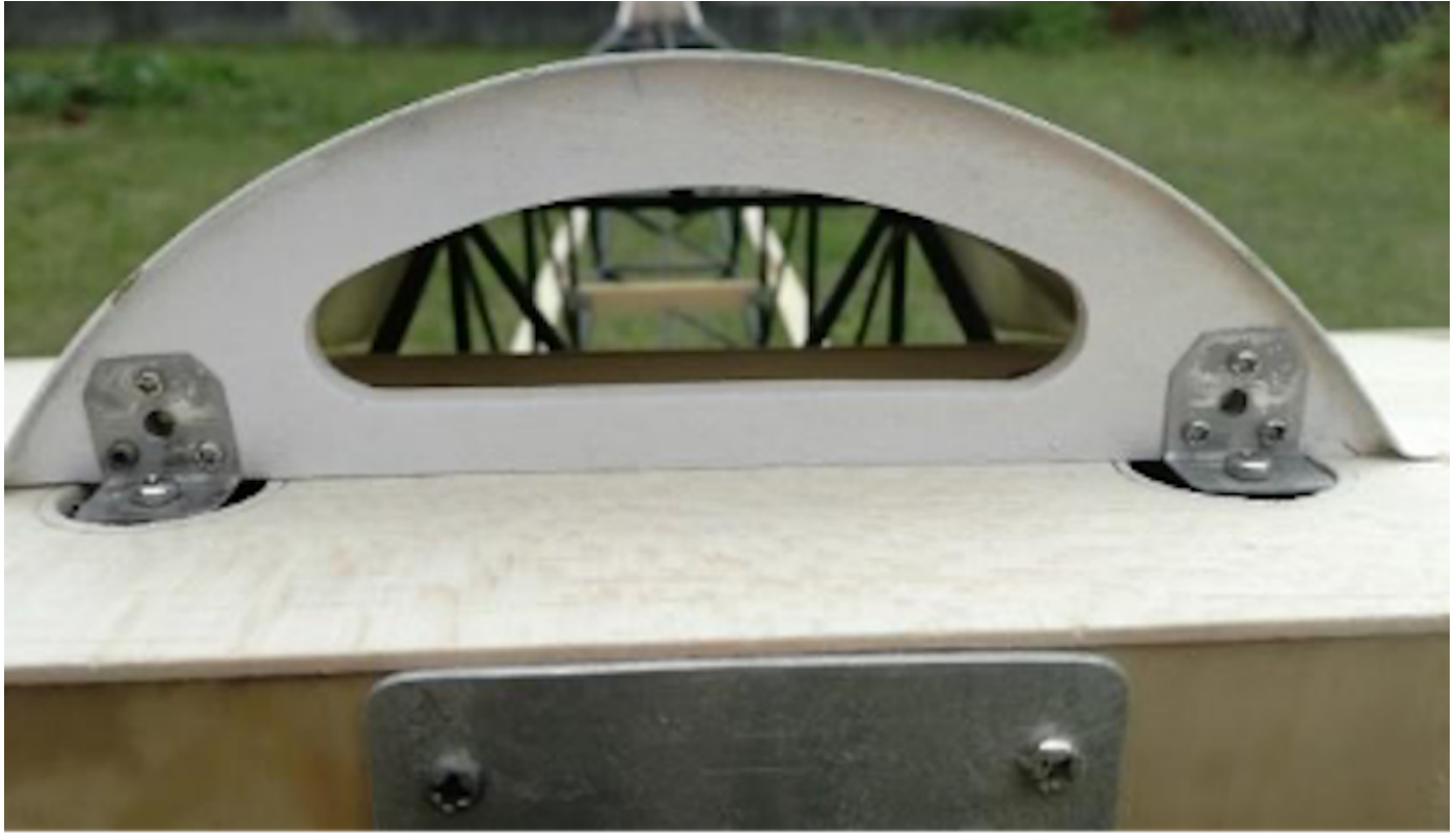
Photo 228: Positioning holes for rear canopy
