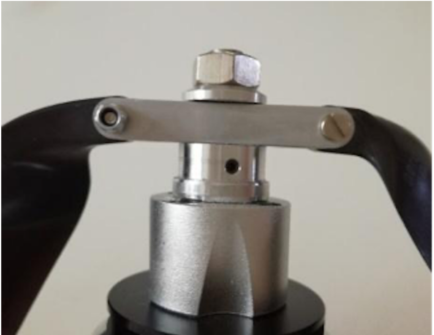
Photo 230: The installed shaft collar.
