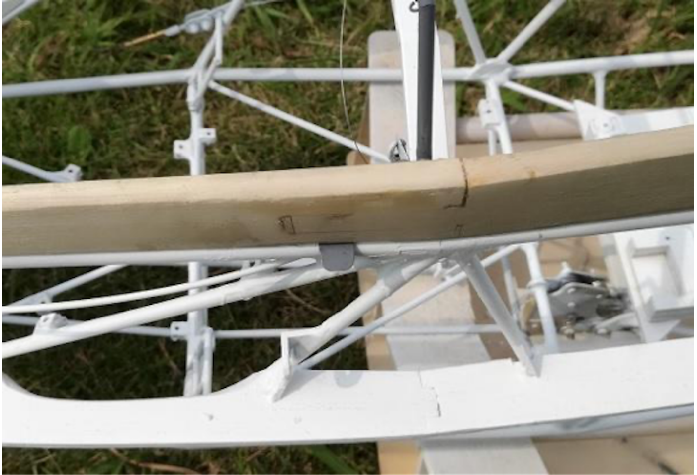
Photo 238: Lever for opening and closing the canopy
