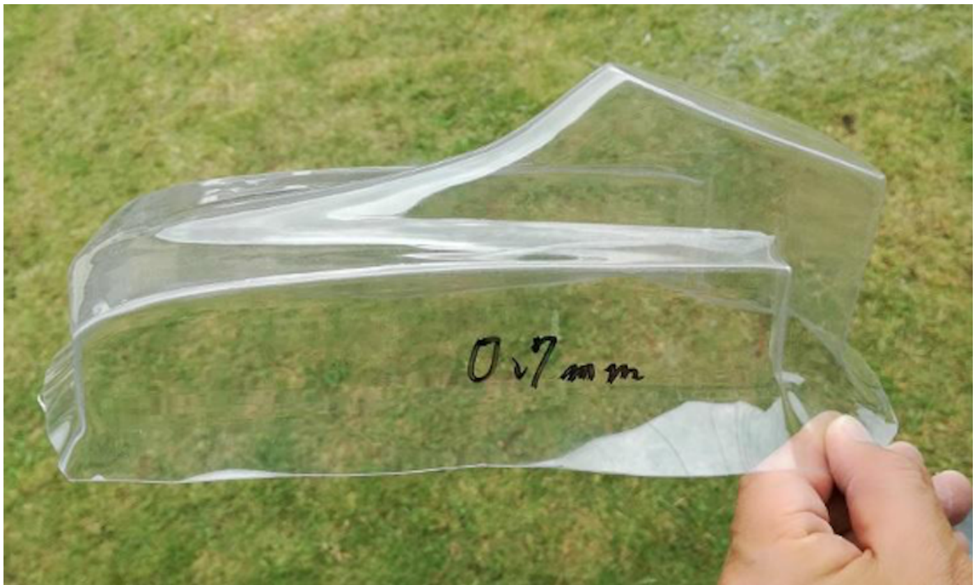
Photo 241: The tail wing fairing made by the vacuum process
