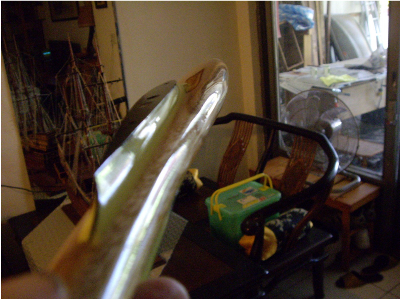
The wing stub Fairing sanded and pre-finished with a sealing coat of epoxy.
