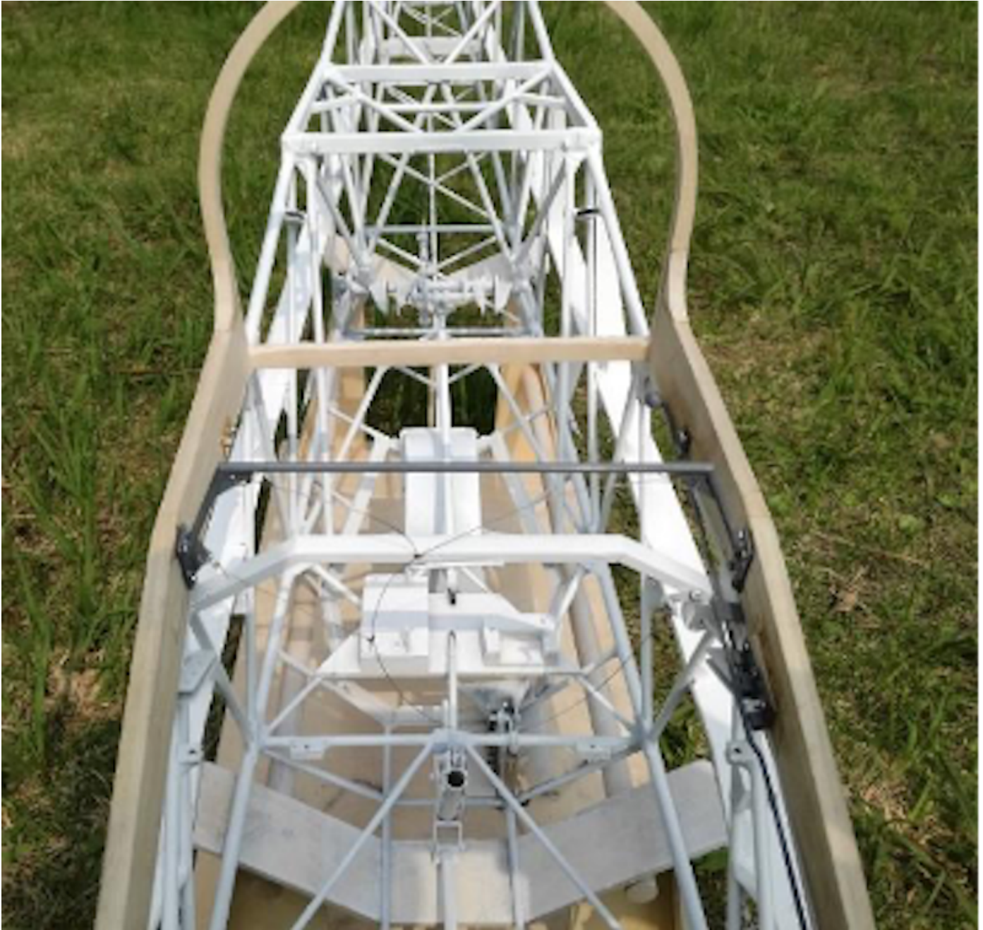
Photo 233: Canopy frame with accessories installed
