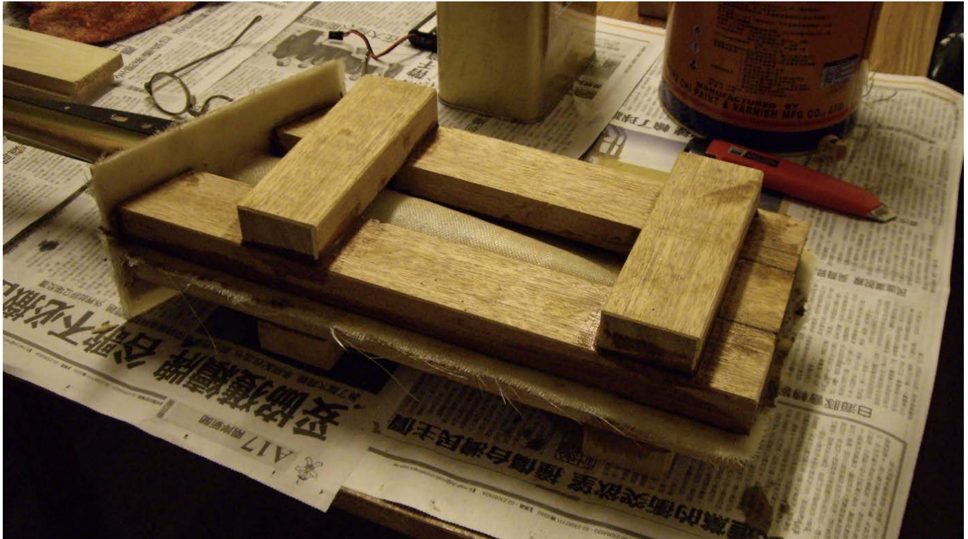
Nosecone mould, untrimmed — note the needle-sharp glass fibres.
