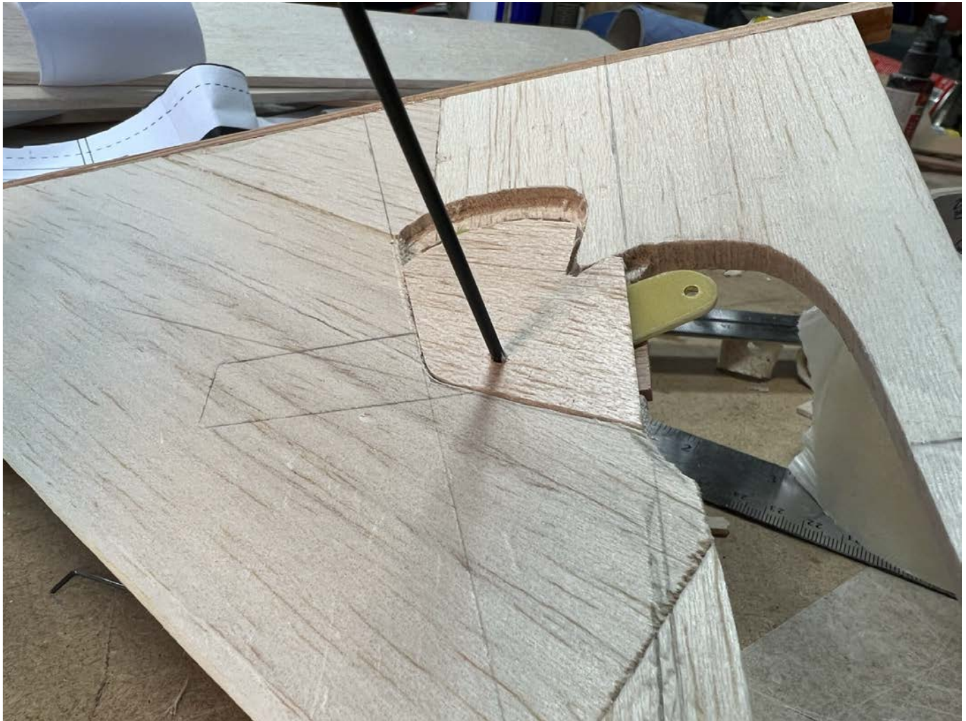
A rebate for the bell crank and a shim to cover it.
