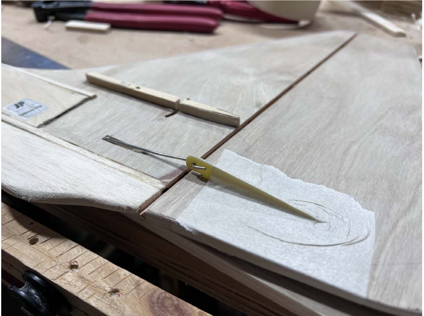
Rudder control horn cut and sanded to shape; recessed into the rudder.
