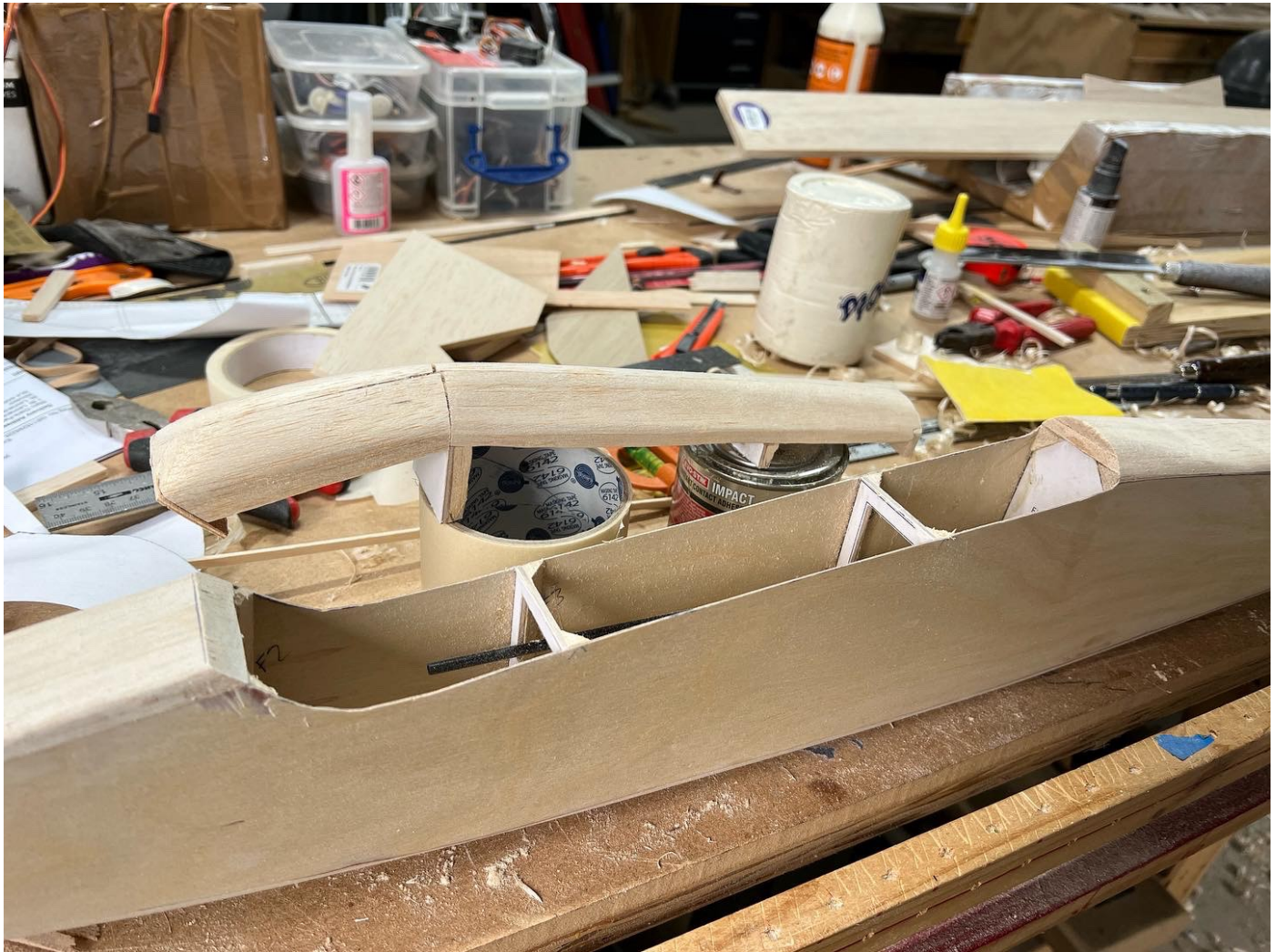
Blocked form balsa canopy top, sanded to shape, then liberated.
