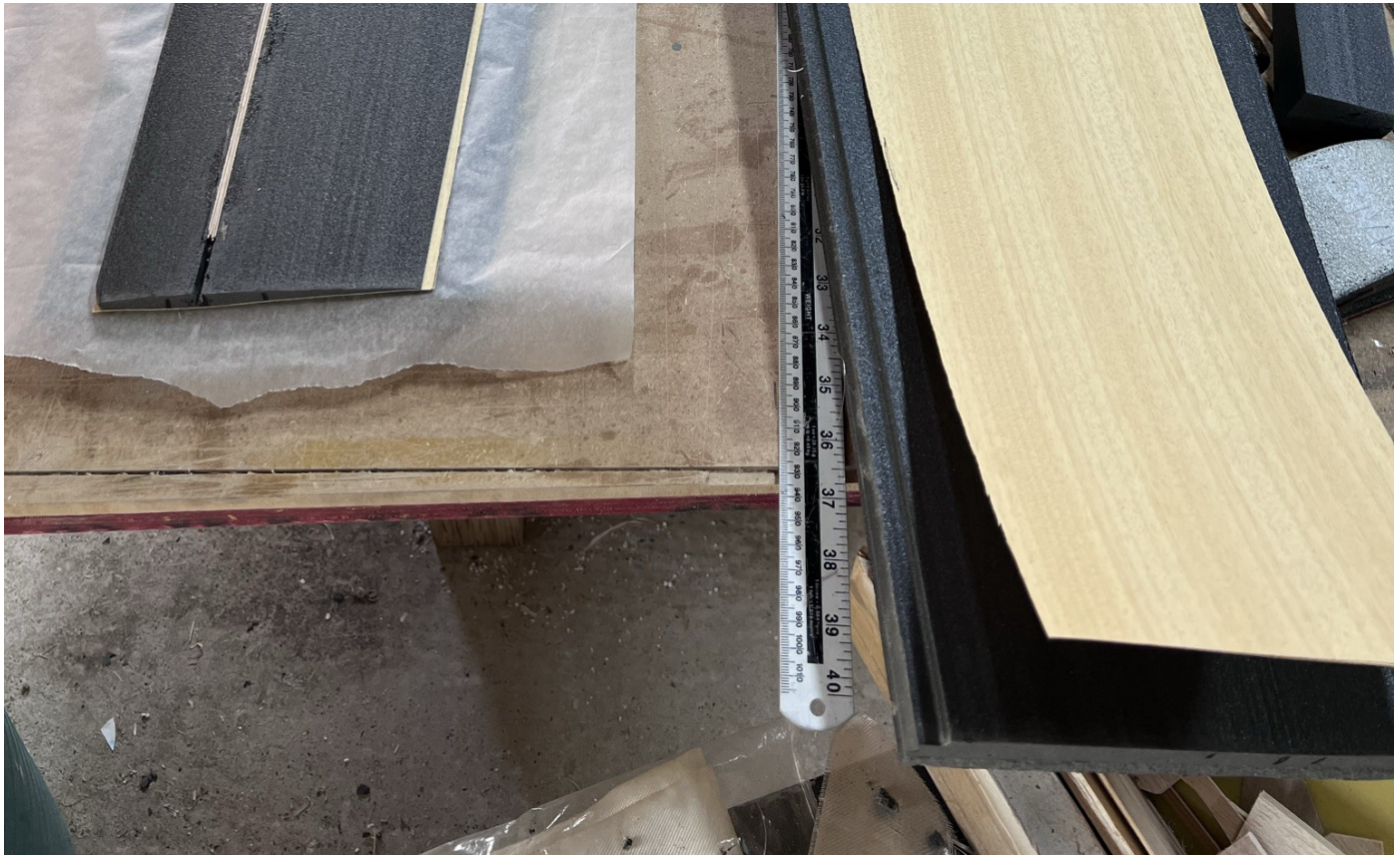
Dry mock-up, veneers and glass cut to size.
