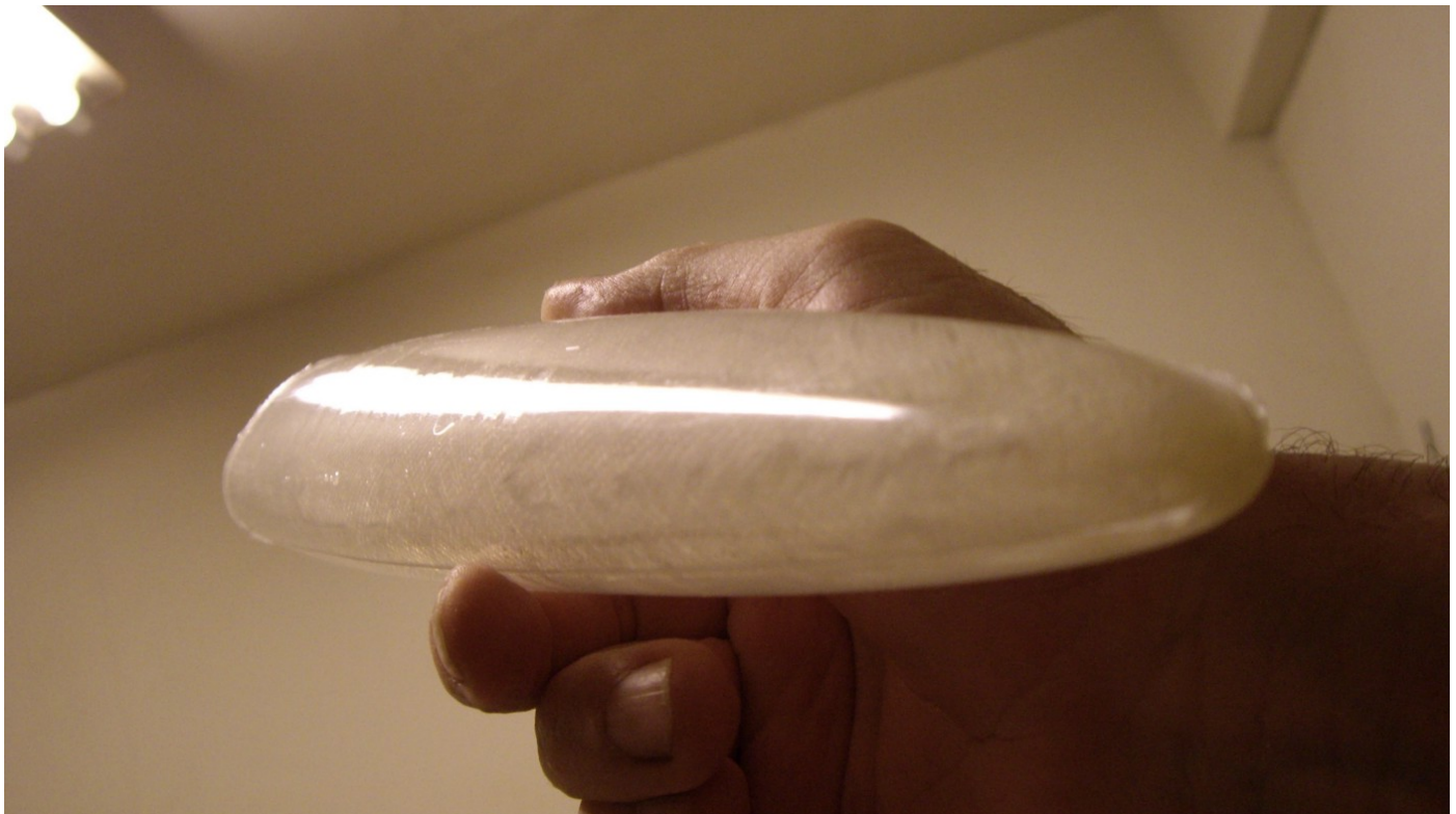
A Shinobi nose cone fresh out of the mould — note the crisp seams.
