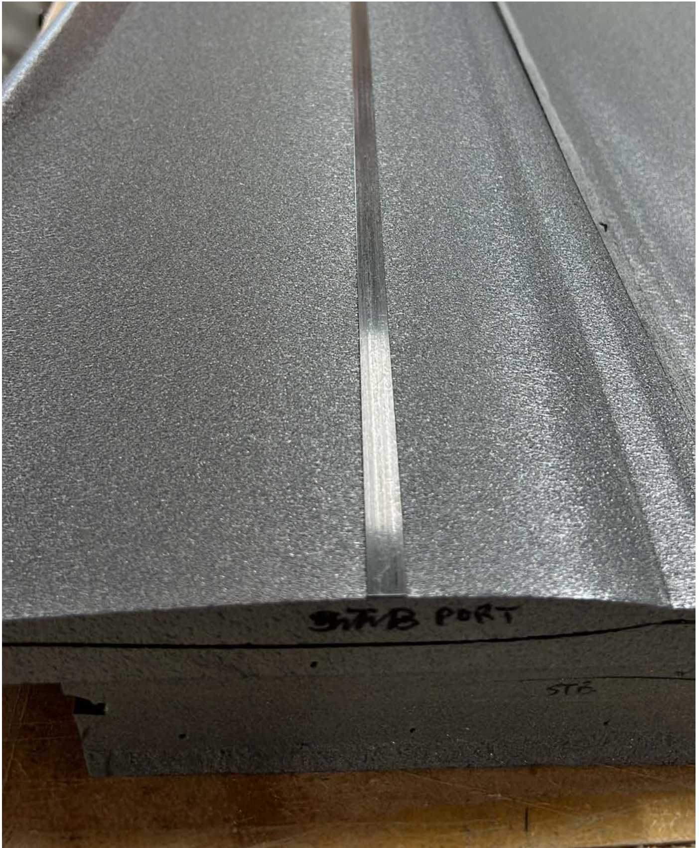
A test core hints at good things to come, testing locations for spars.
