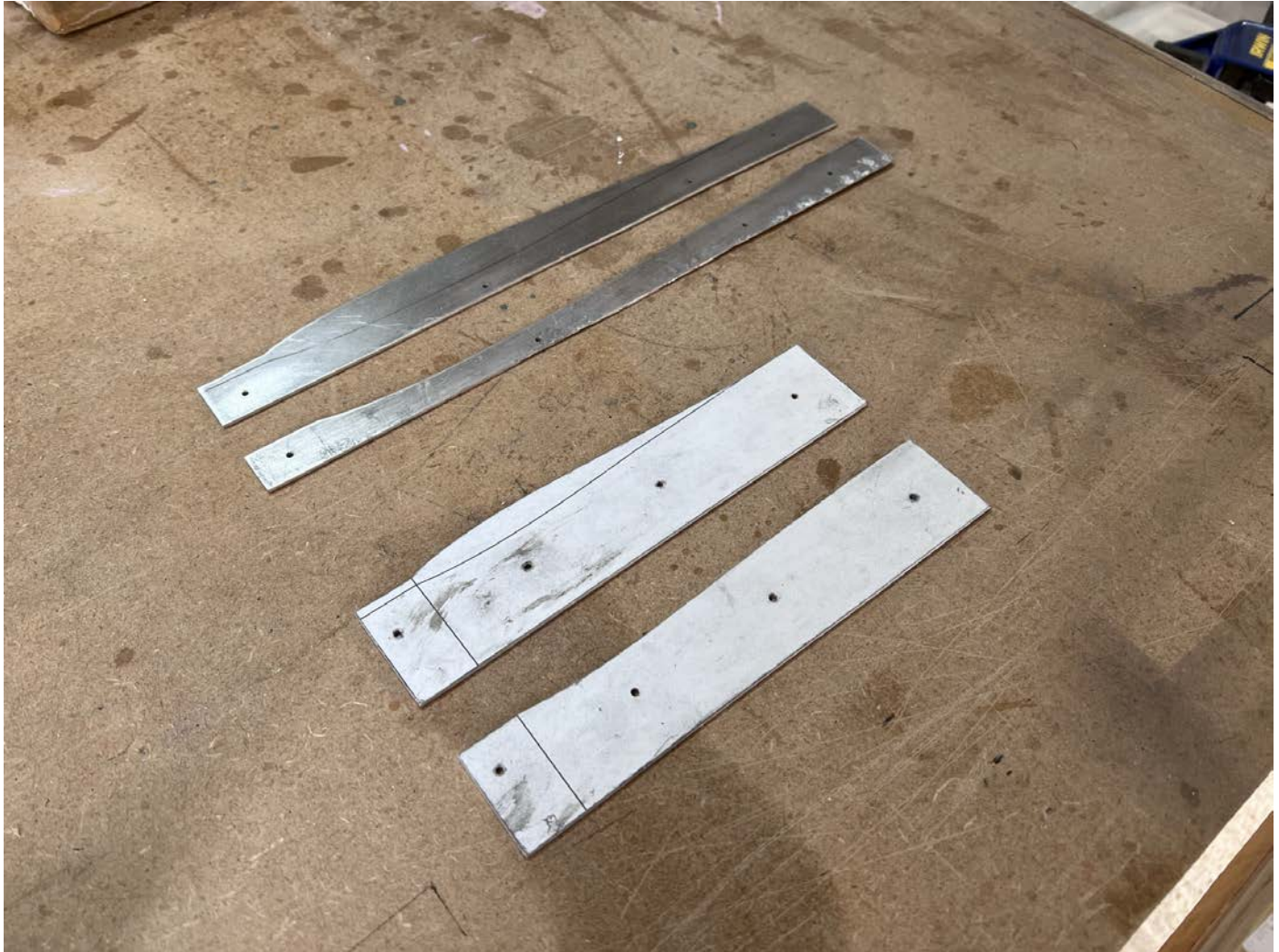
Templates for the hot wire made from aluminium sheet.
