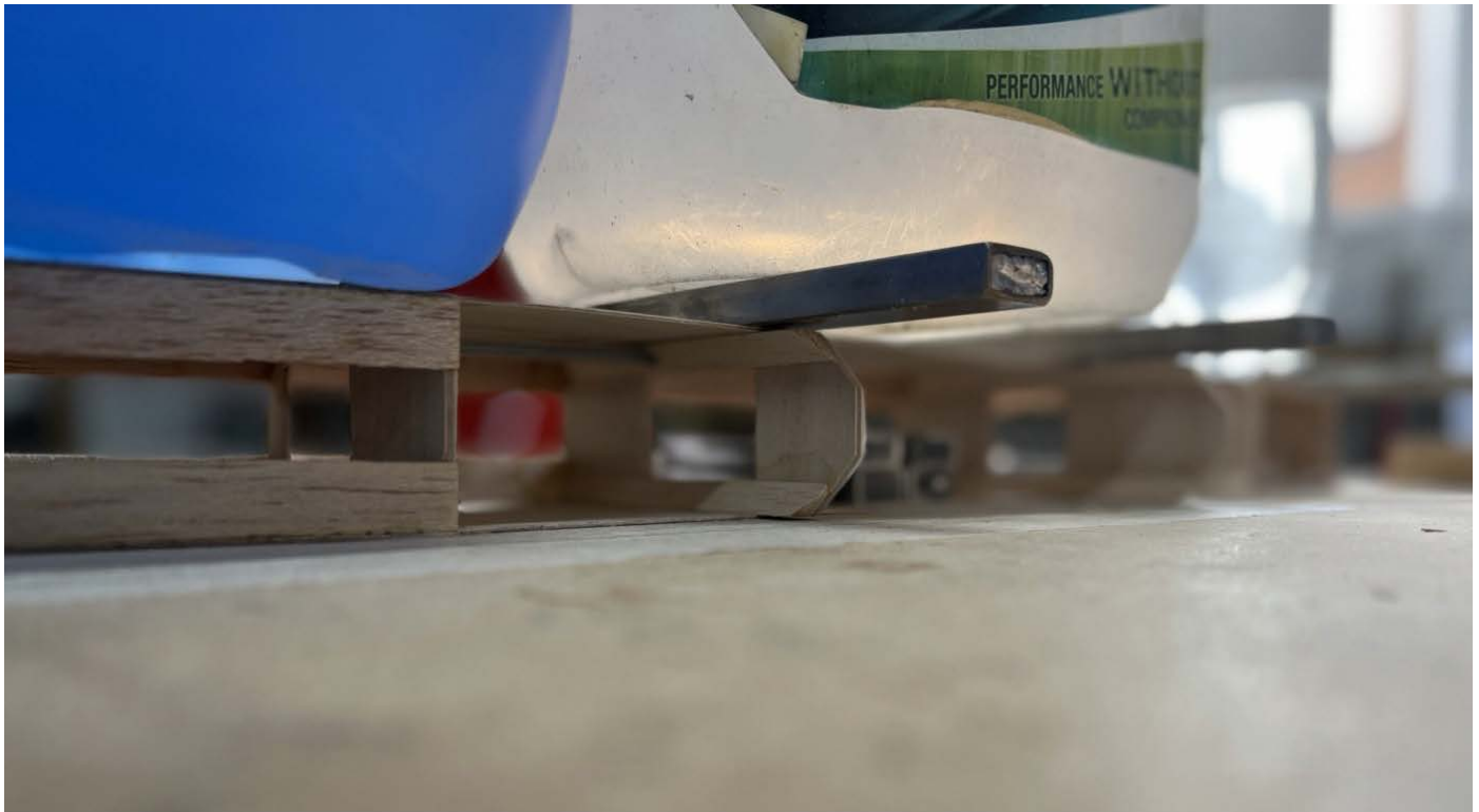
Two sides, glued together and weighted while the glue cures.
