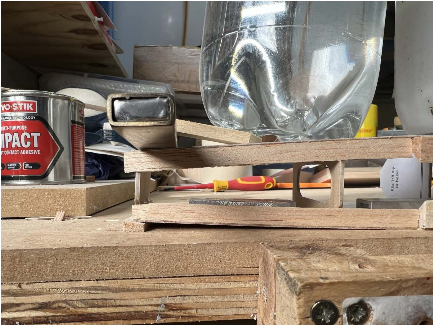
Weights and shims to taper the nose.
