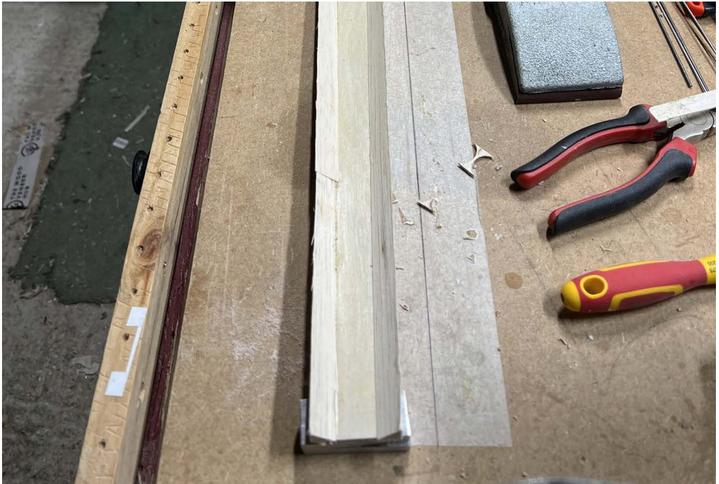
Gluing the formers, weighted to keep things flat and square
