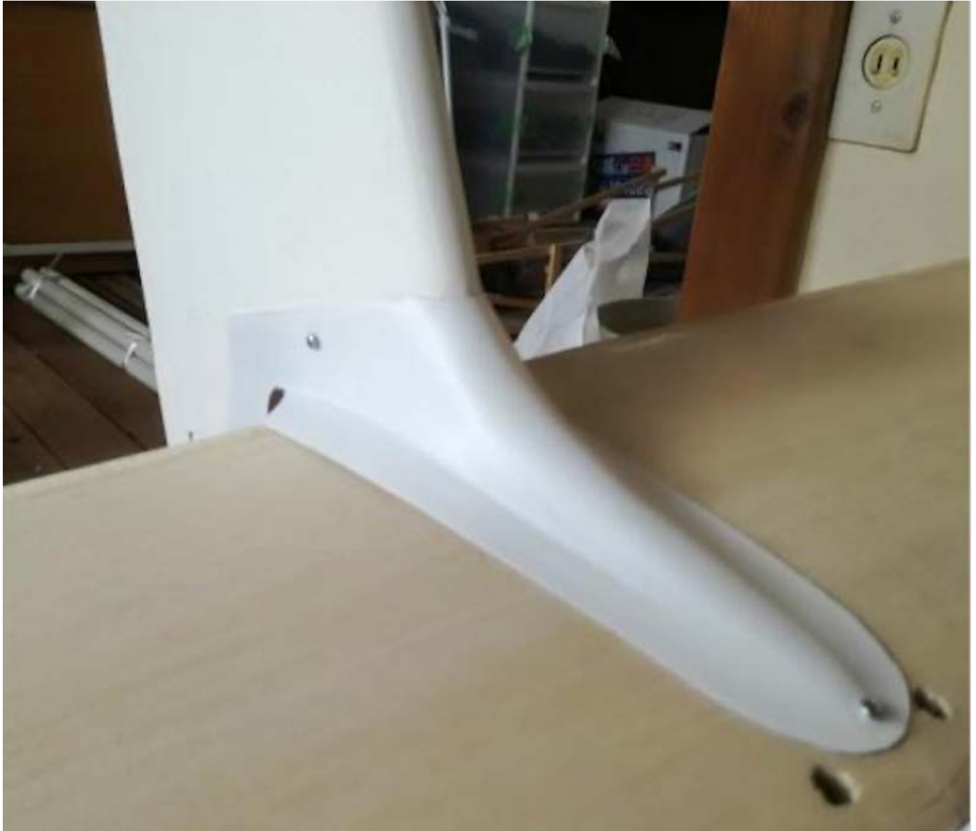
Photo 245: Installation of the tail wing fairing
