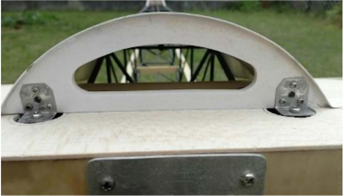
Photo 228: Positioning holes for rear canopy
