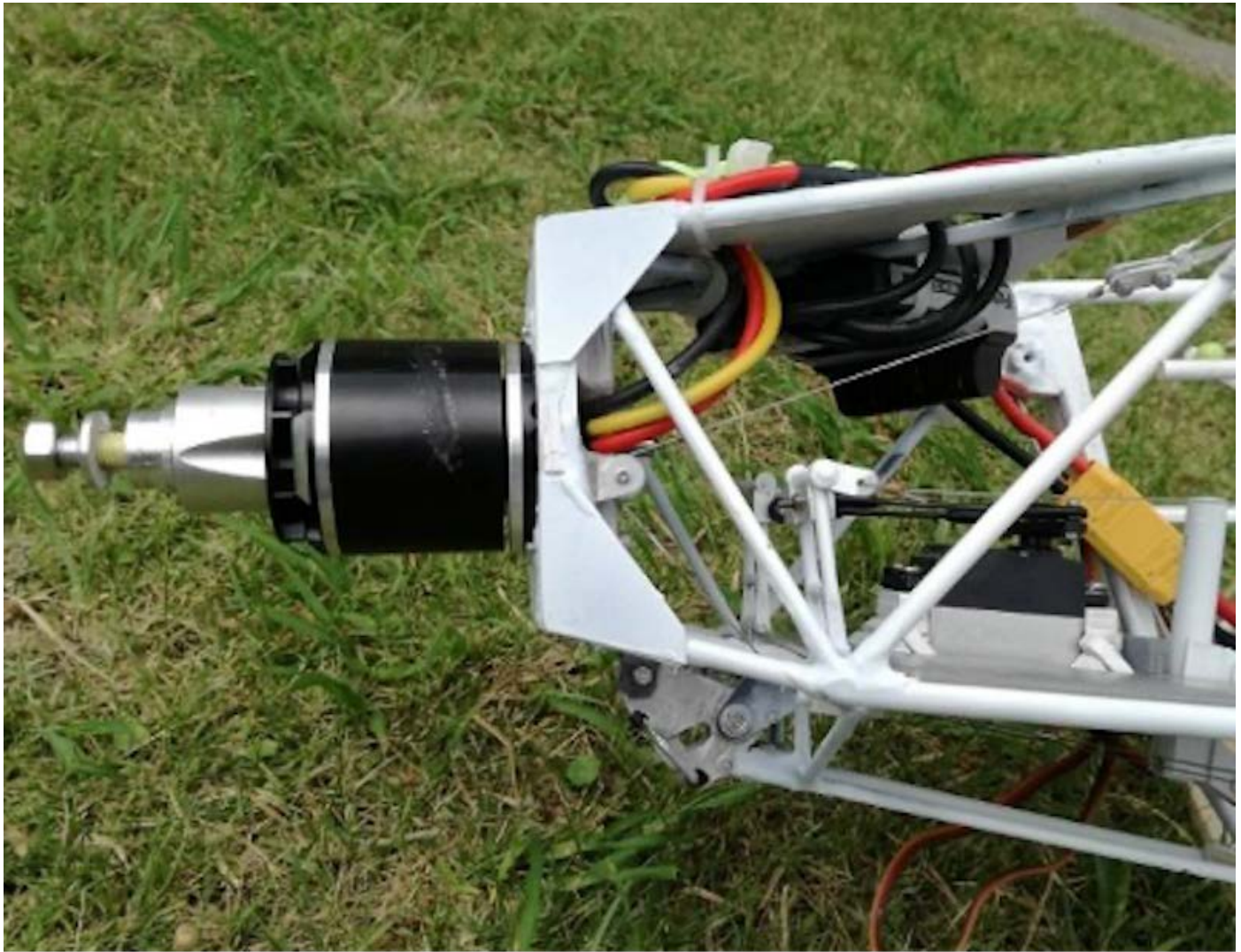
Photo 248: Mounting the power supply for the receiver and the amplifier: power supply (left), amplifier (right)
