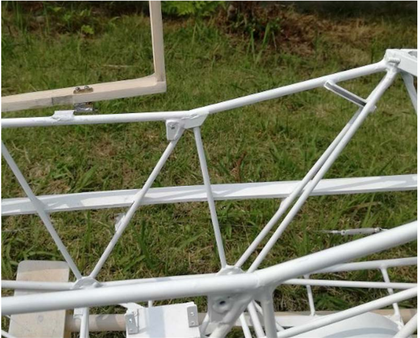
Photo 240: Rear canopy mounting mechanism
