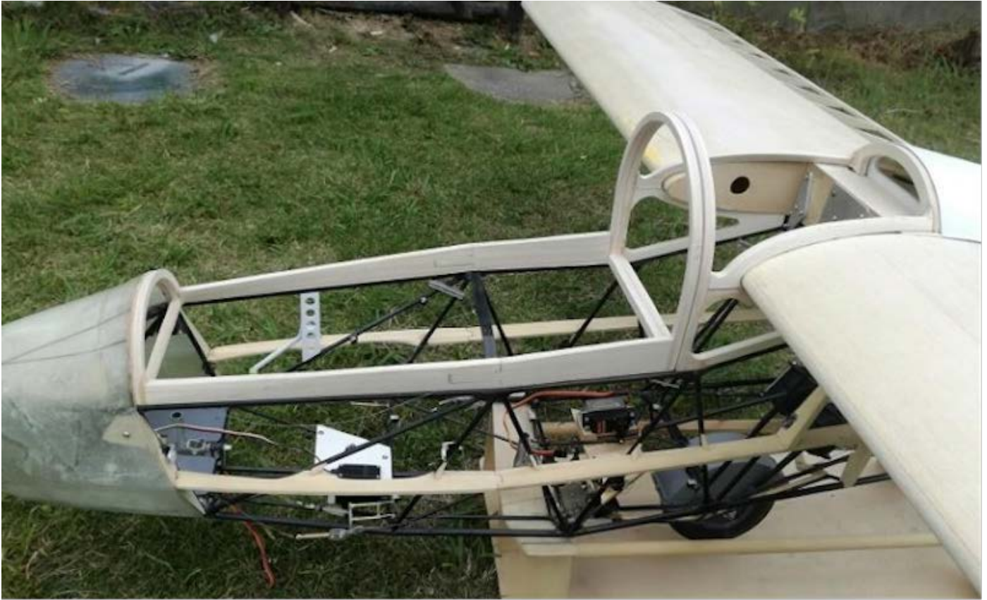
Photo 227: Putting the frame on the fuselage
