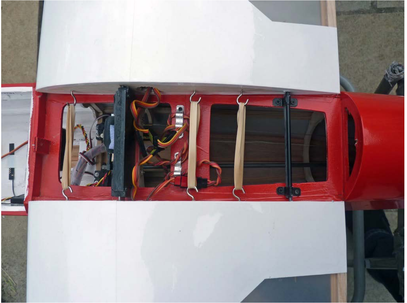
06: The wings are retained with old-fashioned No 63 rubber bands.
