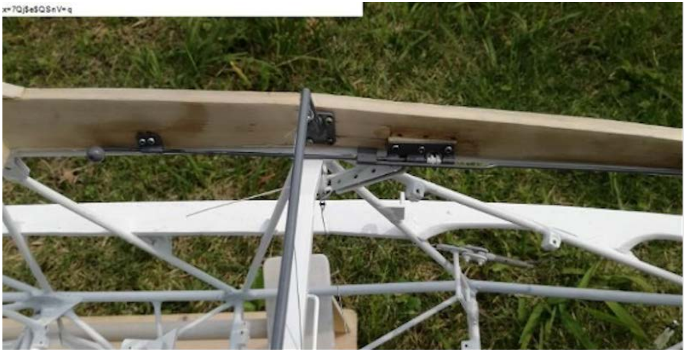
Photo 235: Canopy locking mechanism
