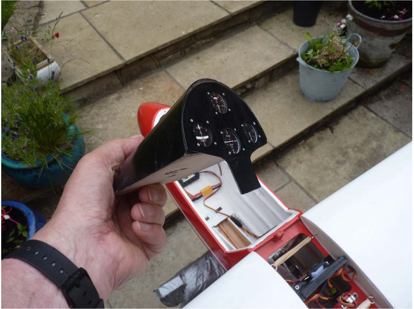
07: The instrument console is retained with magnets, as is the canopy.
