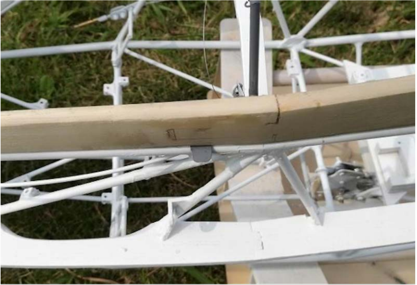
Photo 238: Lever for opening and closing the canopy
