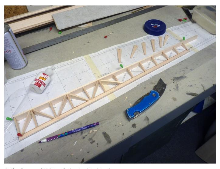
11: The ailerons are built flat on the board and top-hinged.
