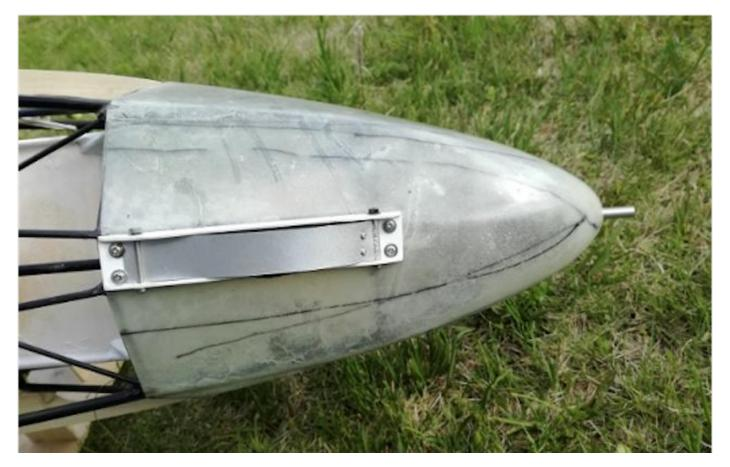
Photo 204: Installation of the nose skid
