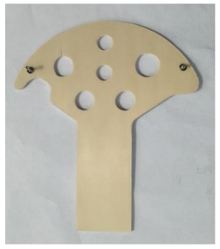
Drawing 53 (left): The instruments panel | Photo 216 (right): The panel made of 1.6 mm plywood
