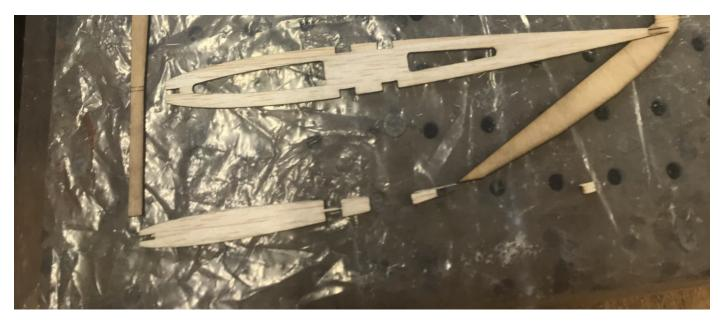
The vertical stab is built as one piece, then the rudder is cut off and the gap is filled in with beveled balsa.
