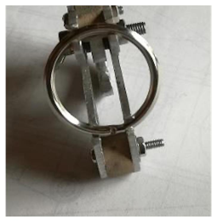
Photo 211: Cable release mechanism for aerotowing; side (left) and bottom (right) views
