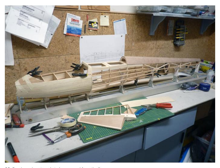
**02**: Fuselage almost ready to be removed from the jig.
