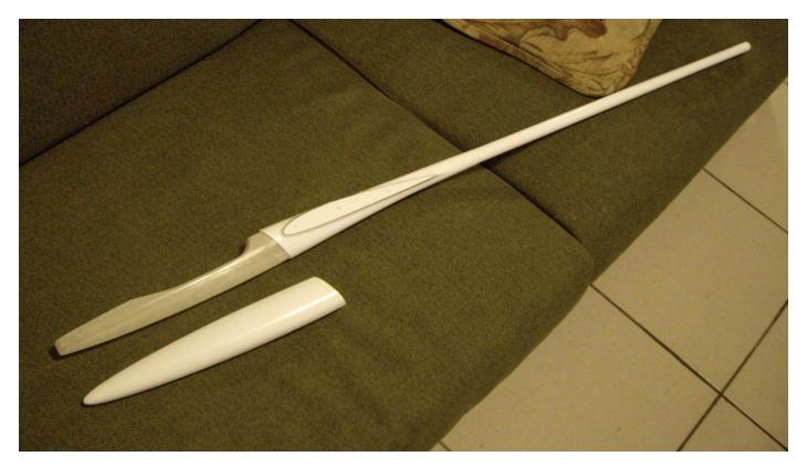
Shinobi: a composite 4-part fuselage assembly for a small model of 50 to 70" span made from a home-made plug/mould set.
