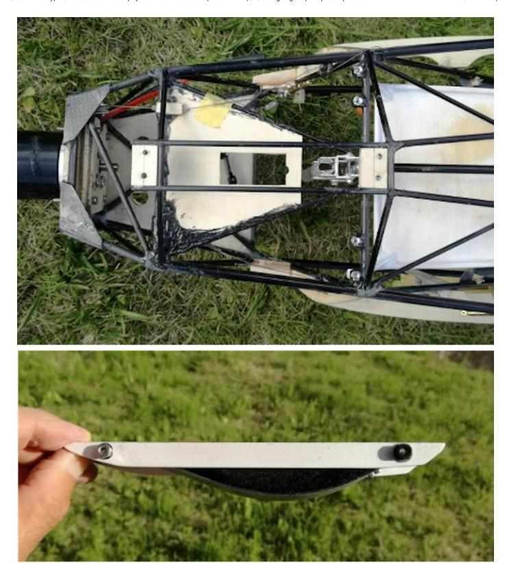
Photo 201: Nose skid attachment structure (left) and skid body (right)
