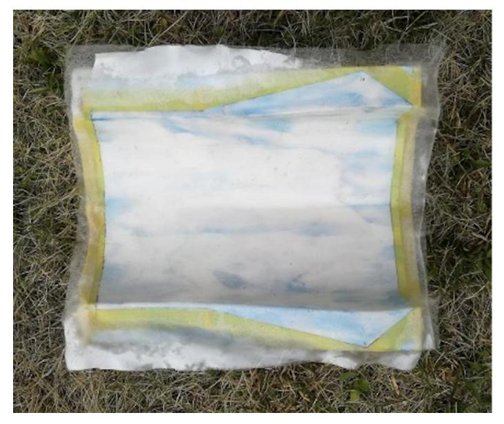
Photo 191: Finished applying the glass cloth
