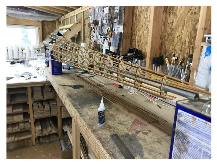
Formers jigged up and stringers partially installed.
