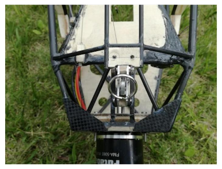
Photo 212: Installation of the Cable Release Mechanism for Aerotowing
