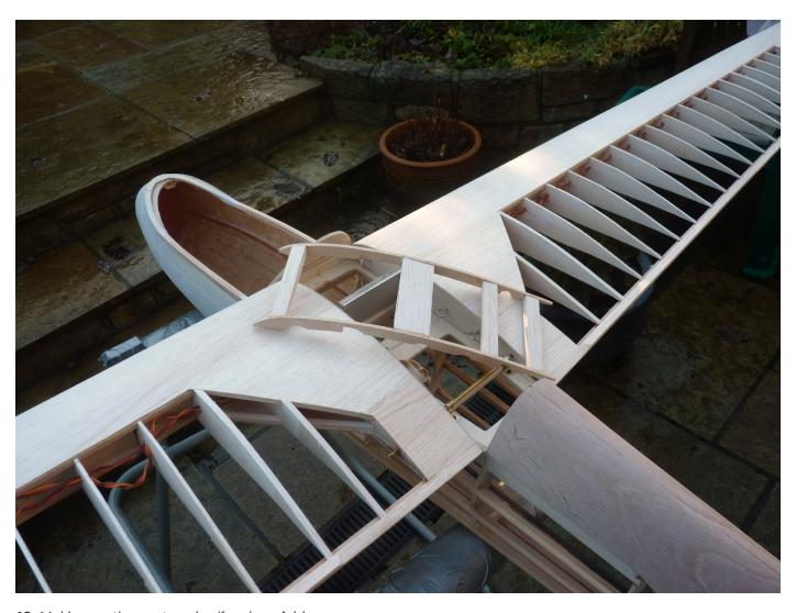
12: Making up the centre wing/fuselage fairing.
