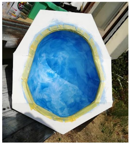
Photo 195: Plaster mold coated with PVA
