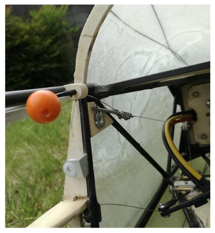
Photo 215: Towing cable release knob and spring
