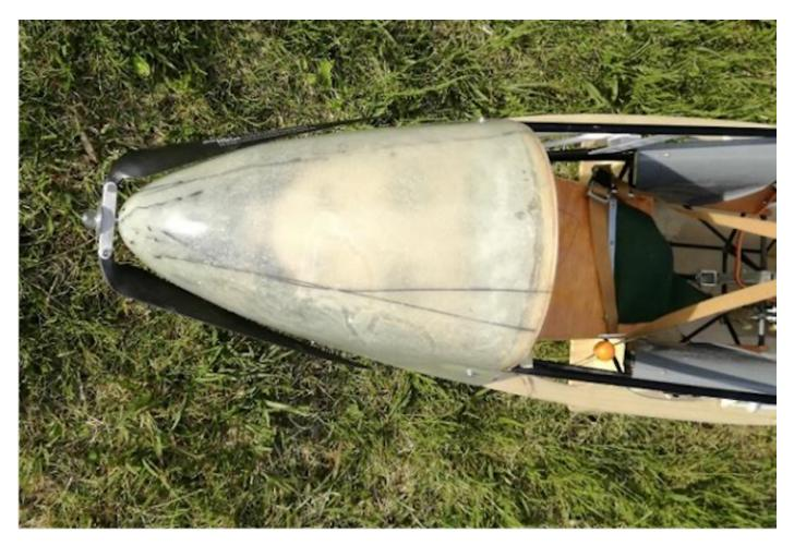
Photo 206: Trial installation of the folding propeller
