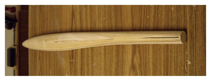
The fuselage shape is rough (**very!**) carved. Note the wing cutout inserted and shaped along with the rest of the curves. You can just see the remains of marks made with a sharpie to remind me that I'm close to the final shape in those areas.
