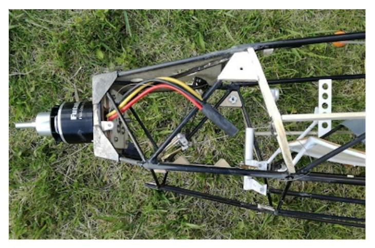
Photo 200: Cowling mounting structure
