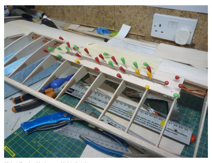
14: Installing the airbrake assembly into the wing.
