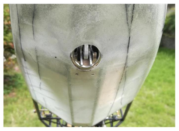
Photo 214: Cable release mechanism for aerotowing
