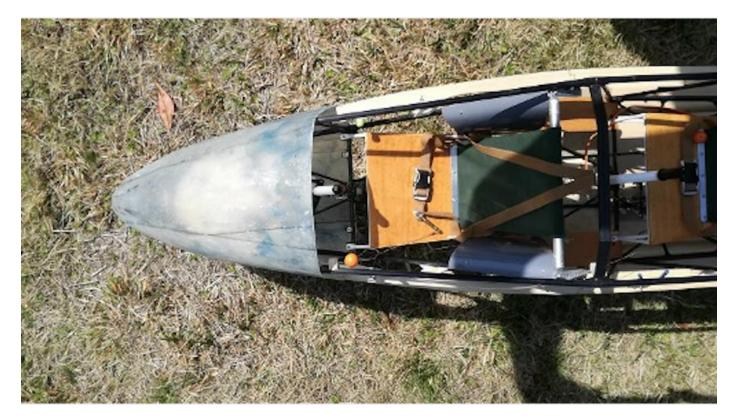
Photo 199: Fit check of the nose cowling
