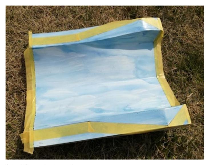
Photo 189: Preparing the plaster mold
