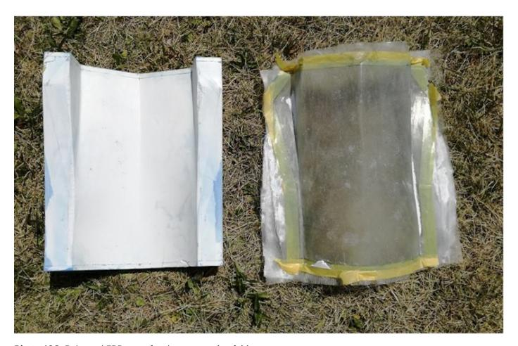
Photo 192: Released FRP parts for the center wing fairing
