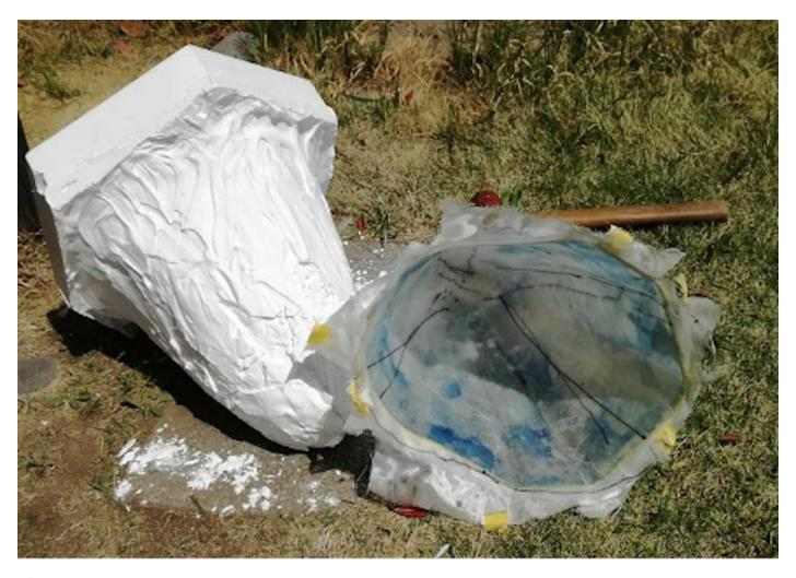
Photo 197: The FRP molded nose cowling finally removed from the plaster mold
