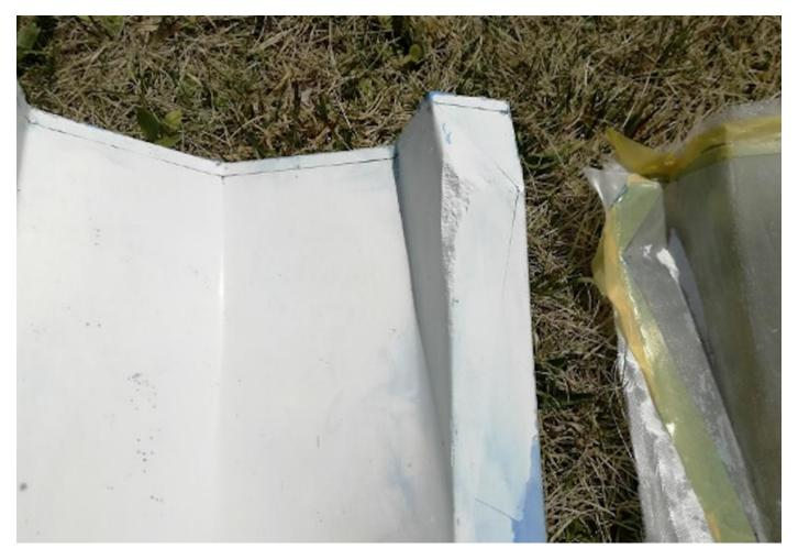
Photo 193: Chipped plaster mold
