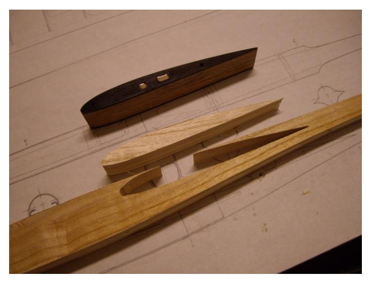
The wing profile that has been removed from the fuselage will now be tack glued back in to provide support when carving the final shape.
