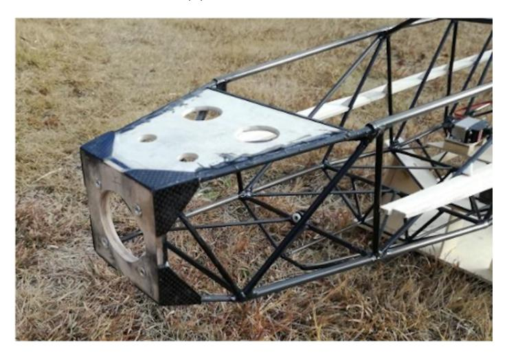
Photo 217: Top plate of the nose structure
