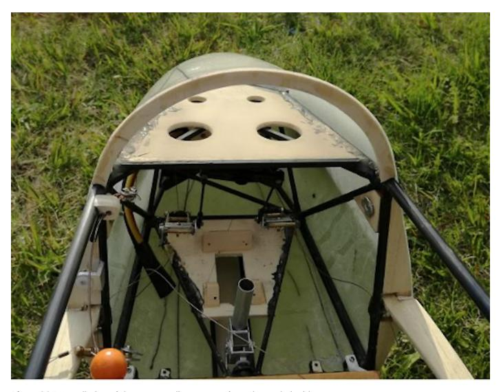
Photo 205: Installation of the nose cowling as seen from the cockpit side
