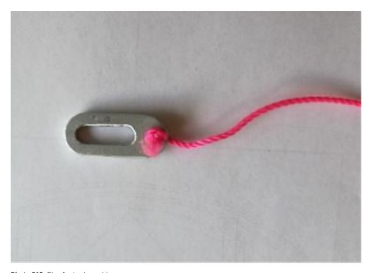
Photo 219: Ring for towing cable
