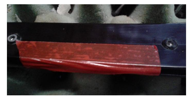
Put your bolts in the wing (or dowels or whatever) so you can get the alignment right before pressing the wing all the way down.
