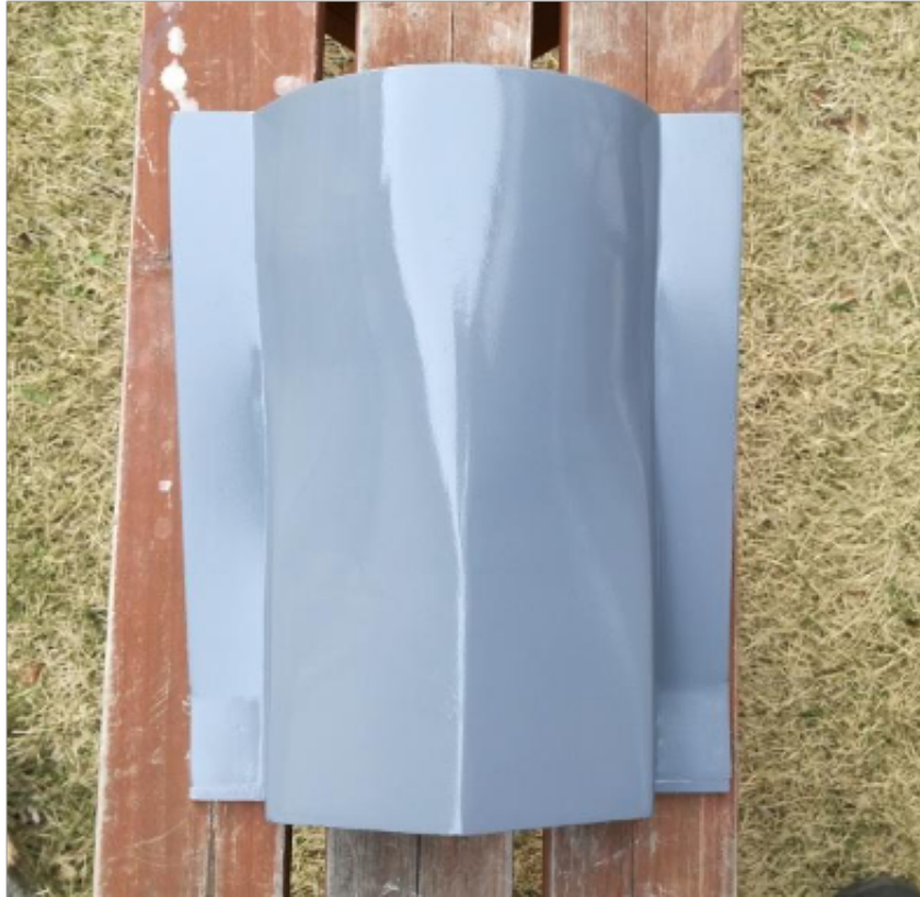
Photo 167: The completed wooden mold for the center wing fairing.
