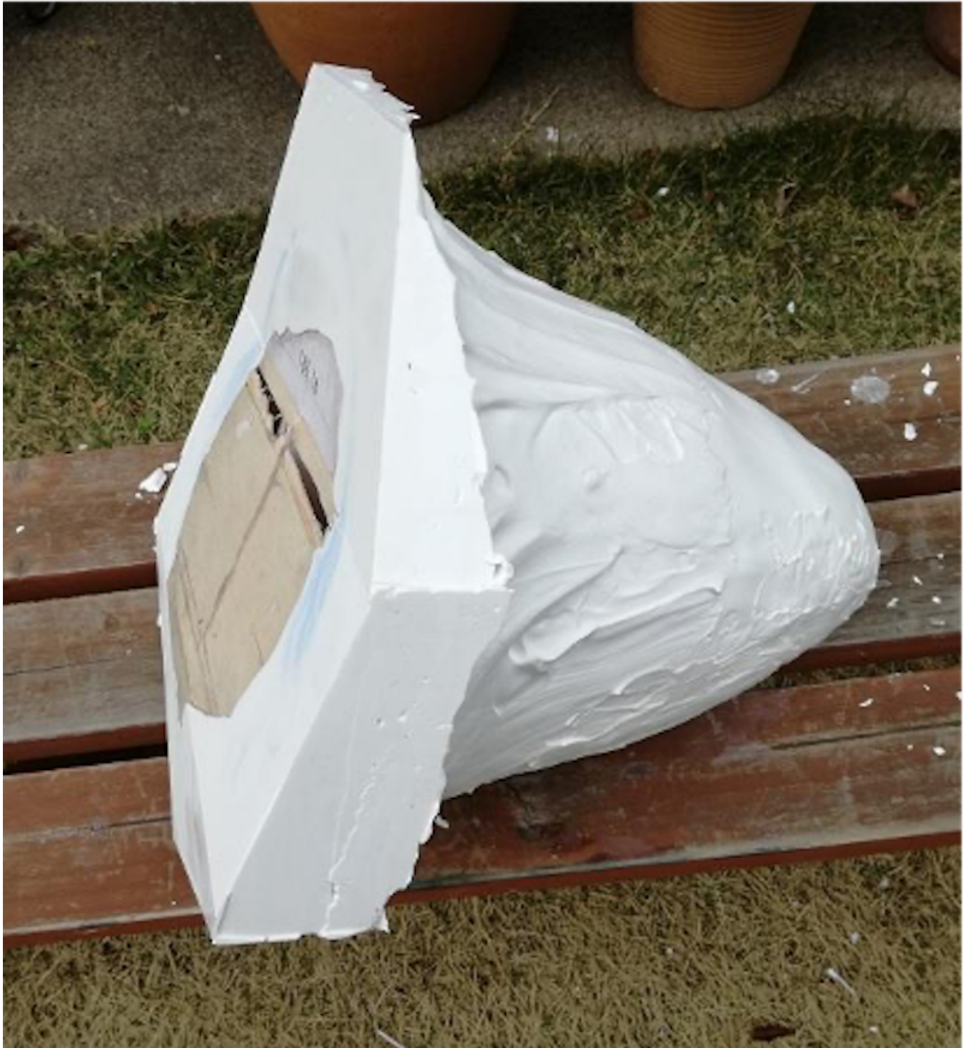
Photo 178: Plaster mold with the wooden frame removed.
