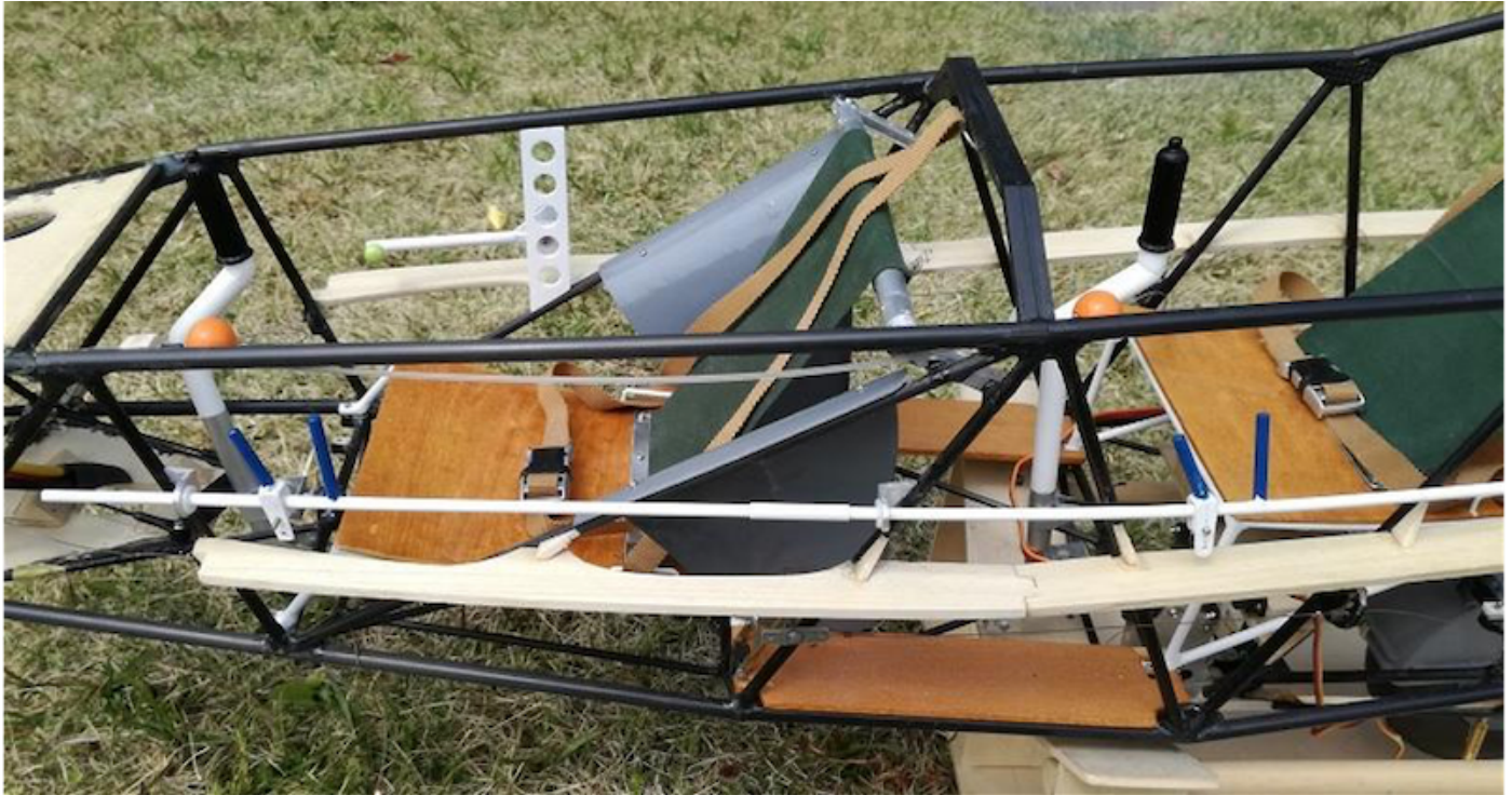
Photo 188: Spoiler operating mechanism.
