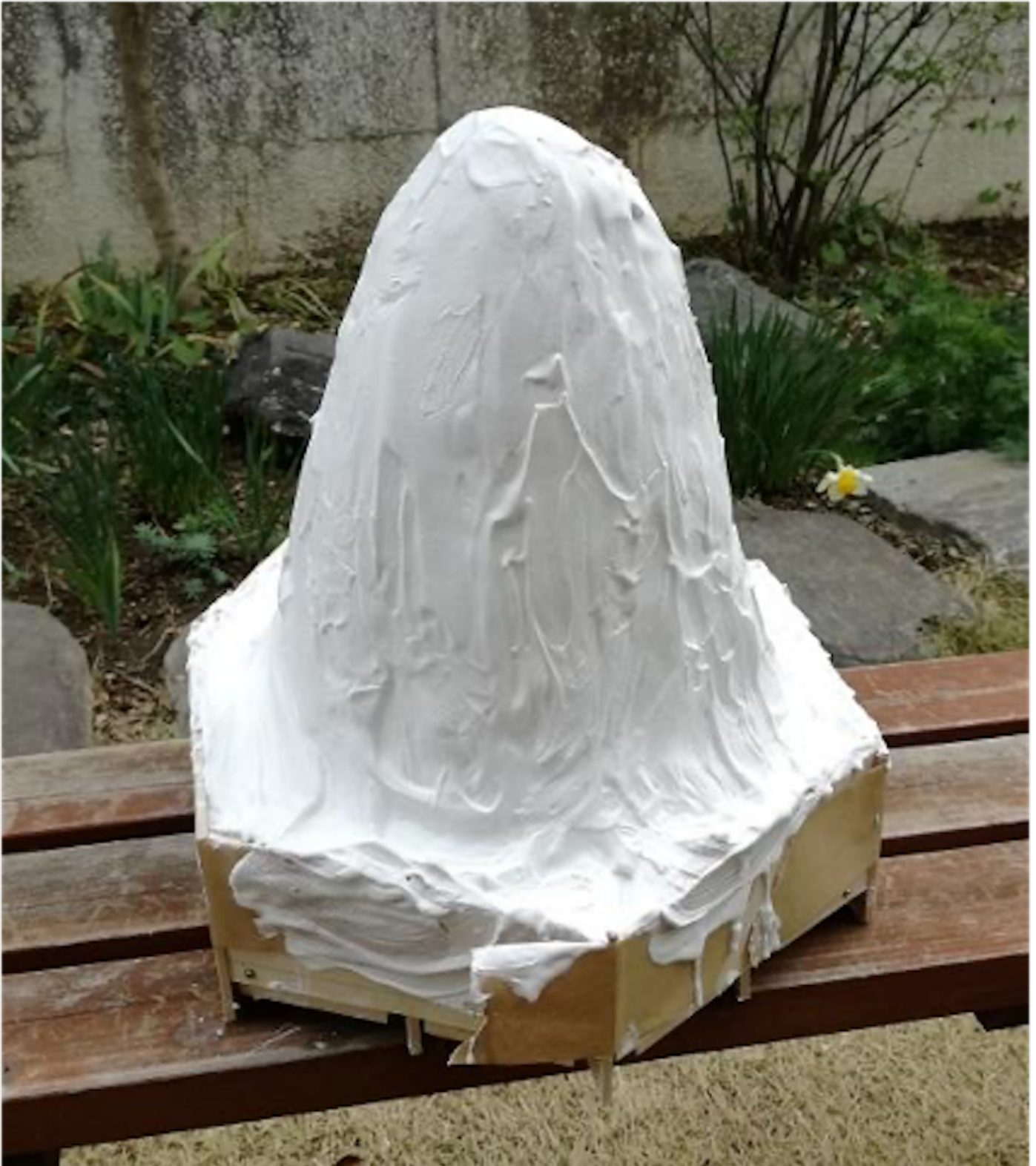
Photo 177: Wooden mold after plastering.
