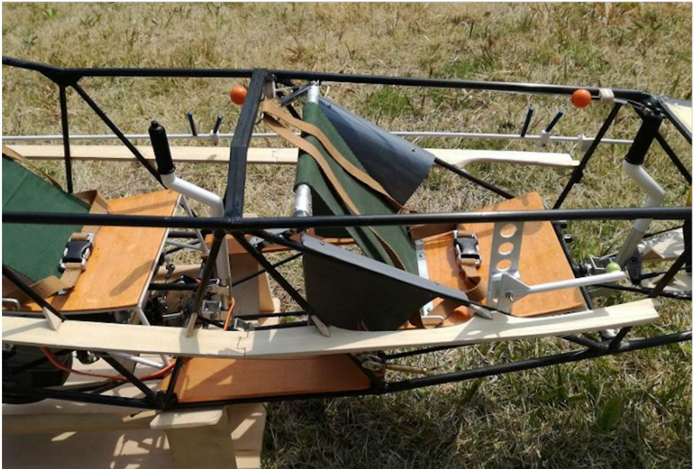
Photo 184: Control sticks and related structure.
