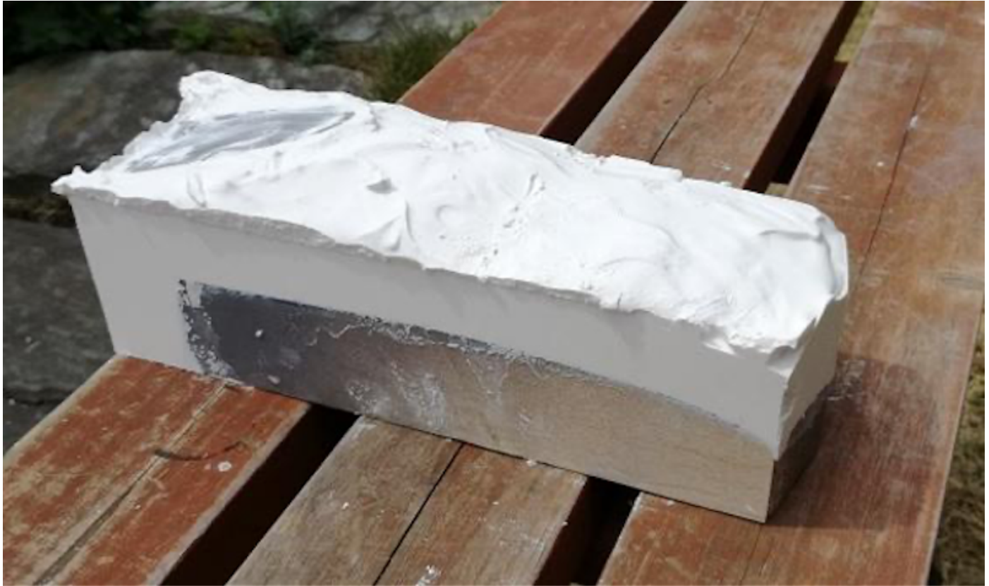
Photo 182: Plaster mold with the wooden frame removed.
