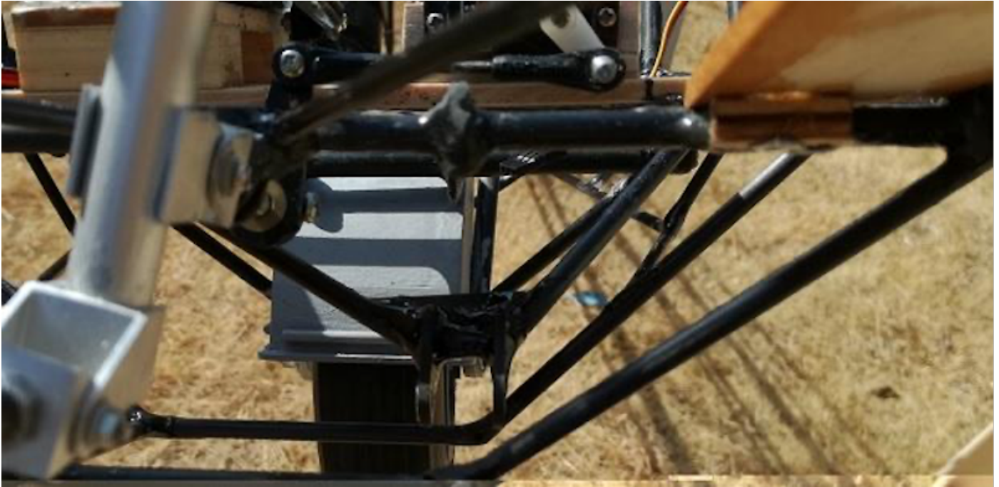
Photo 151: Assembly of the release mechanism mounting structure.
