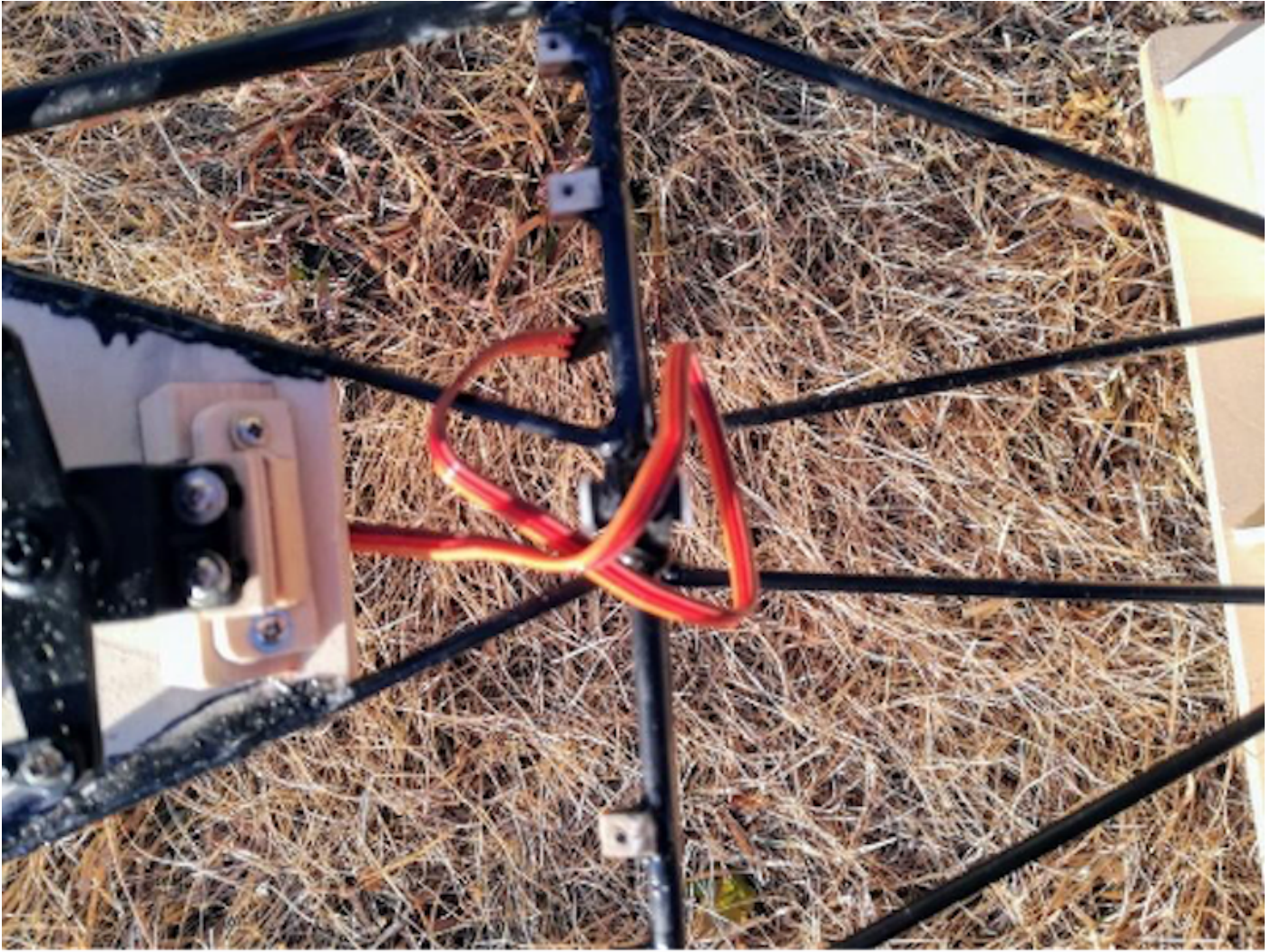
Photo 138: The 'lug holders' attached to the fuselage structure.
