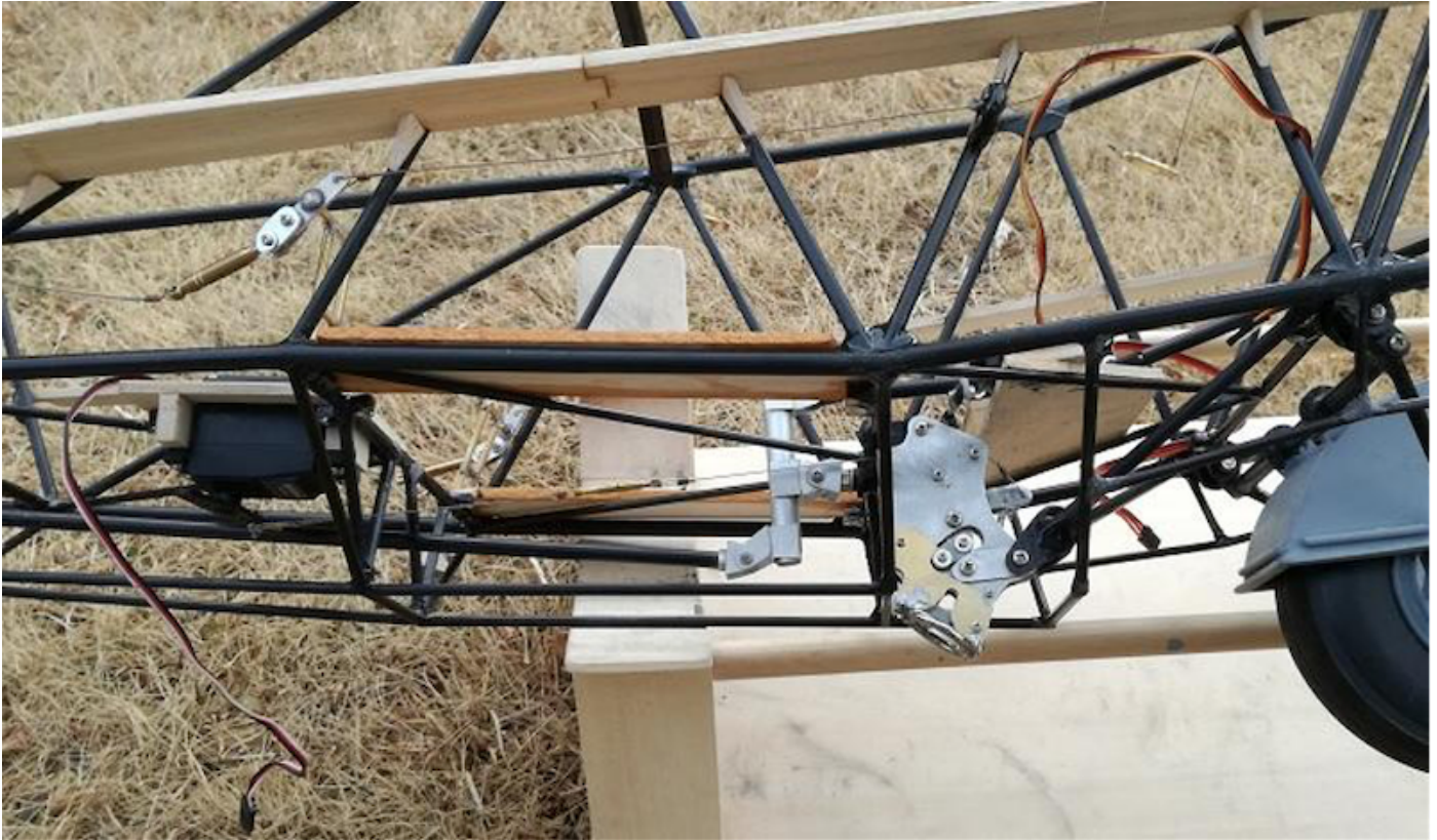
Photo 154: Release mechanism and its open/close servo.
