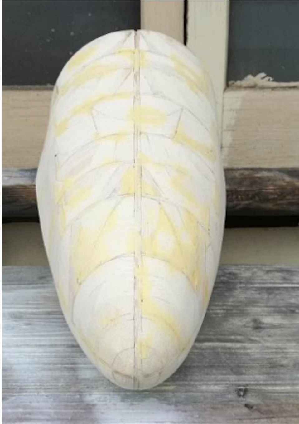
Photo 159: Pasting and shaping of the outer surface.
