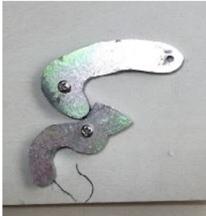
Photo 145: Prototype of the release mechanism: closed (left) and open (right).
