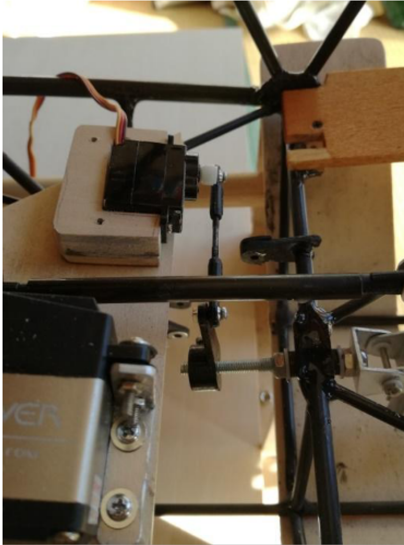
Photo 144: Dummy aileron servo installed.
