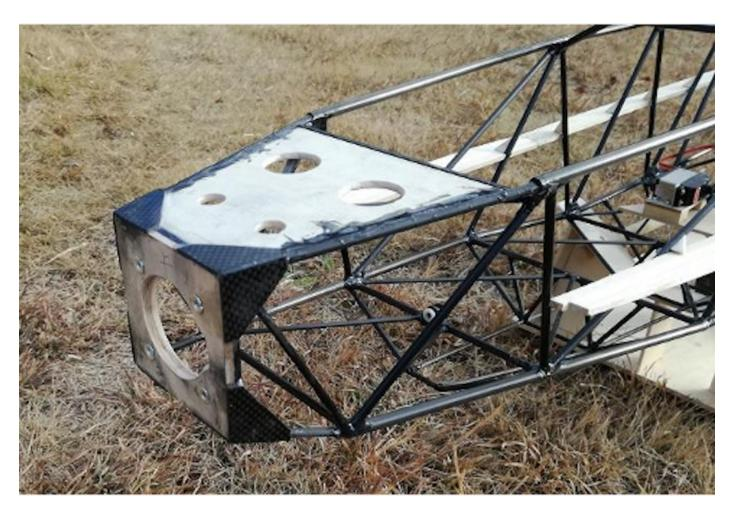
Photo 125: The completed motor mount.
