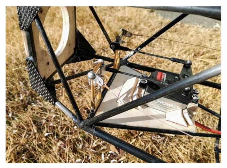
Photo 132: Installation of the rudder servo.
