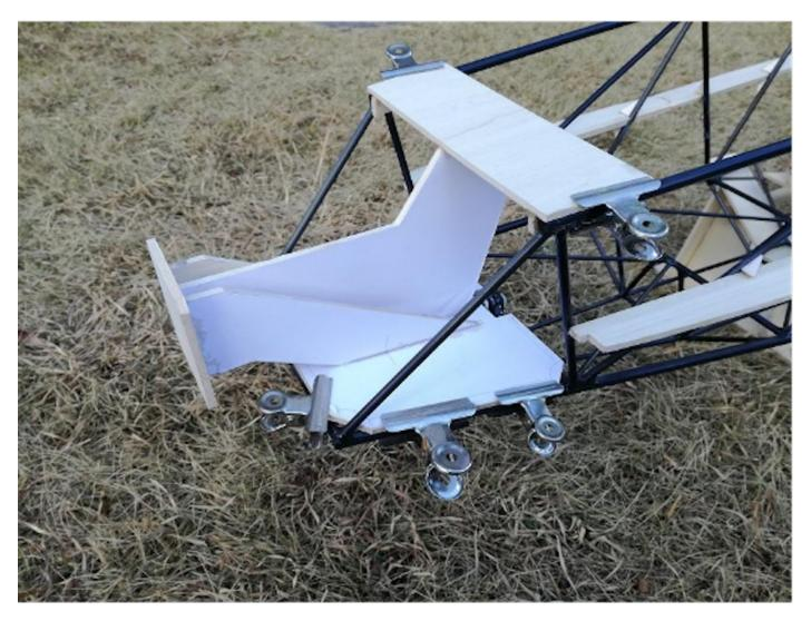
Photo 122: Motor mount assembly jig.
