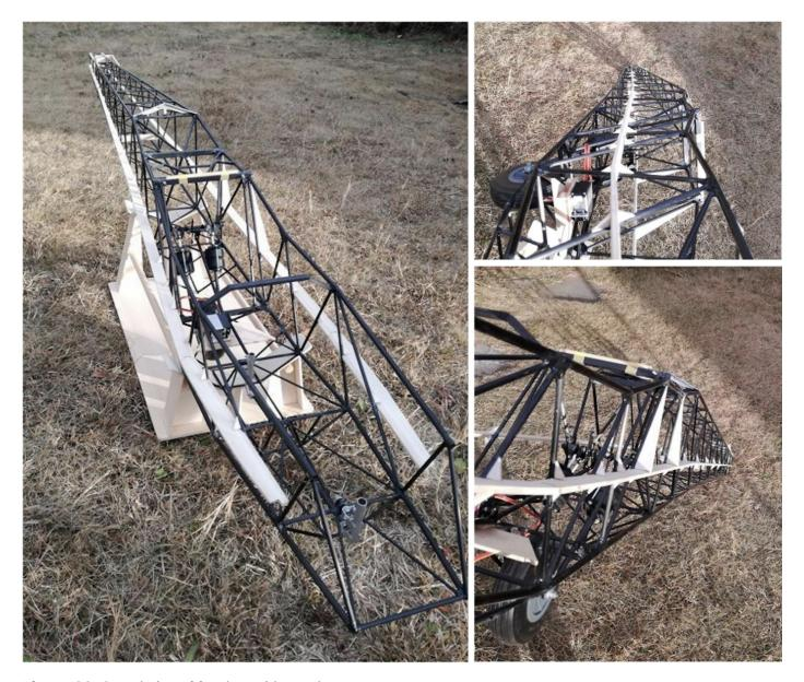
Photo 120: Completion of fuselage side overhangs.
