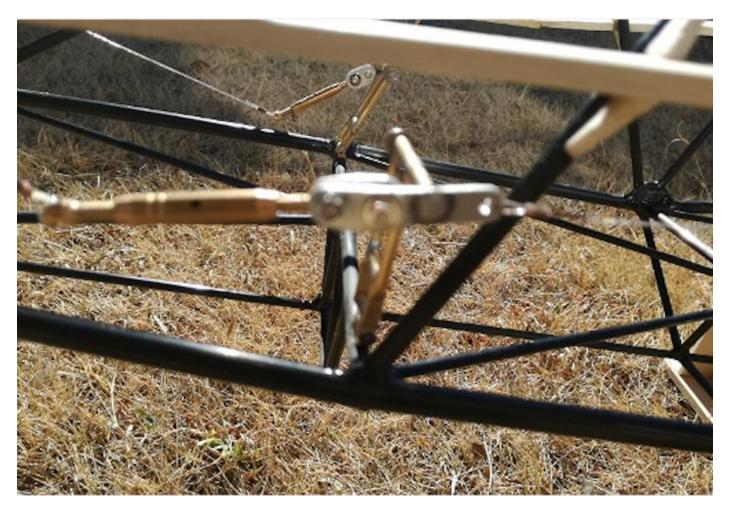
Photo 130: Installation of pedals Left, front seats. Right, rear seats.
