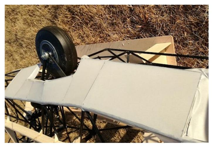
**Photo 134** (left): Structure around the main landing gear seen from the front. | **Photo 135** (right): Trial application of the Oratex.
