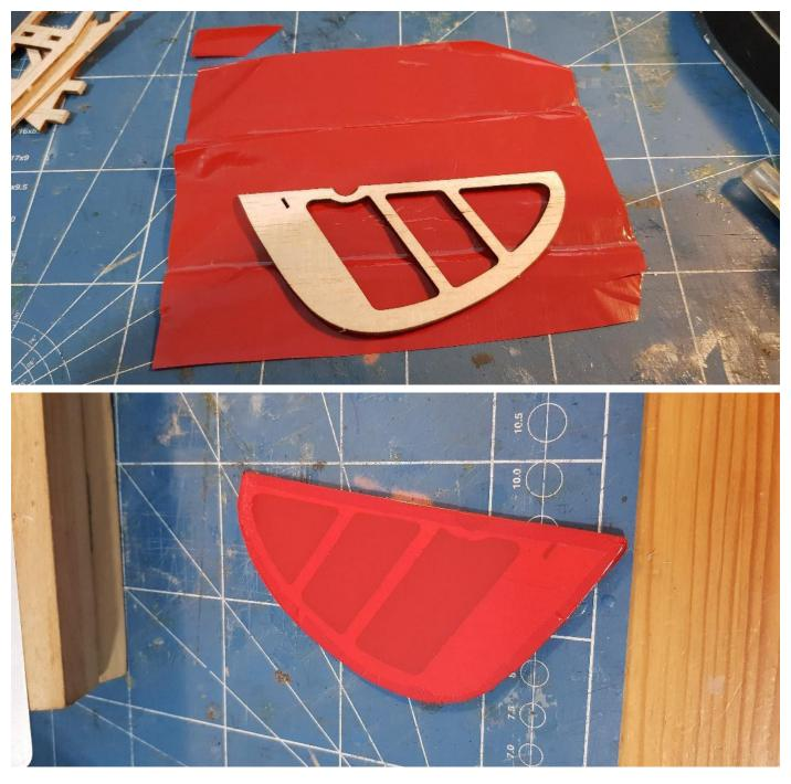
26, 27: First experiment; covering the rudder in one piece. Do-able.
