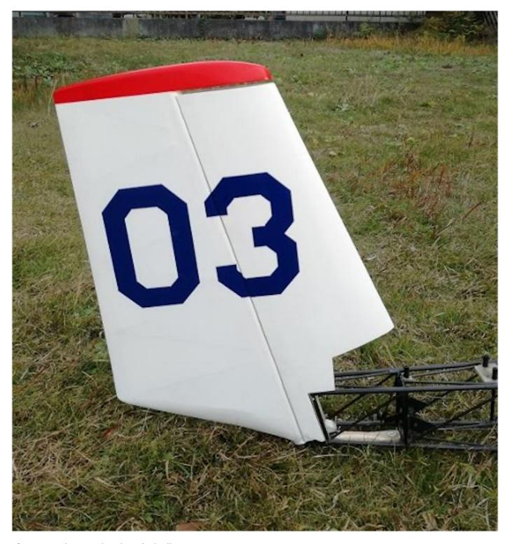
Photo 111: The completed vertical tail.
