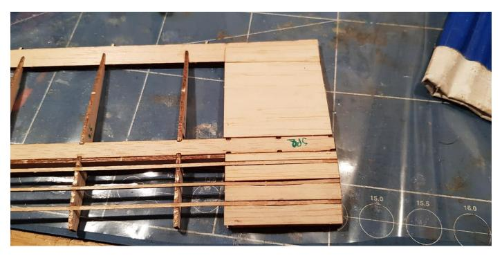
10 through 17: The basic build sequence for the wing. The leading edge is added on later.
