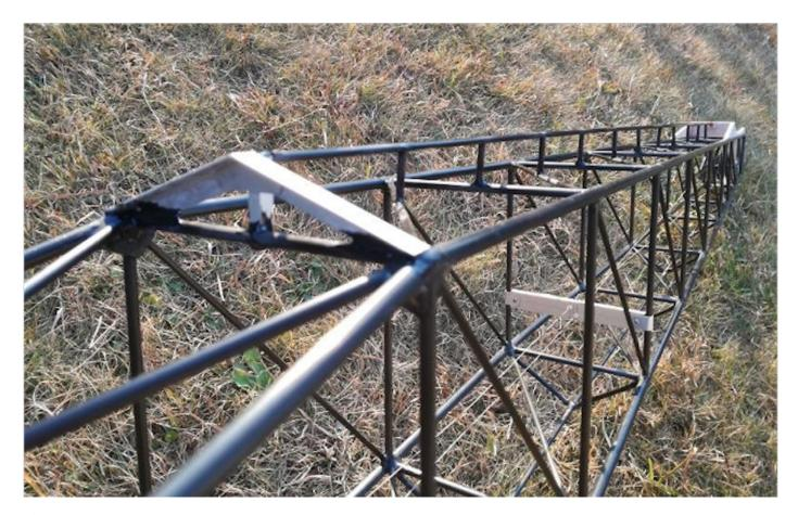
**Photo 115**: Front part of the upper overhang structure.
