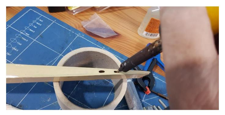
30: Opening up holes with a warm soldering iron.
