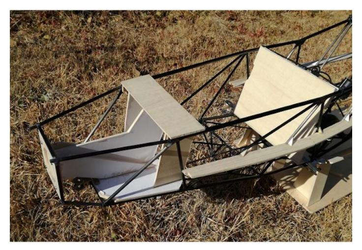
Photo 124: Simple assembly jig.
