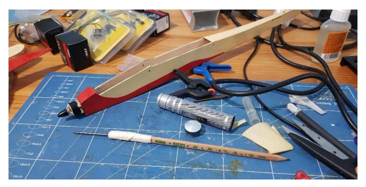
**34**: Fitting the tiny motor into the even tinier fuselage. My custom, 'extended reach' Allen driver is in the foreground.
