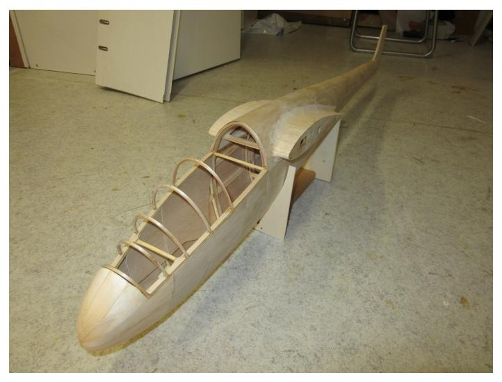
17 (top left), 18 (top centre): Bending ply across the grain. | 19 (top right): Glued in place. | 20 (bottom left): Fairing completed. | 21 (bottom right): Fuselage roughly finished.
