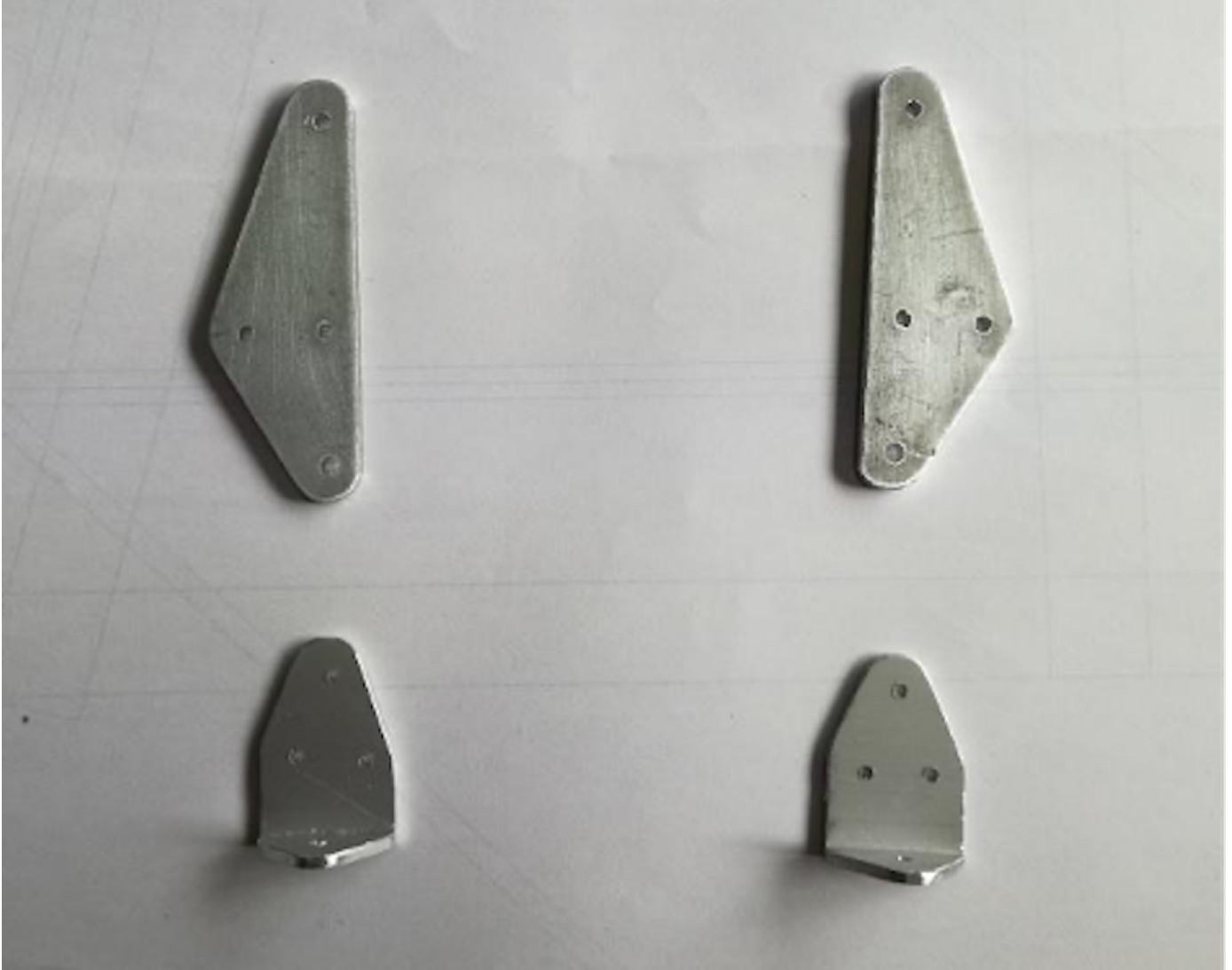
Photo 96: Wing fuselage joint fittings: top, front side; bottom, rear side.
