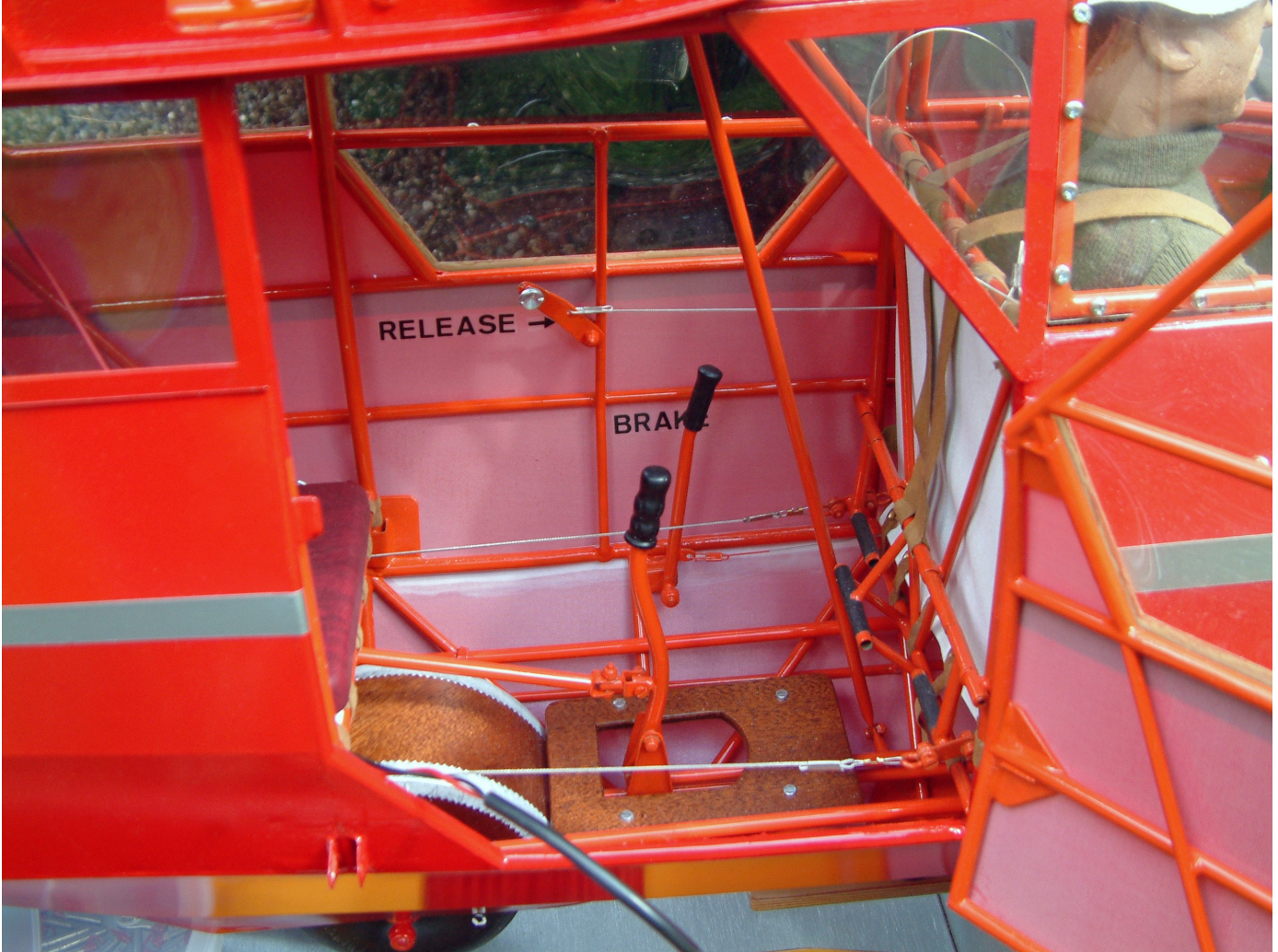
Left: The Rétroplane prime mover: Vincent Besançon displays his exquisite ¼ scale Frankfort Cinema. Right: The Cinema's fuselage is made up of silver-soldered steel tube.
