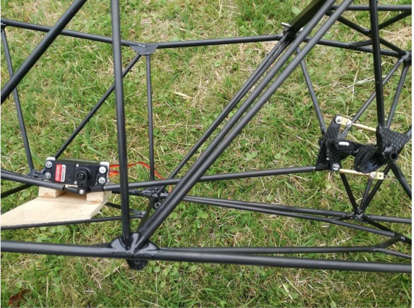
Photo 88: Elevator servo and front side bellcrank.
