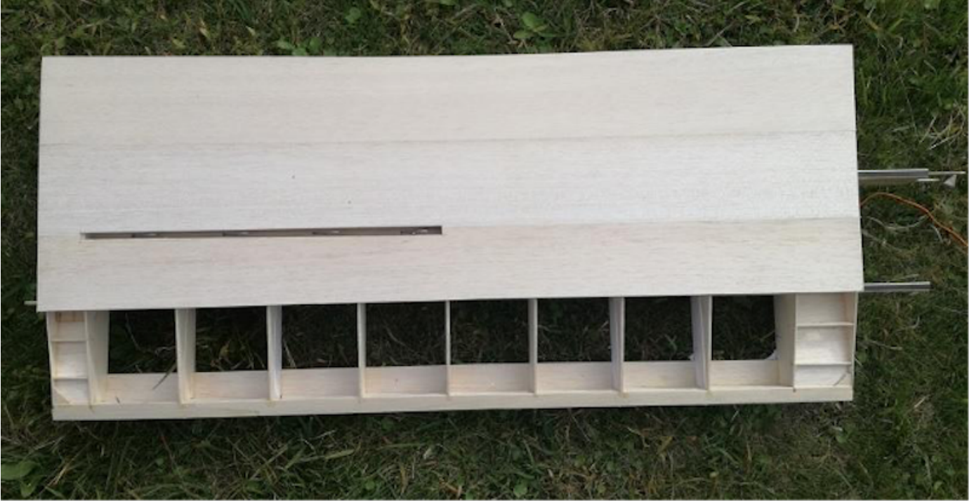
Image 93: Aligning the upper plank material.
