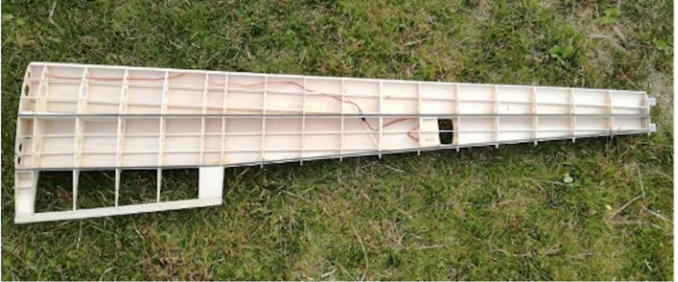
Photo 106: The outer wings with the lower plank completed.
