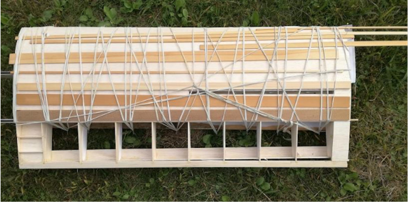
Image 94: Upper plank of the center wing.
