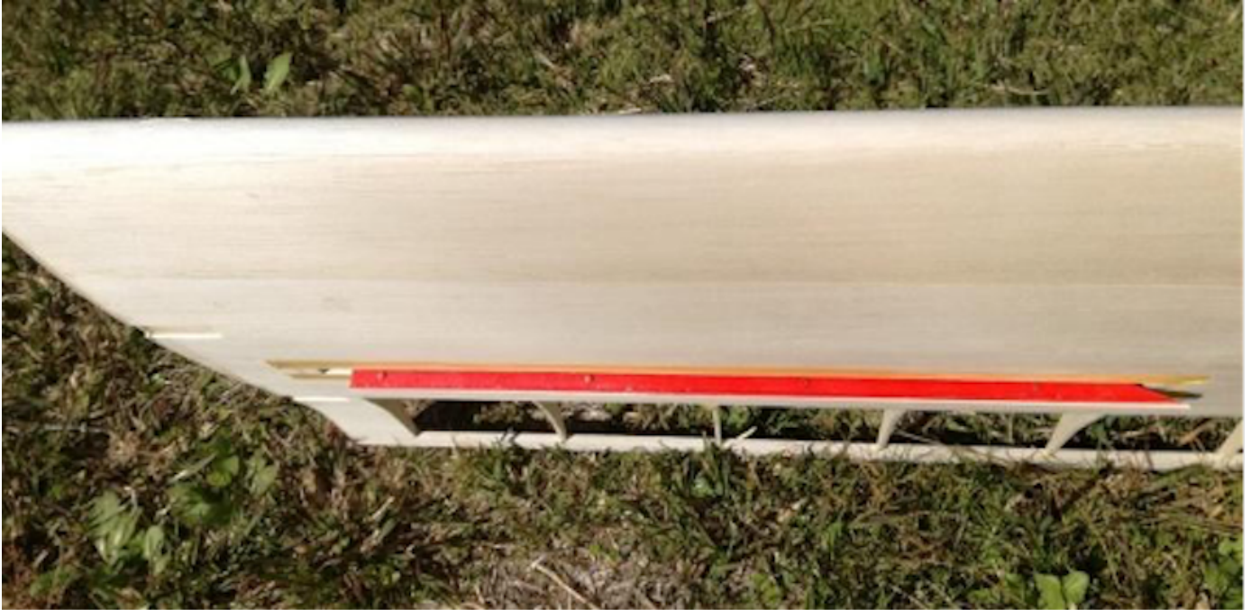
Photo 101: Checking the spoiler open state: left, upper side; right, lower side.
