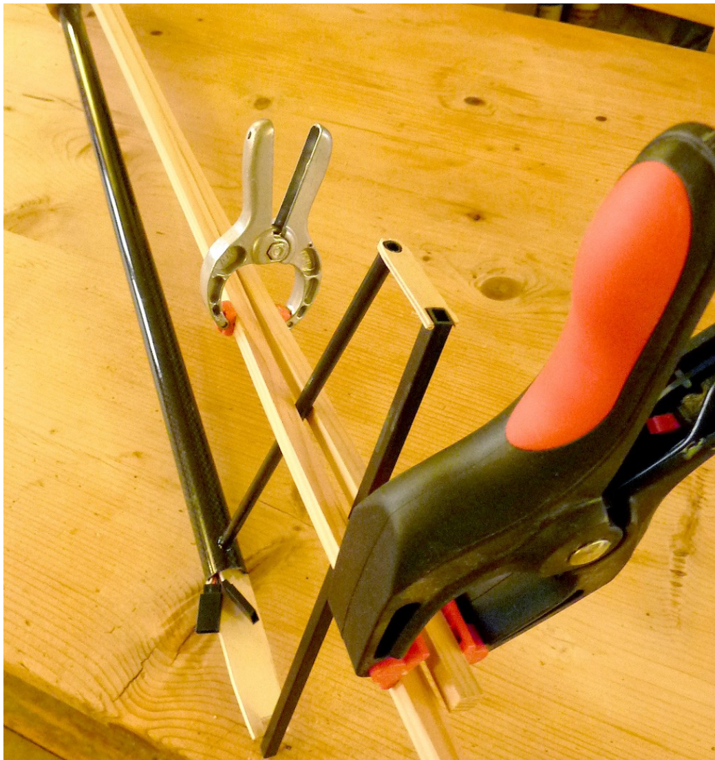
Photo 9: Two spruce spars clamped onto the fin uprights.
