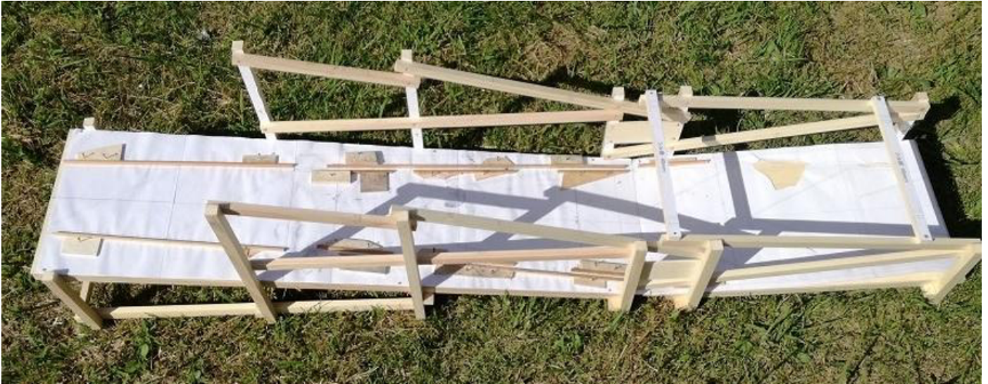
Photo 71: Completed fuselage assembly jig.
