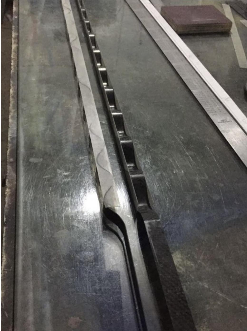
Photo 7: An early experimental ASWS on some G10 glass plate. This method was abandoned in favour of direct bonding to the spar caps. (image: James Hammond)
