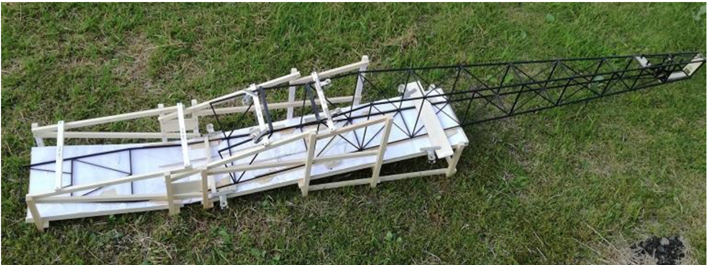
Photo 72: Temporary mounting on the assembly jig.
