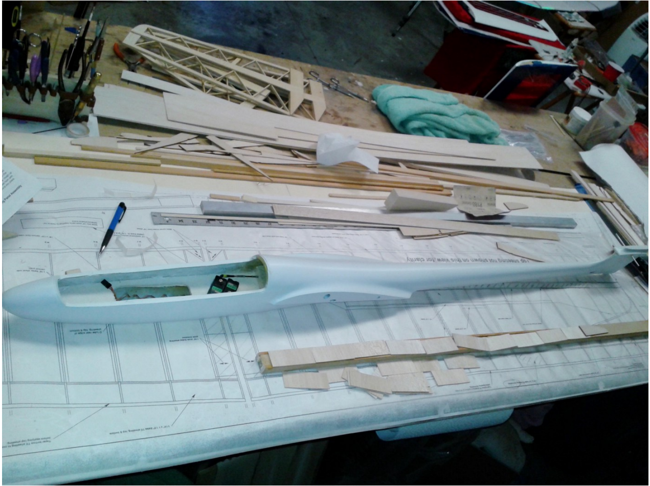
Photo 27: The nose on this Aquila was fuse totally demolished, but I managed to put Humpty Dumpty back together again. After some sanding and filling, the fuse came out great.
