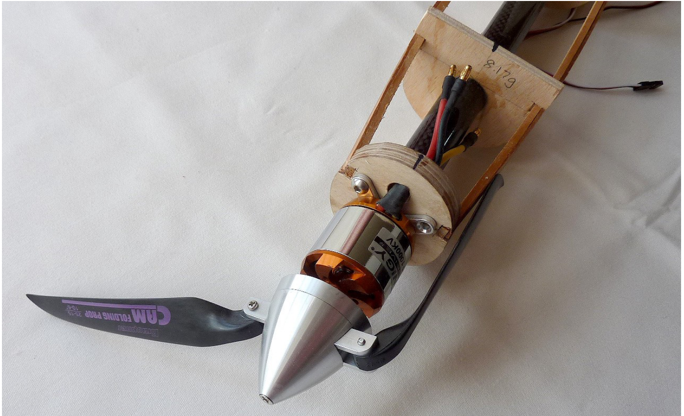
Photo 10: The motor mounted on the motor bulkhead.
