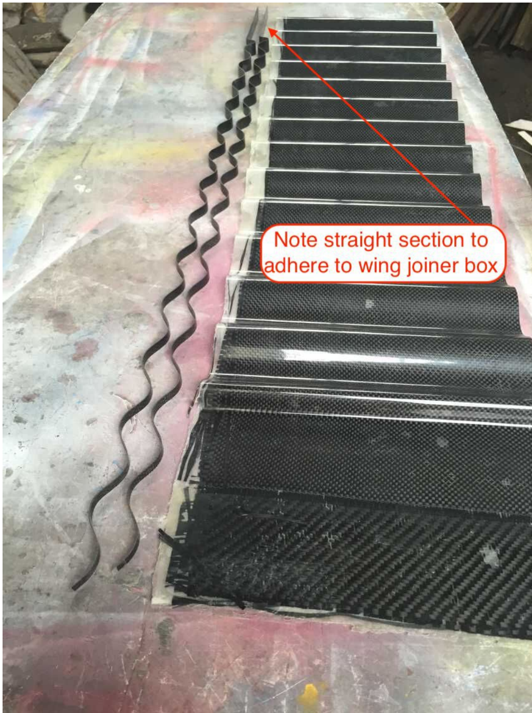
Photo 4: A whole sheet of early spars. Later the carbon was reduced and carefully oriented for optimum strength. (image: James Hammond)
