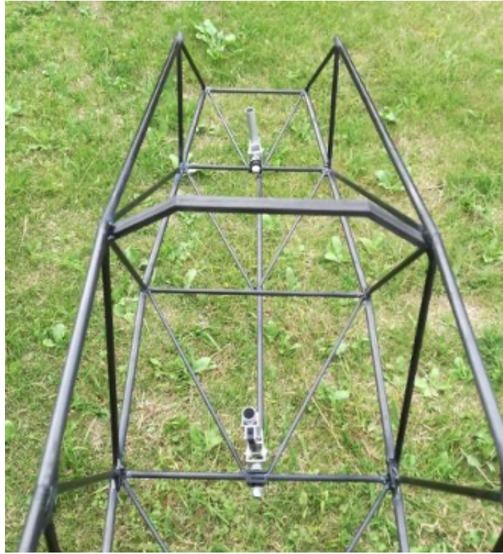
Photo 85: Installation test of the gimbal mechanism.
