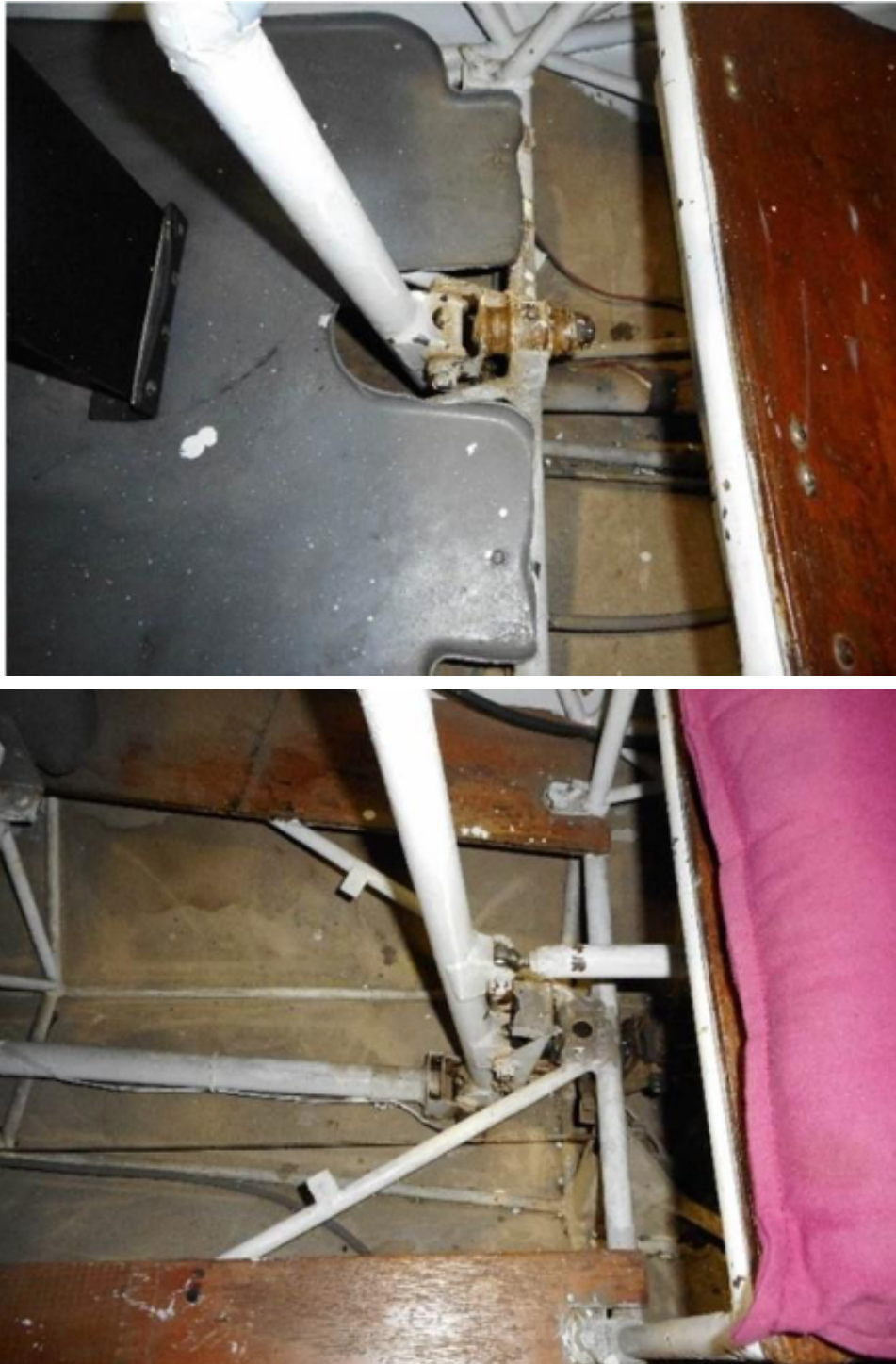
Photo 81: Gimbal mechanisms of the actual aircraft; left = front seat, right = rear seat.
