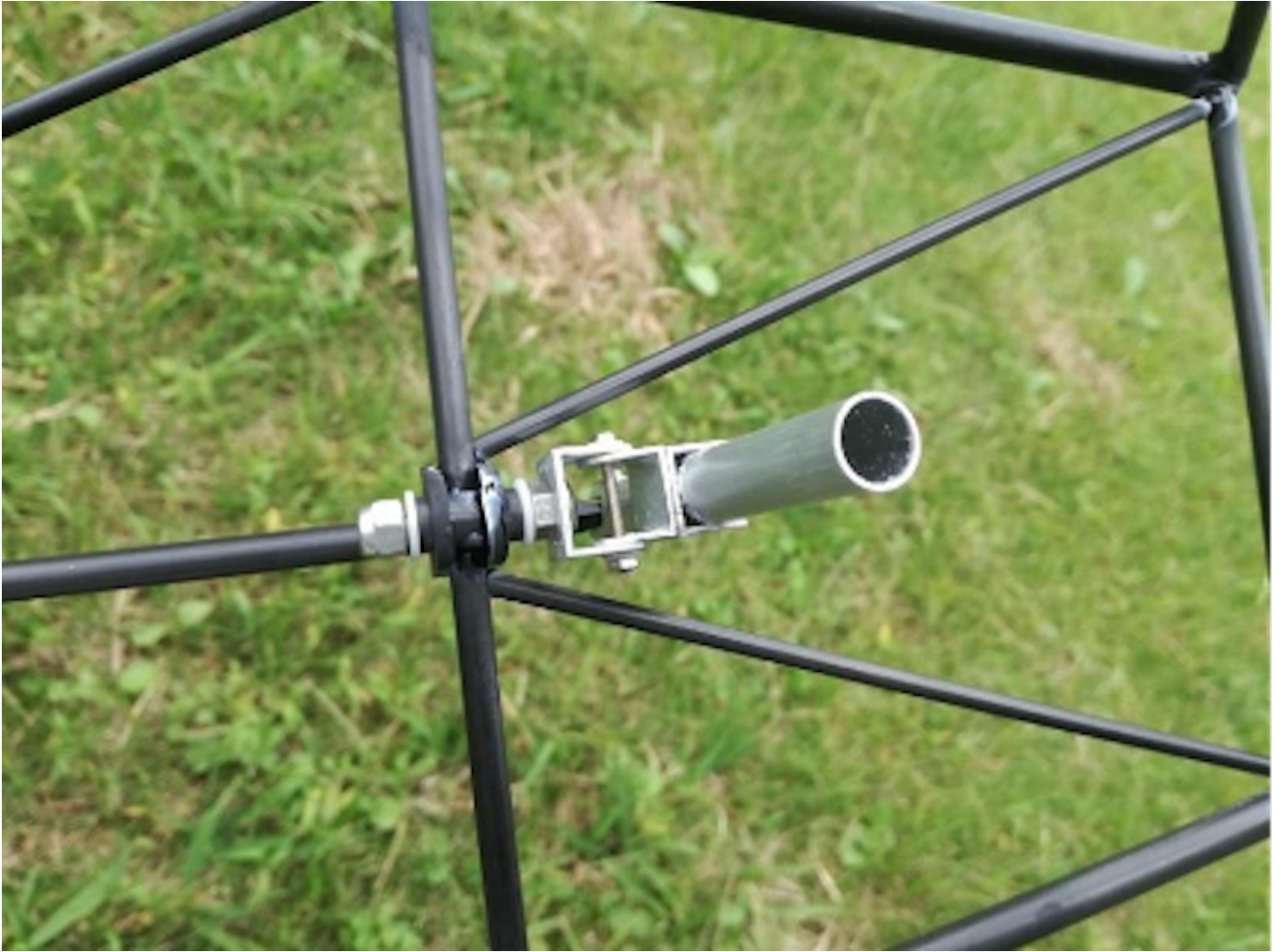
Photo 86: Close-up view of the gimbal mechanism.
