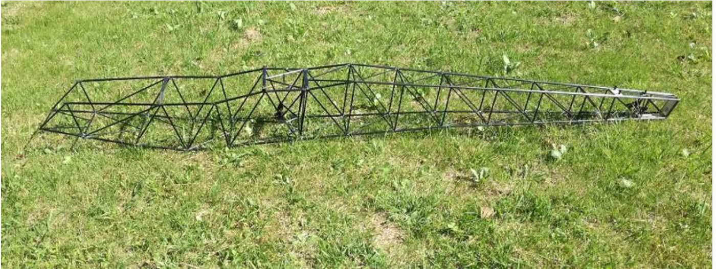
Photo 77: Main structure of the completed fuselage.
