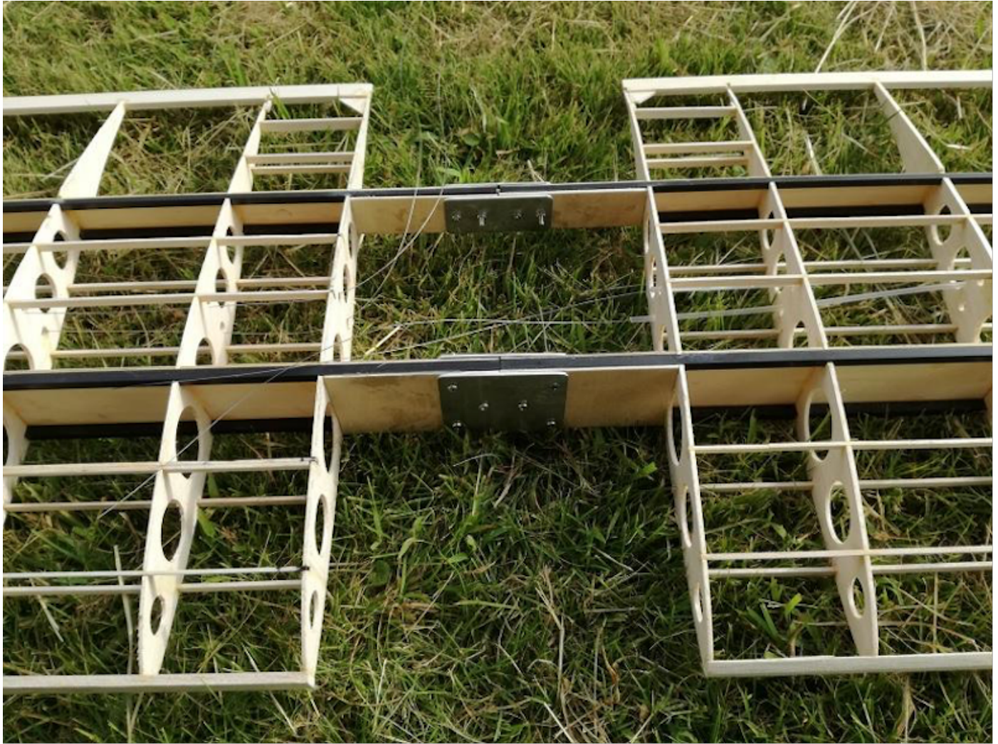
Photo 65: Testing the left and right connection.
