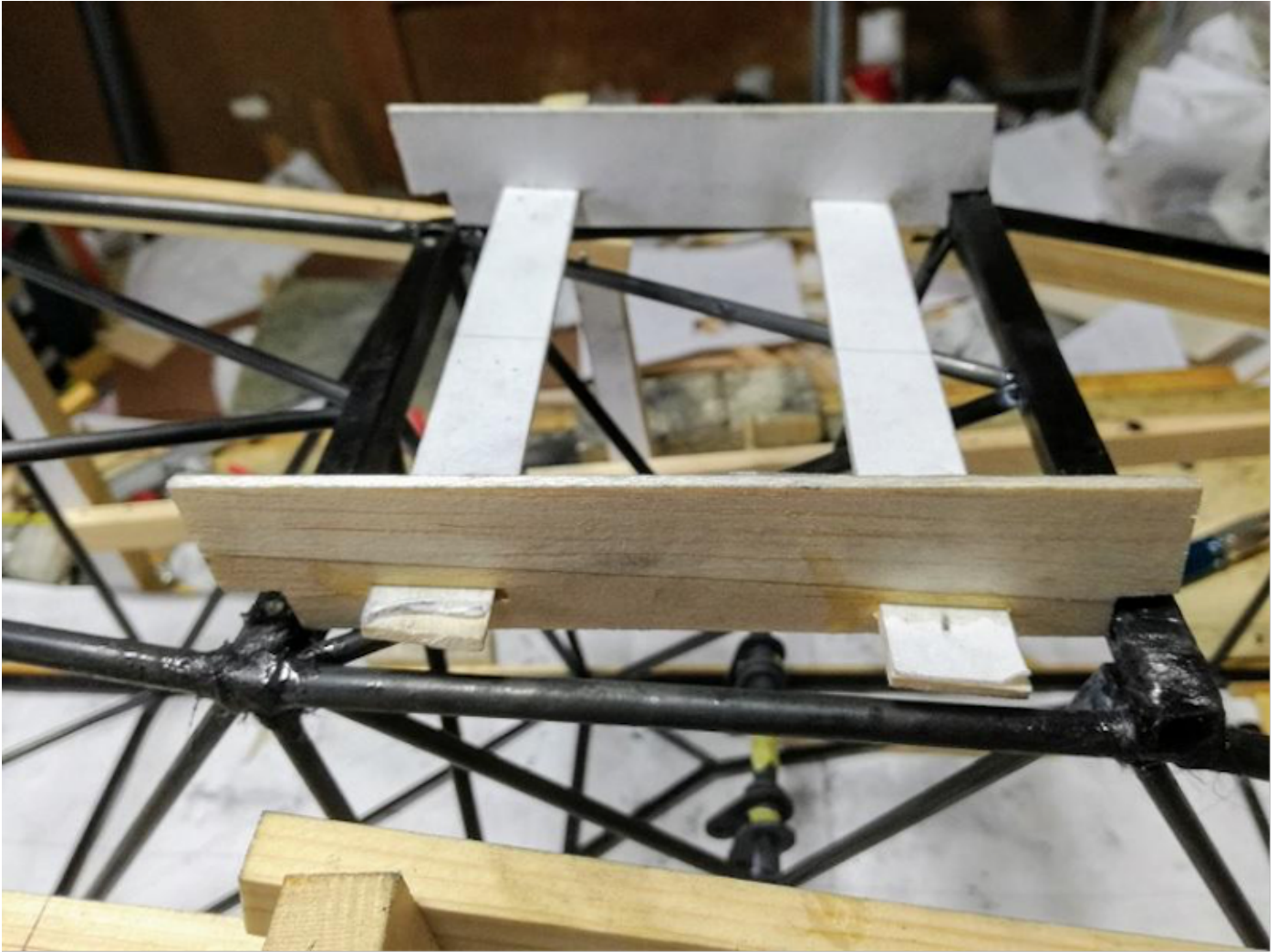
Photo 76: Positioning jig for main wing attachment beams.
