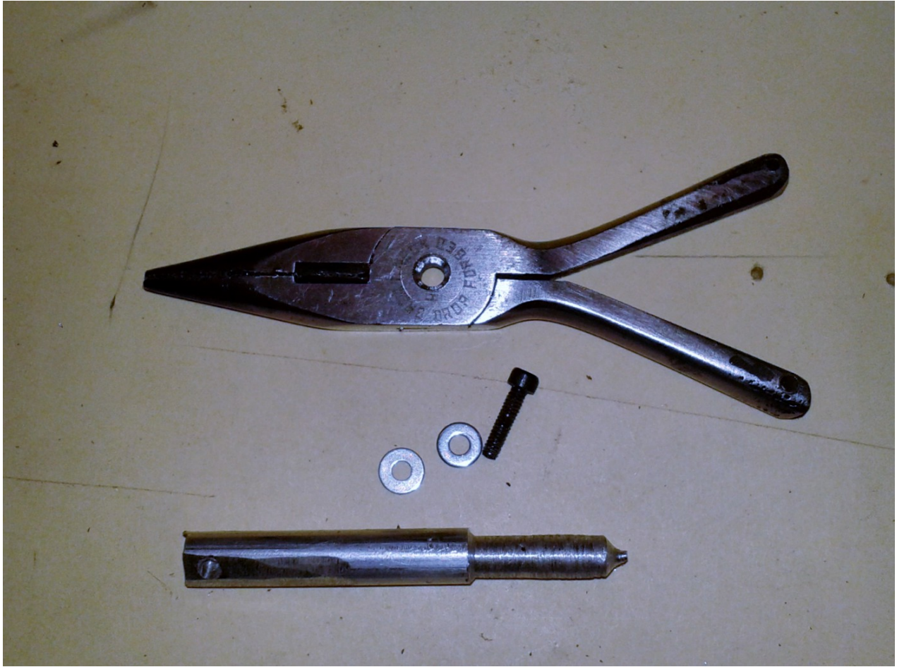
Photo 12: I drilled through the center of the pliers, took a piece of aluminum rod, turned down one end to fit the tube, drilled and tapped it for a tiny socket head cap screw. You could just as easily fill the rod with epoxy or a dowel and put the pliers right on the rod. Just account for that when making the slots.
