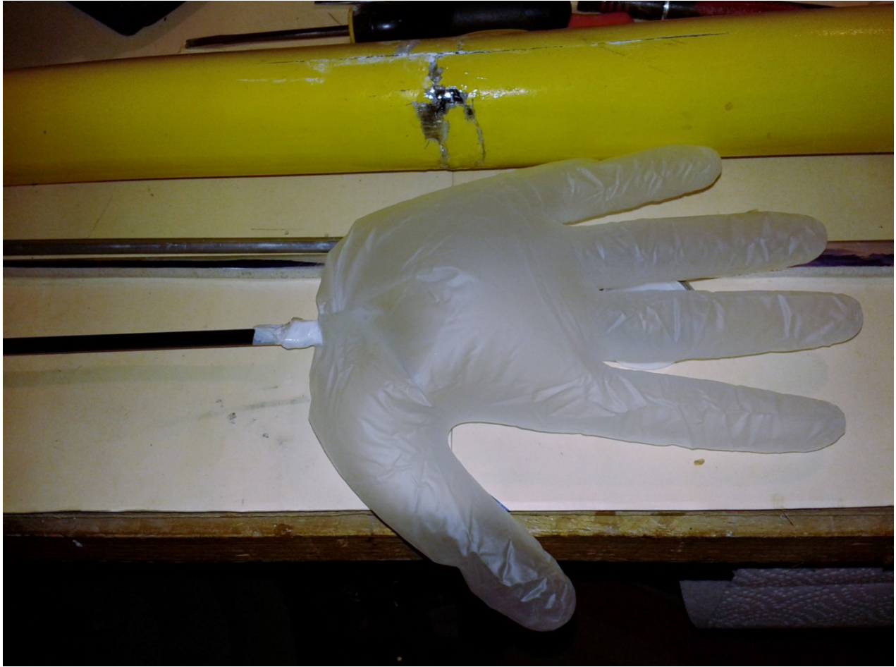
Photo 26: Ran the balloon in to the right spot and blew it up gently. Then blew hard to pop it and pulled it out. I did it again with a surgical glove since I ran out of balloons. I left it in until the epoxy got tacky and then blew until it popped and pulled it out.
