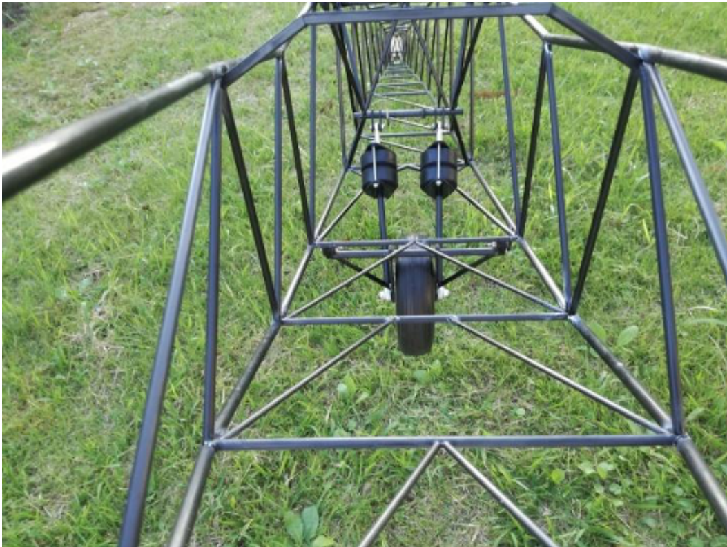
Photo 80: Temporary installation of the main landing gear.
