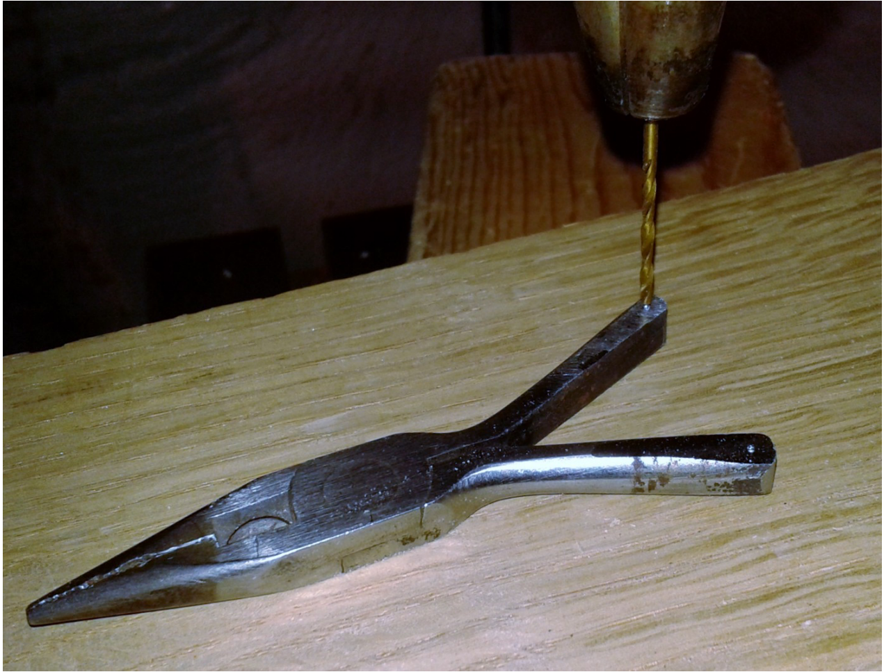
Photo 8: After cutting and grinding, I drilled a couple of holes for the pushrods.
