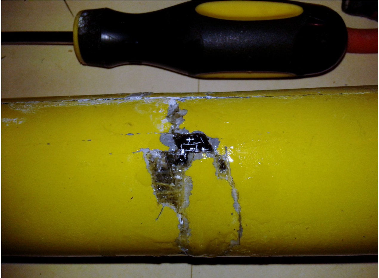
Photo 25: Put a little extra epoxy in the big holes. I had dripped in some extra epoxy before running the cloth in also.
