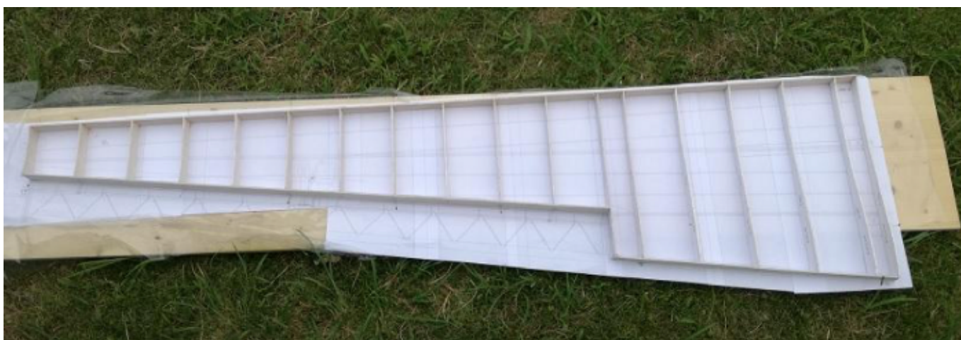
Photo 44: Assembly jig of the left outer wing
