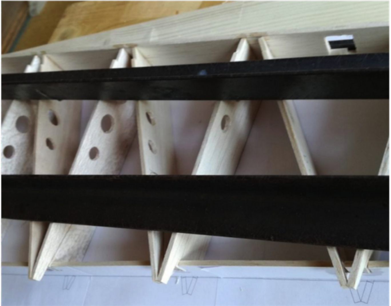
Photo 17: Rib assembly of the rudder.
