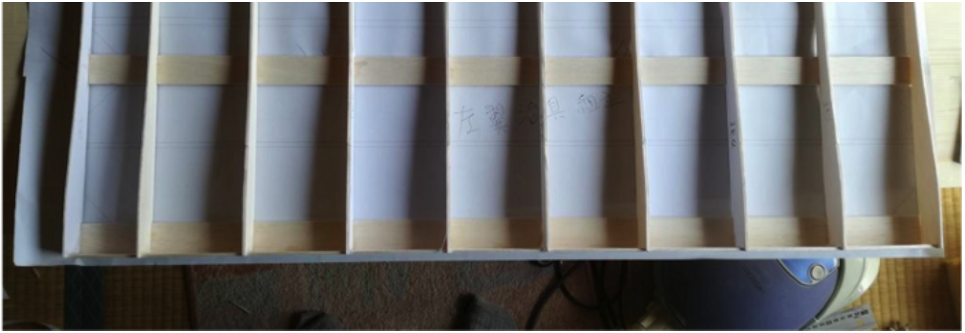
Photo 9: The center wing assembly jig completed
