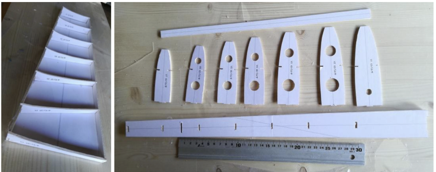
Photo 19: Assembly jig and parts of the vertical fin.
