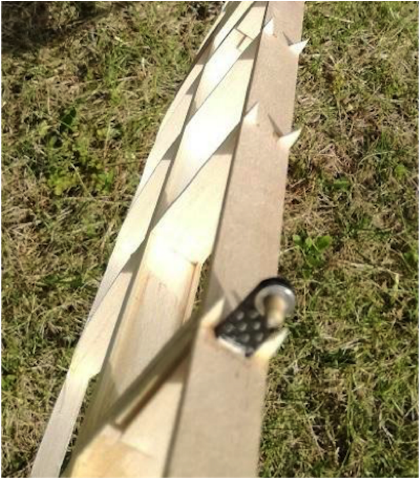
Photo 25: Completed rib assembly of the horizontal fin.
