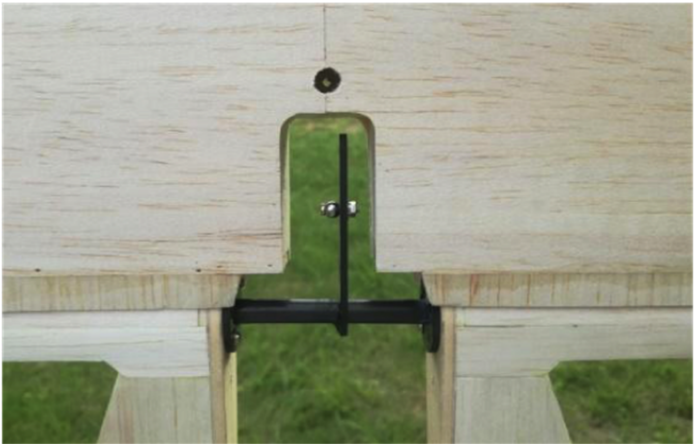
Photo 28: Elevator connecting part.
