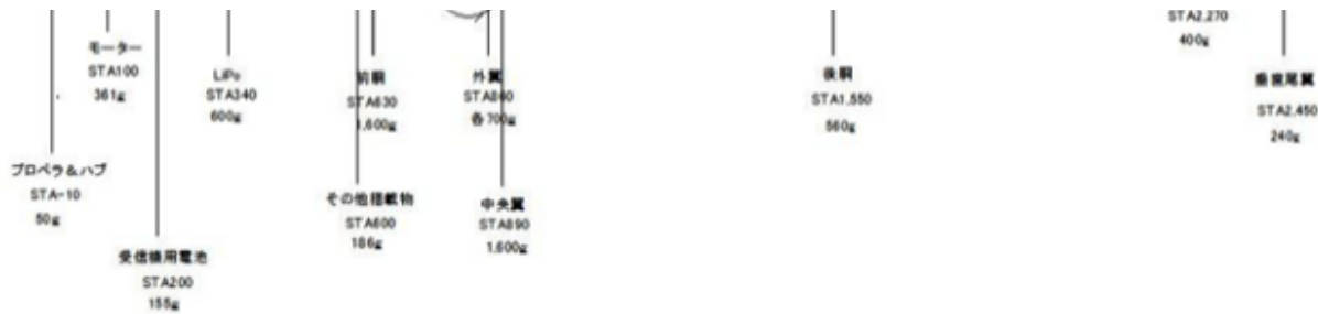
Drawing 6: Weight of each component and its position.
