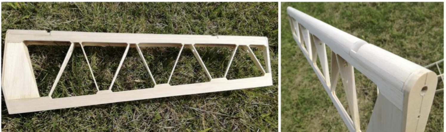
Photo 23: The left elevator completed.
