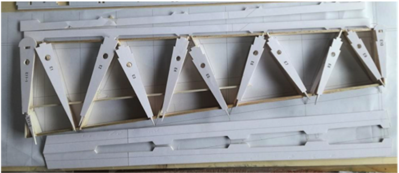
Photo 22: Elevator components placed on its assembly jig.
