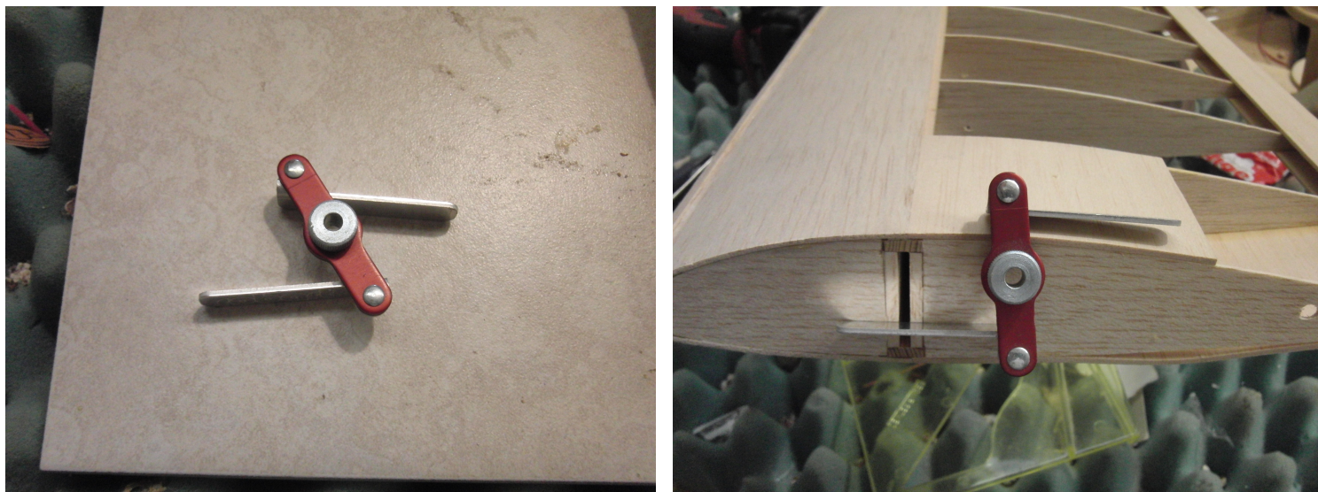
Photos 1 and 2: The Robart Hinge Point Drill Jig which I simply refer to as their center finder because that's what it actually does.
