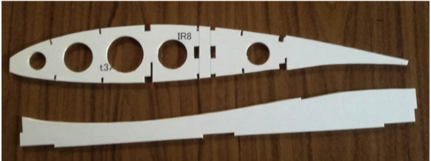
Image 8: Cut-out rib and assembly jig component
