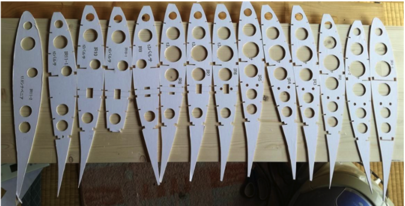
Photo 10: Ribs for a half center wing.
