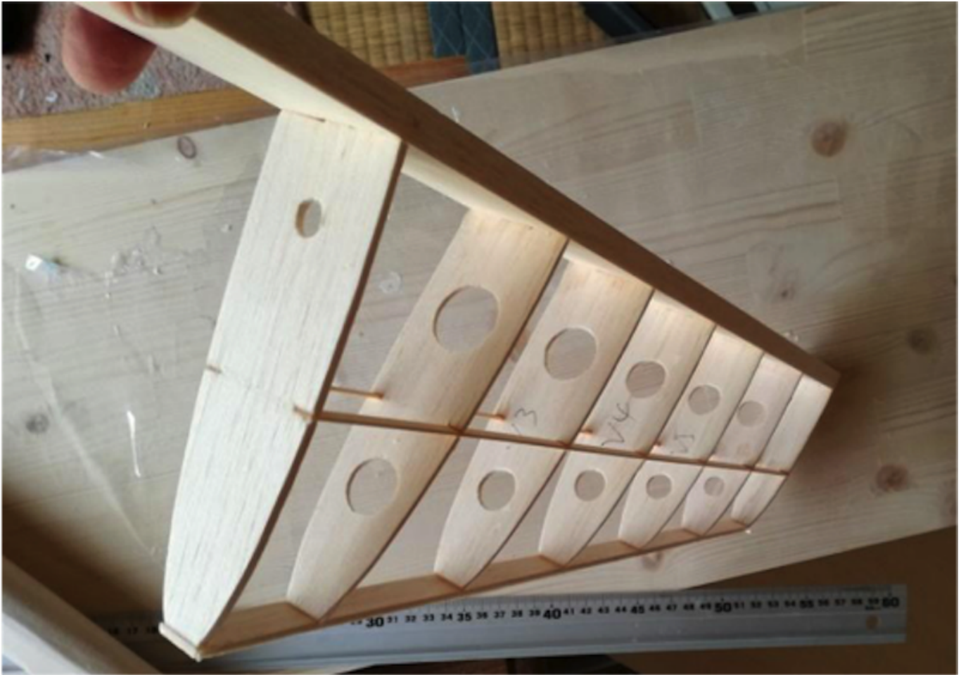
Photo 20: Vertical fin rib assembly.
