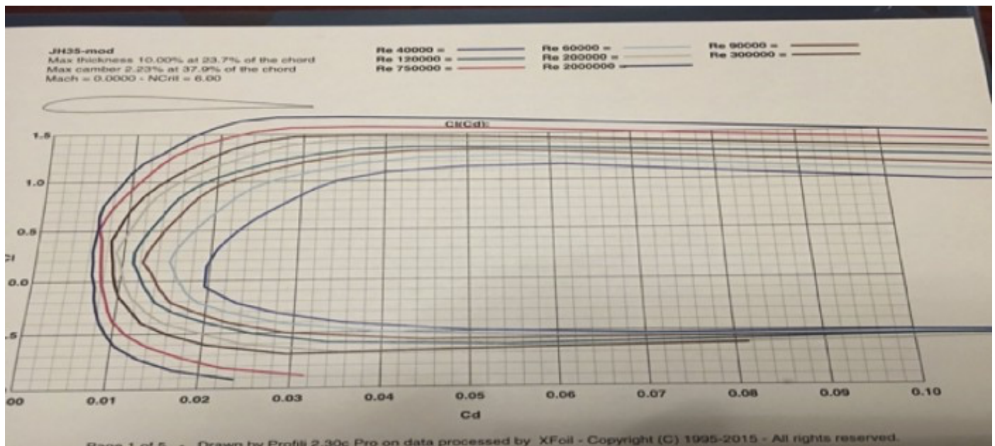
Photo 3: A set of L/D curves for the JH35 Alpine soaring section.
