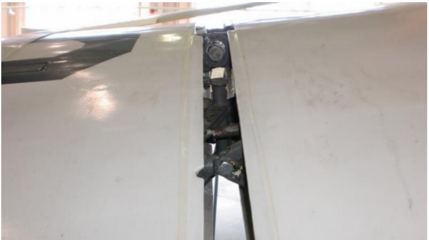
Photo 3: Joint of the center and outer wings of the actual aircraft.
