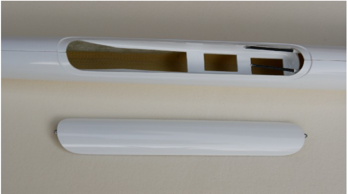
Photo 3: The servo tray is molded and drilled perfectly, with Kevlar reinforcement toward the nose
