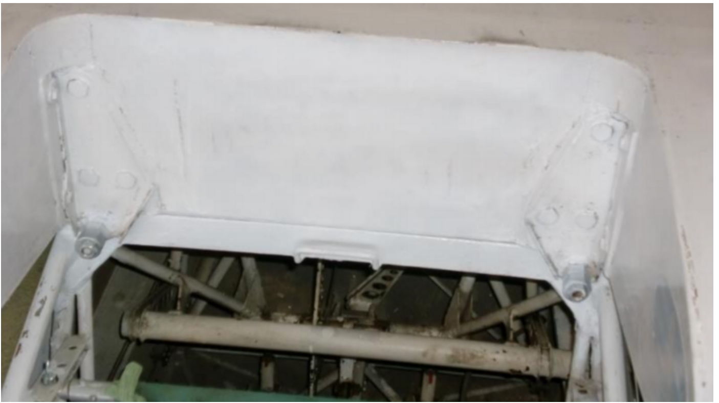
Photo 4: Wing-fuselage joint of the actual aircraft (front side).
