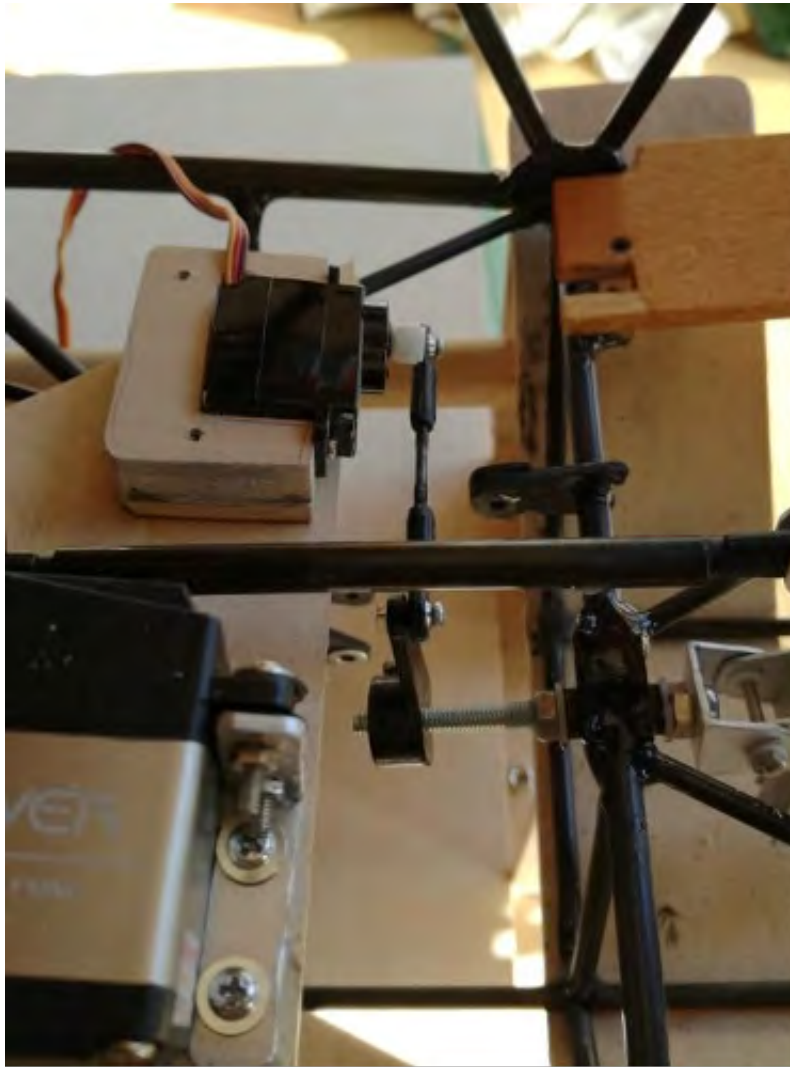
Photo 144: Dummy aileron servo installed.
