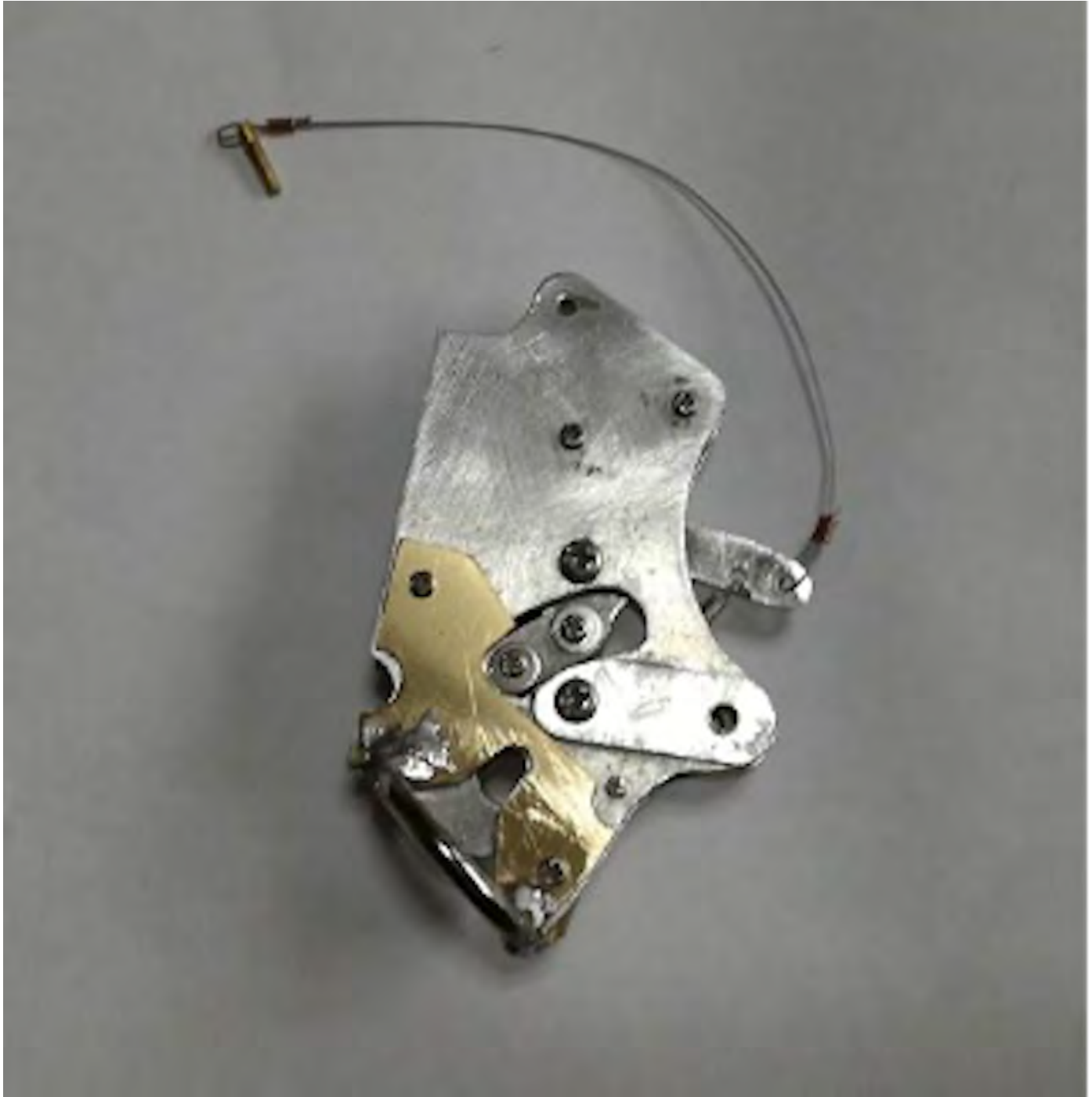
Image 149: Release mechanism with brass plates.
