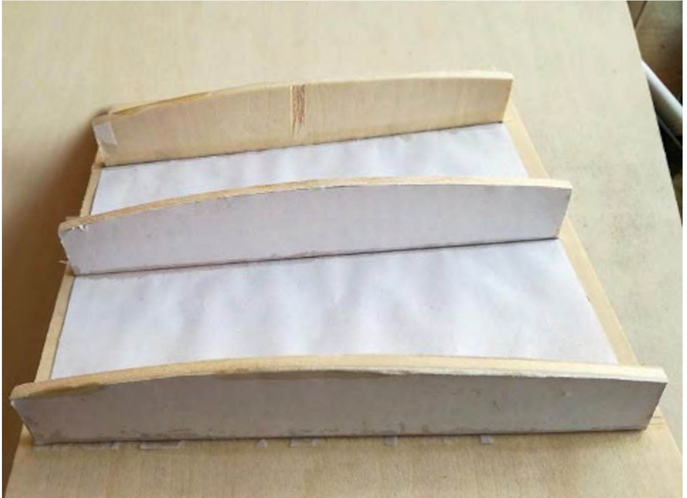
Photo 137: Assembly jig for the seat board and bamboo rods.
