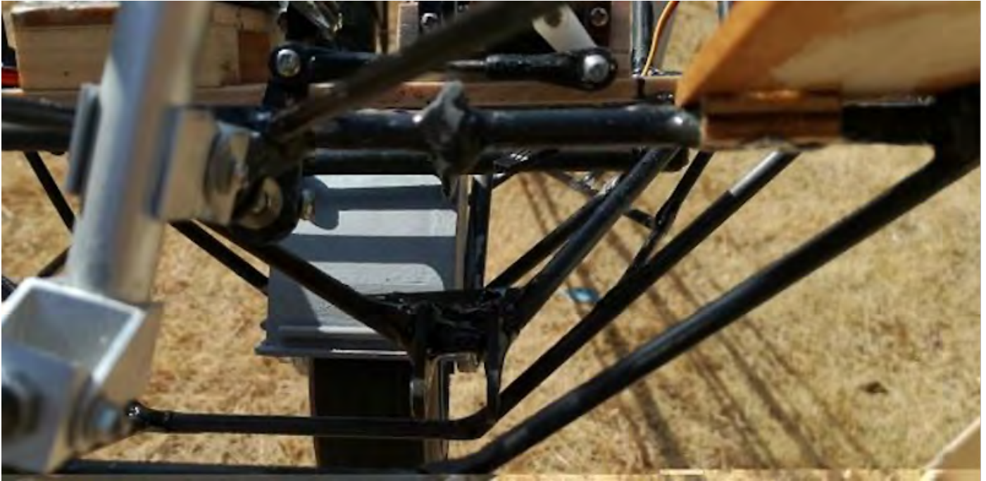
Photo 151: Assembly of the release mechanism mounting structure.
