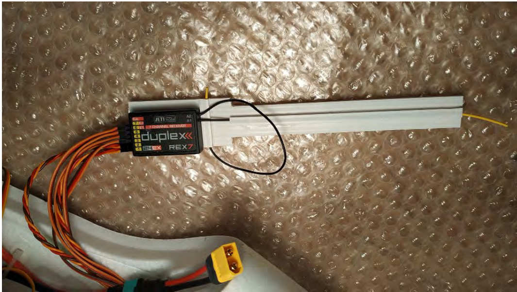
10: The receiver tray, made of corrugated plastic cardboard
