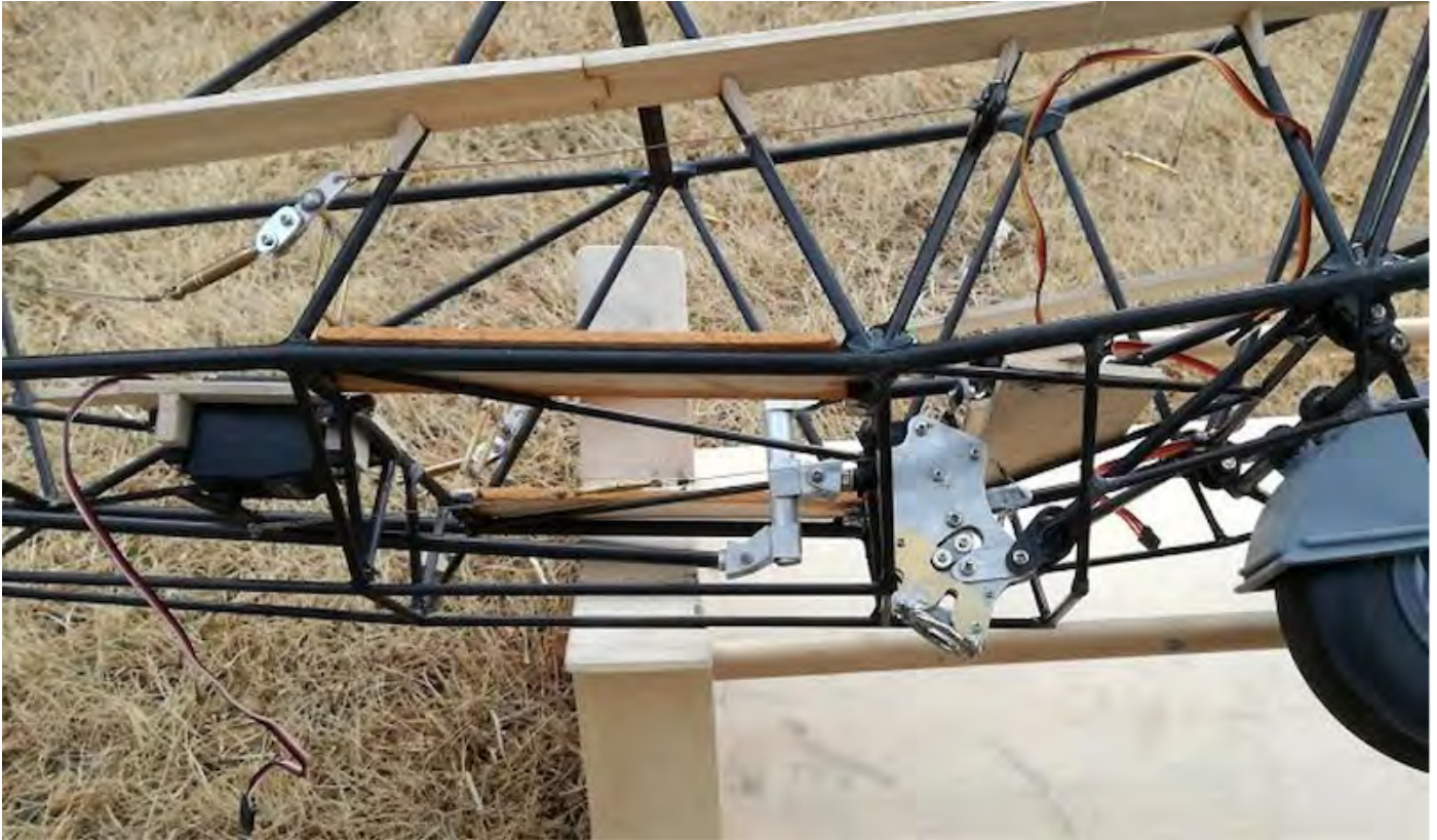
Photo 154: Release mechanism and its open/close servo.
