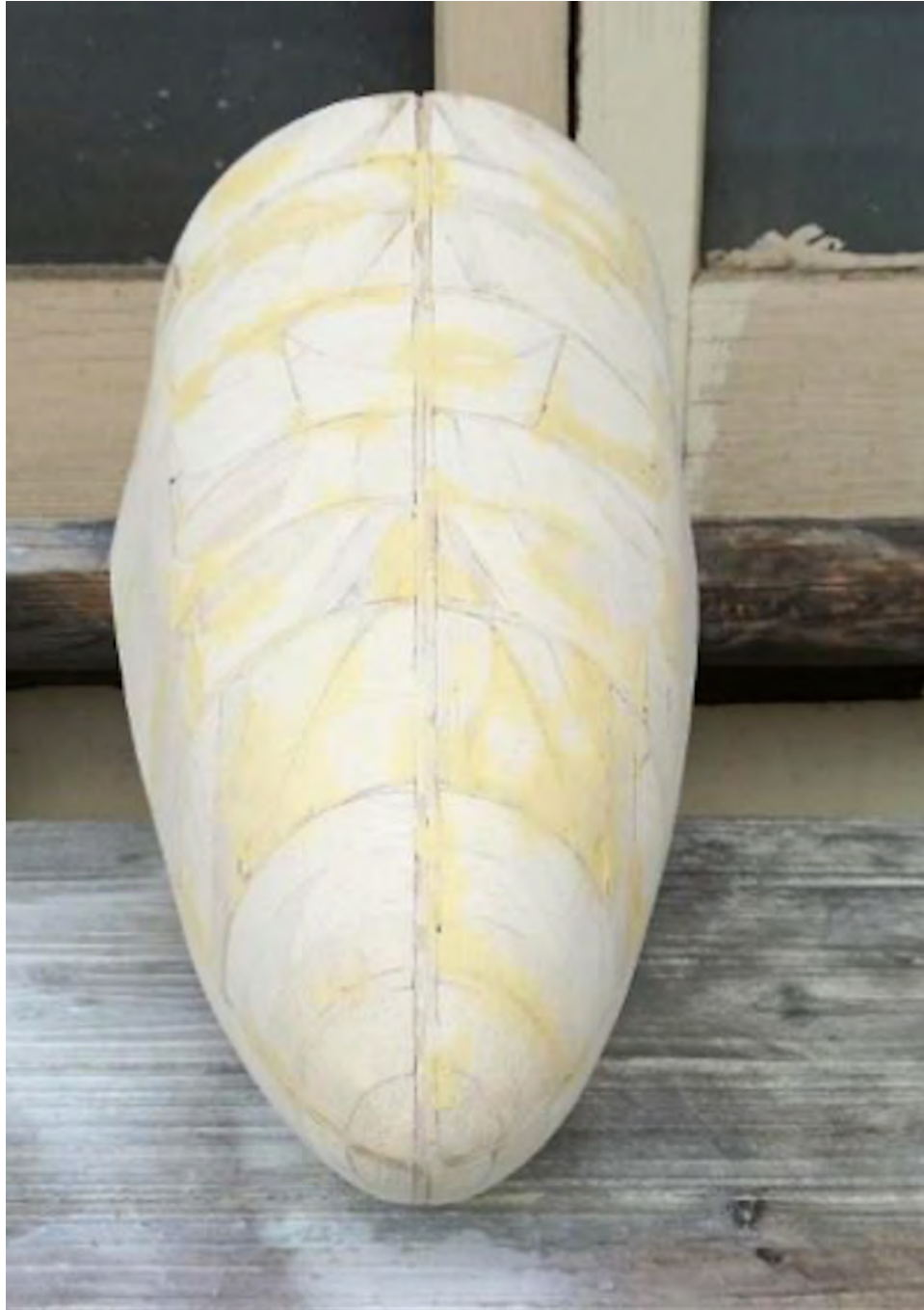
Photo 159: Pasting and shaping of the outer surface.
