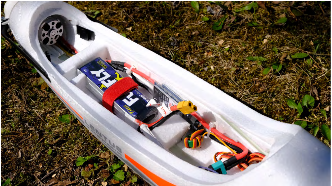
9: The front part of the fuselage with the ESC fixed on the side, letting lots of space for the battery
