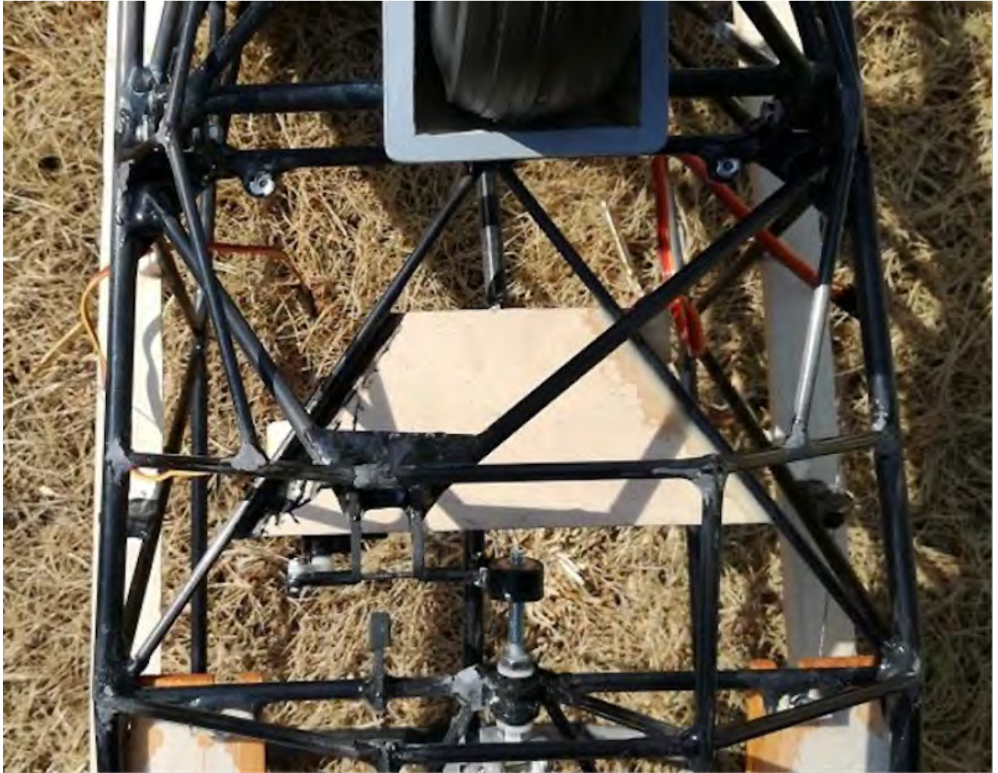
Photo 152: Back side of the release mechanism attachment structure.
