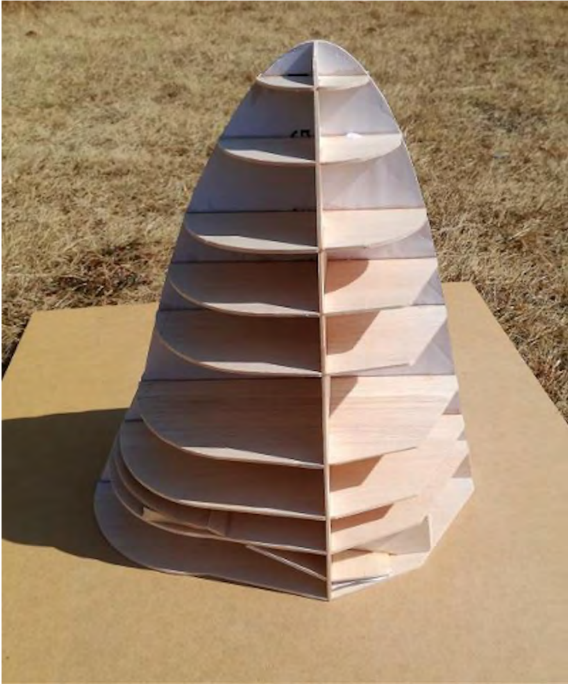
Photo 158: Cowling wooden skeleton.
