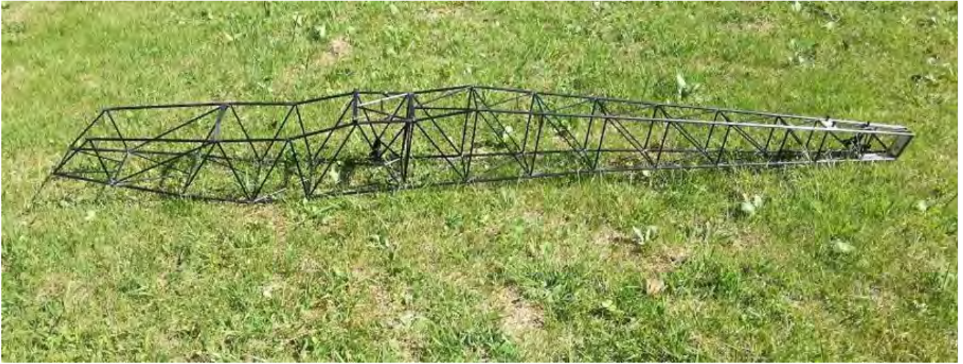
Photo 77: Main structure of the completed fuselage.
