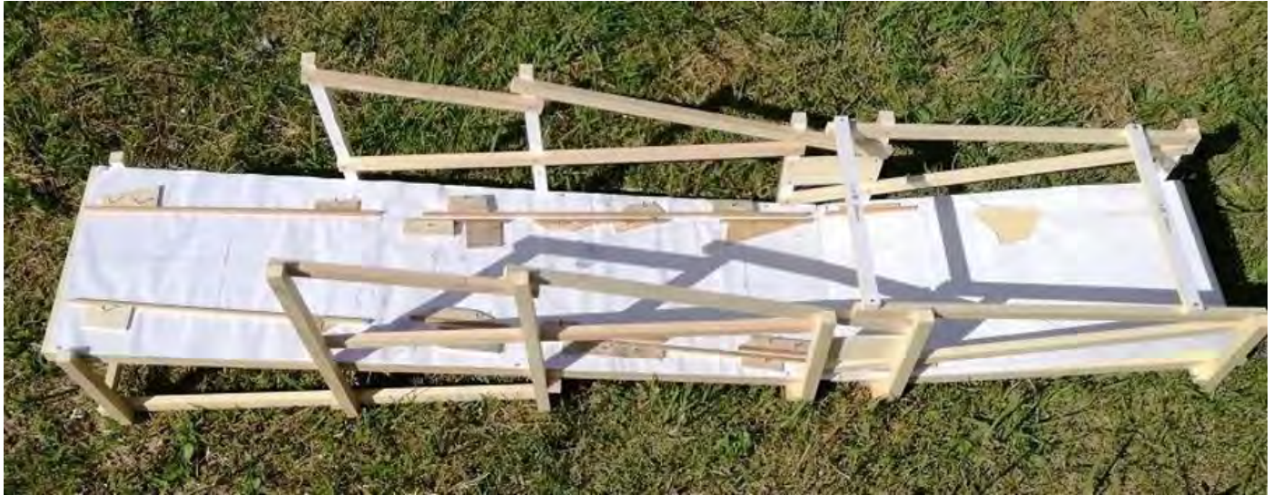
Photo 71: Completed fuselage assembly jig.
