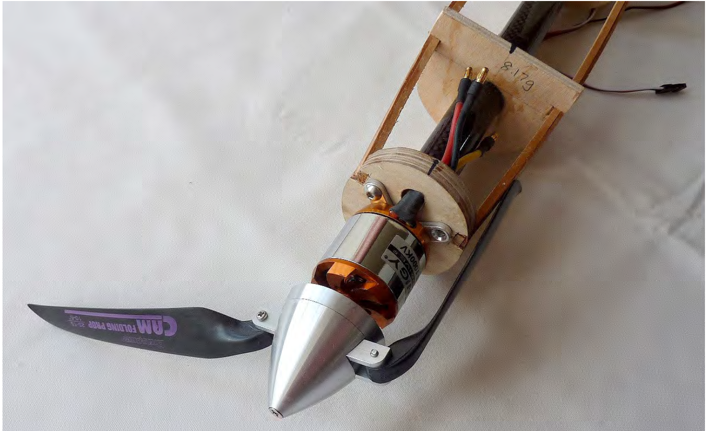
Photo 10: The motor mounted on the motor bulkhead.
