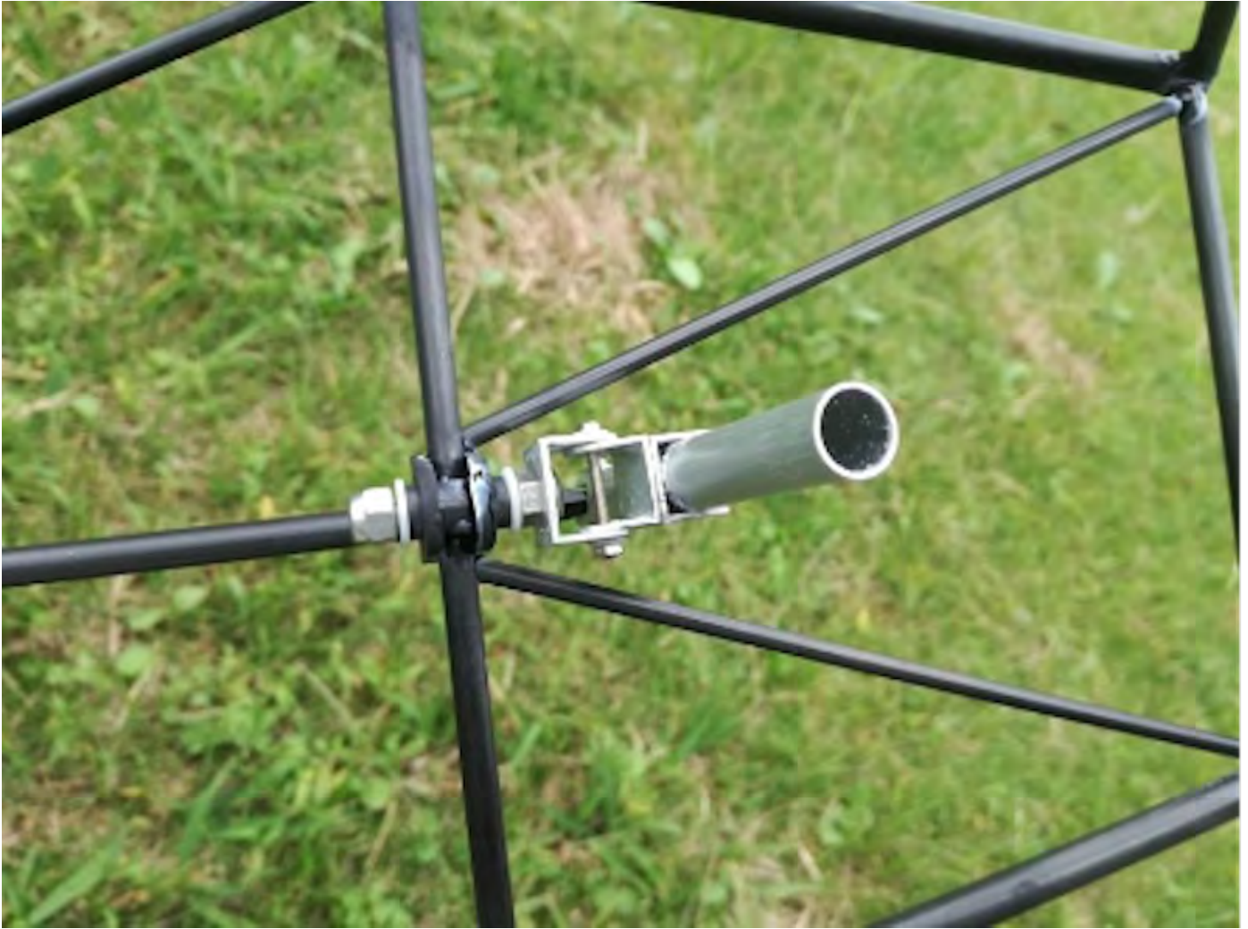
Photo 86: Close-up view of the gimbal mechanism.
