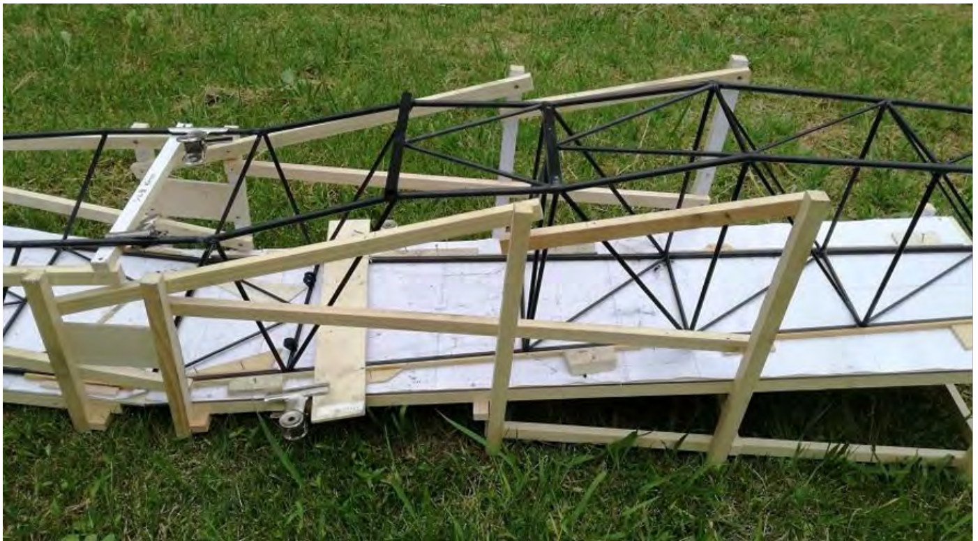
Photo 73: Front fuselage being assembled on the assembly jig.
