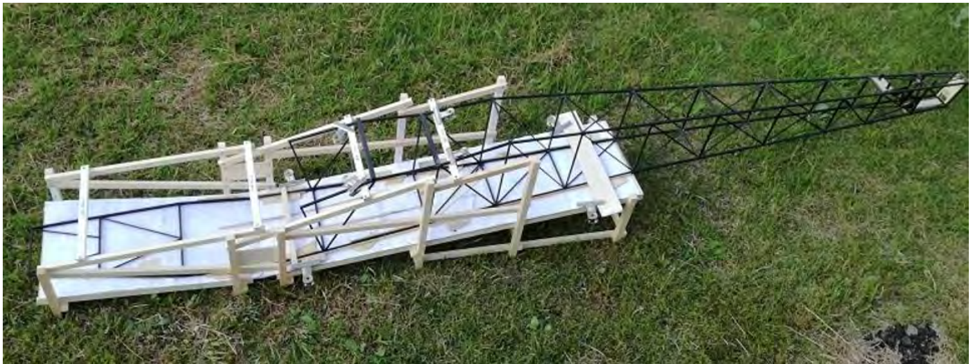
Photo 72: Temporary mounting on the assembly jig.
