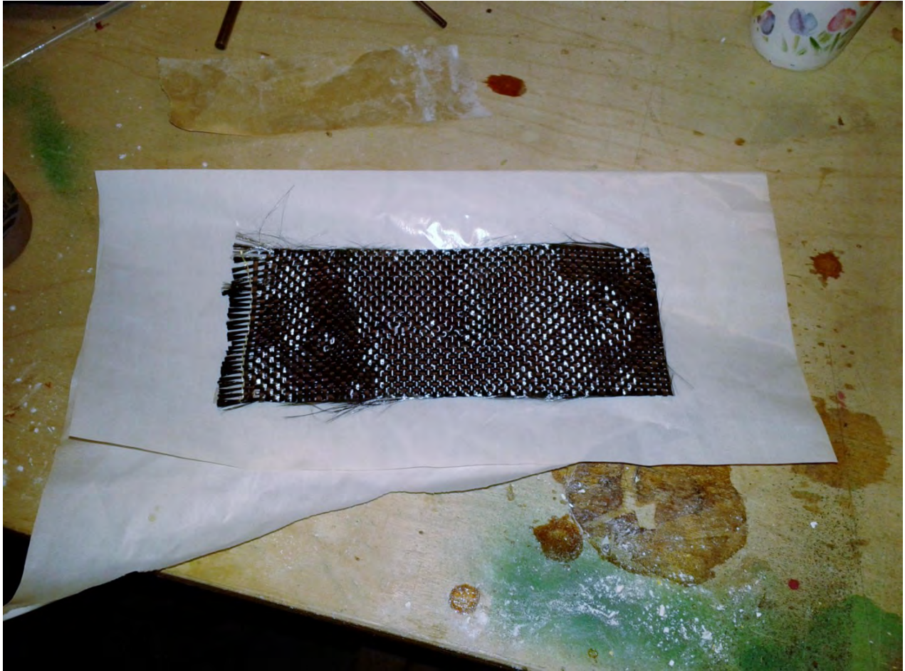
Photo 22: Cut and wet out a piece of carbon cloth.
