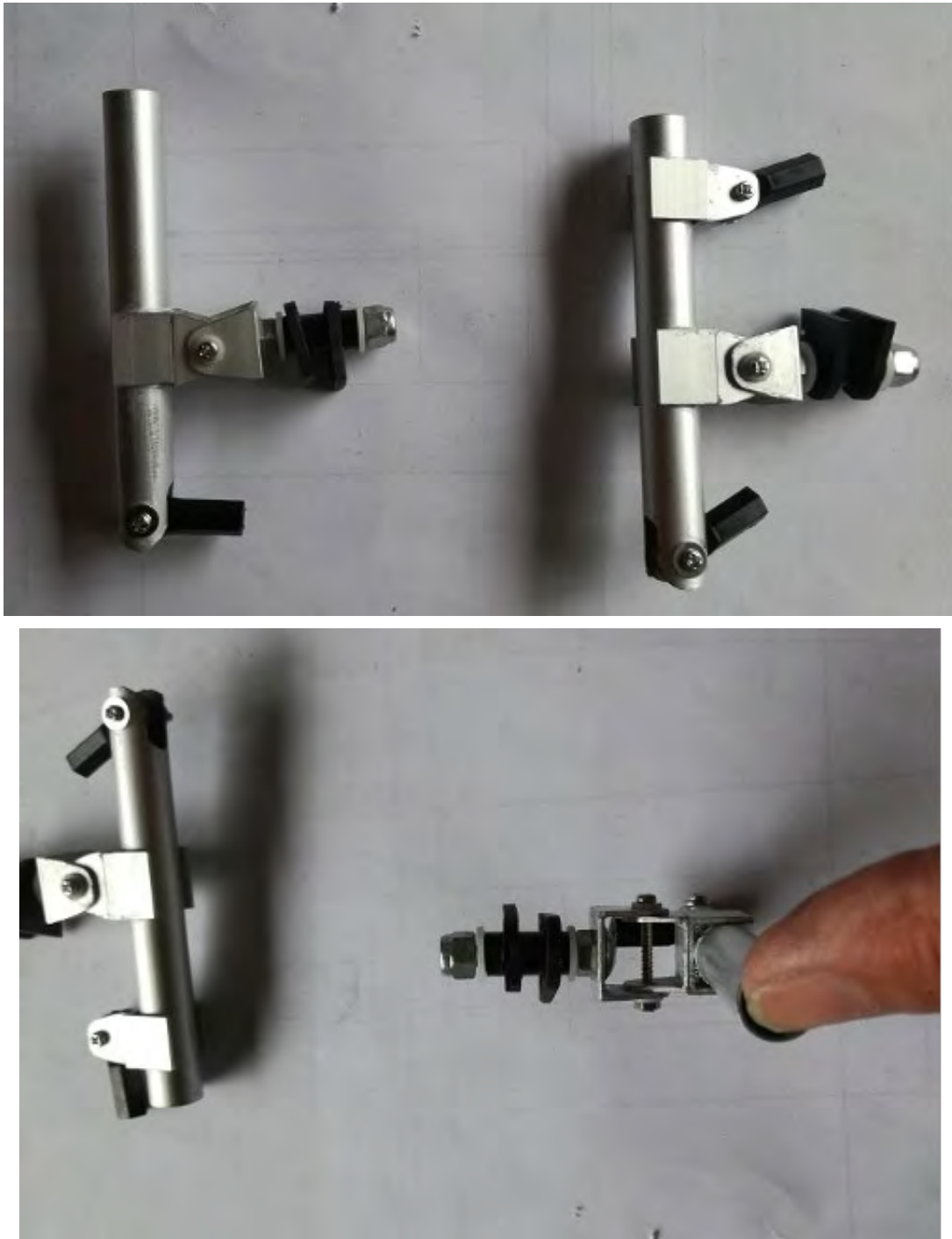
Photo 83: Assembled gimbal mechanism.
