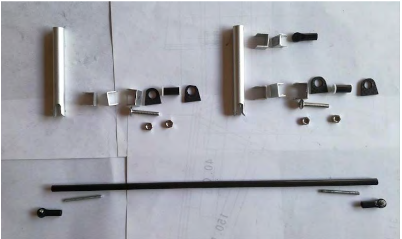
Photo 82: Parts of the gimbal mechanism.
