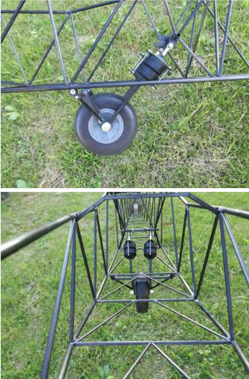
Photo 80: Temporary installation of the main landing gear.
