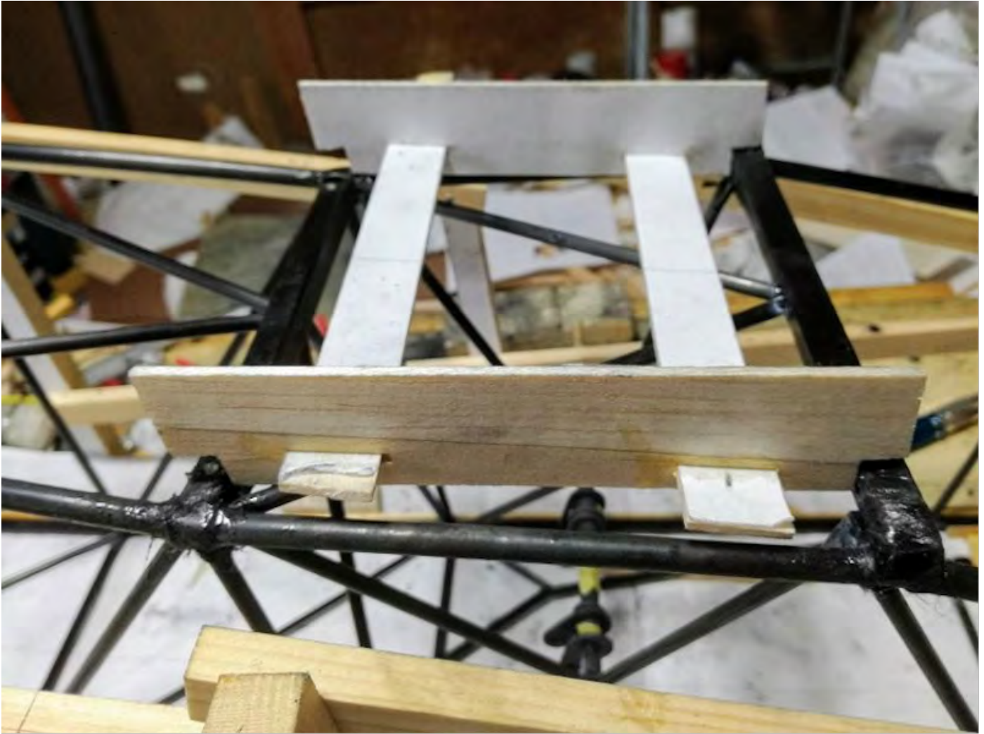
Photo 76: Positioning jig for main wing attachment beams.
