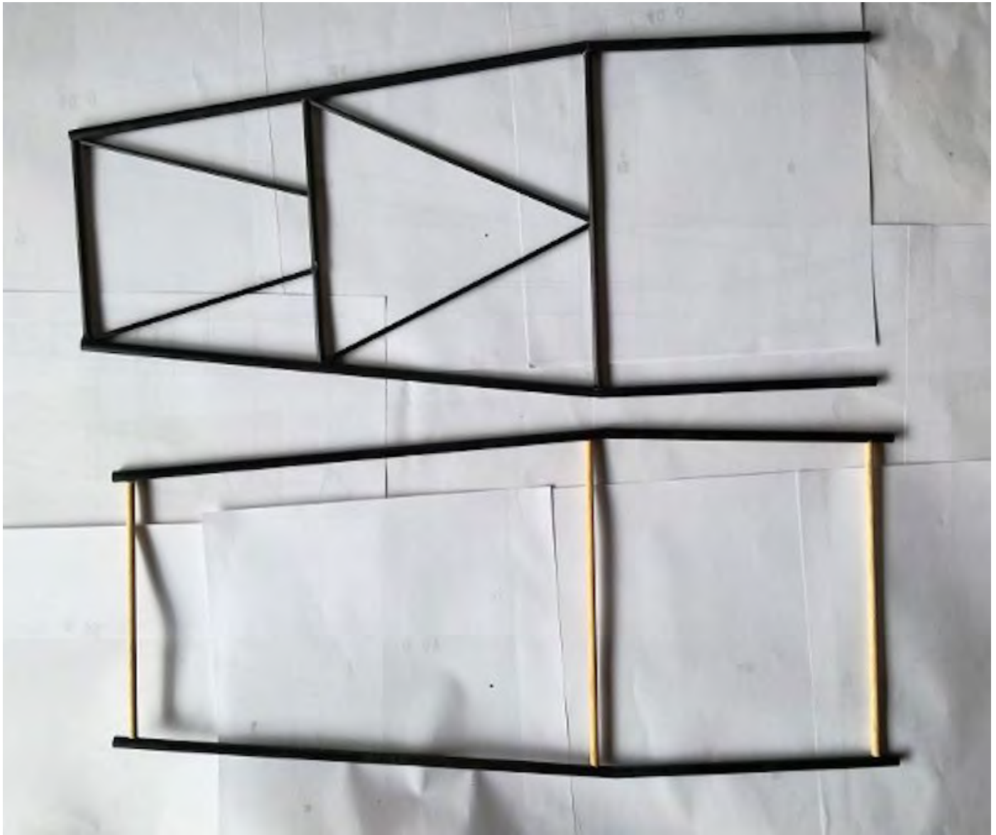
Photo 68: Cockpit floor structure (top) and canopy sill (bottom).
