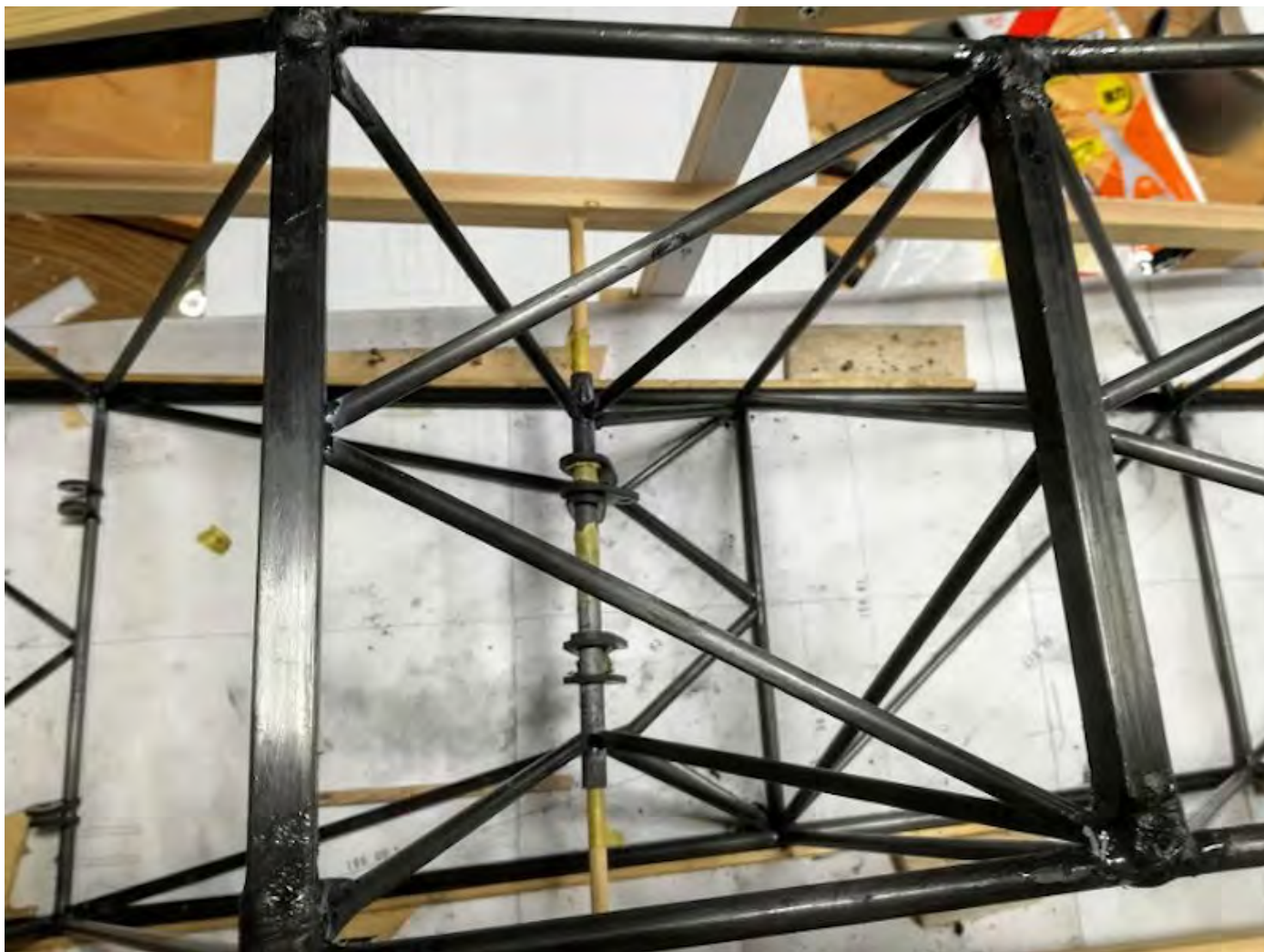
Photo 74: Assembly of the truss structure for the main landing gear.
