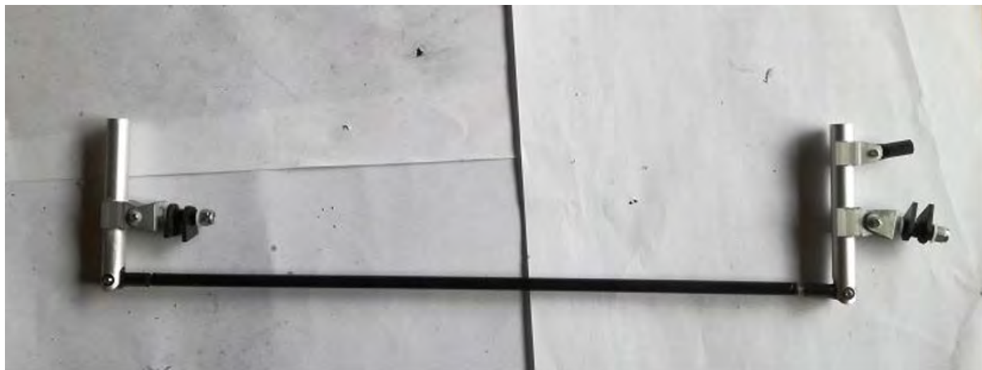
Photo 84: The connected gimbal mechanism.
