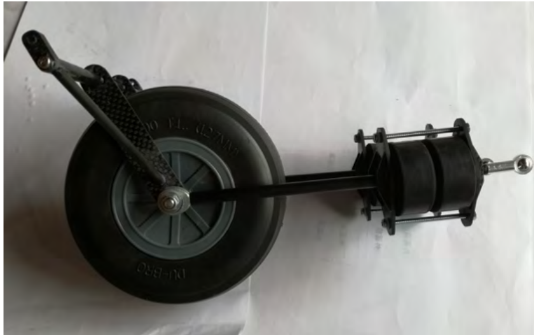
Photo 53: The completed main landing gear assembly
