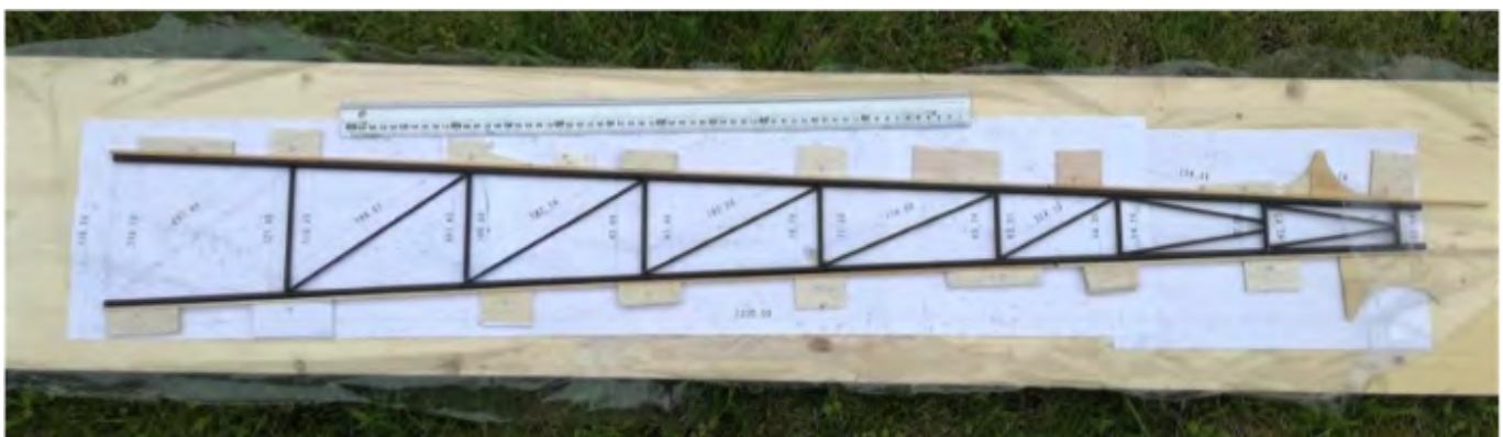
Photo 30: Production of the upper panel of the rear fuselage
