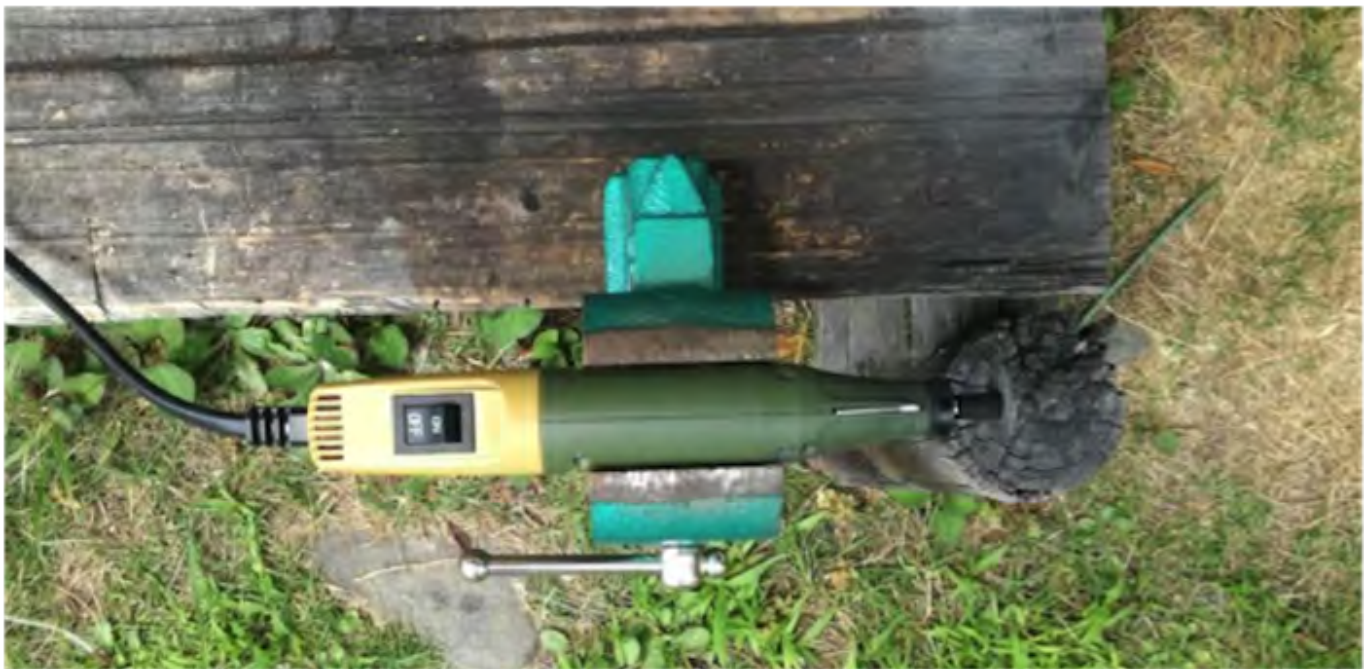
Photo 29: Mini router for cutting carbon pipes
