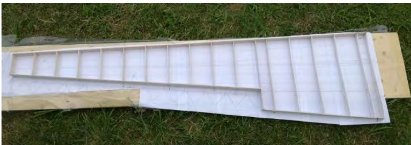
Photo 44: Assembly jig of the left outer wing
