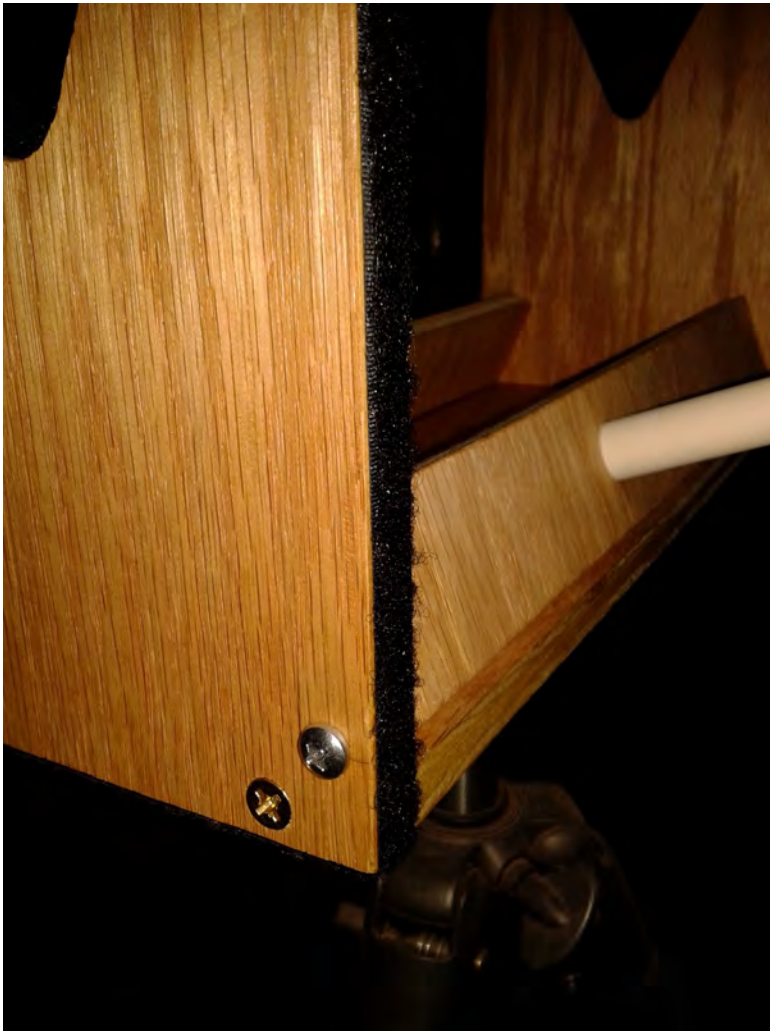
Photo 5 (left): The pan-heads let the side supports adjust and are tightened when you have it positioned where you want it. Photo 6 (right): All the stands have Velcro loop on the ends and use Velcro hook to secure the planes.
