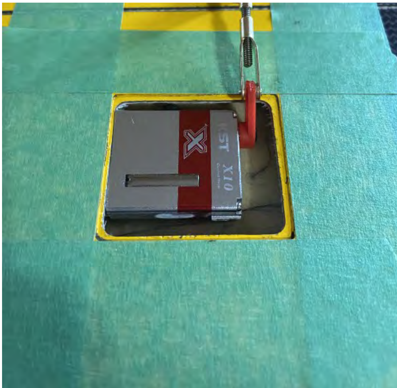
Photo 7: KST X10 servos were used on all surfaces of both planes. (image: Michael Berends)
