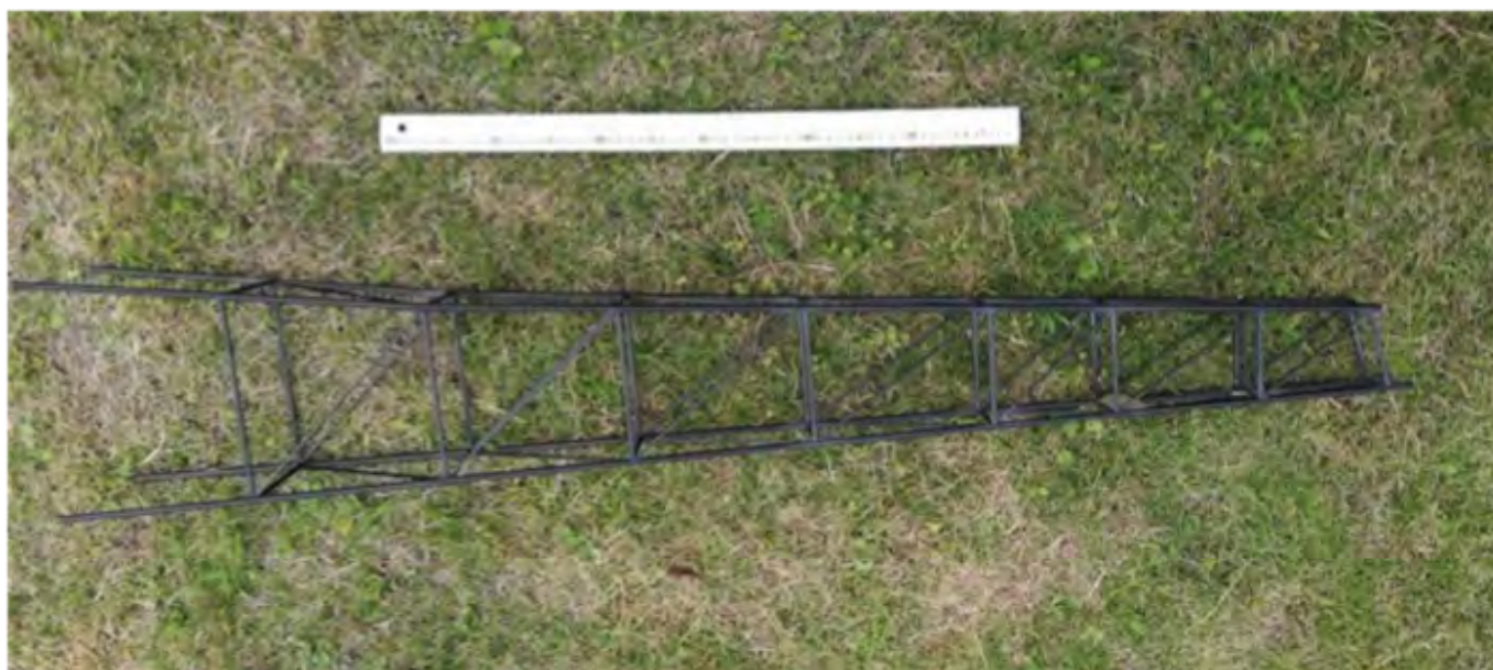
Photo 32: The completed rear fuselage main truss structure
