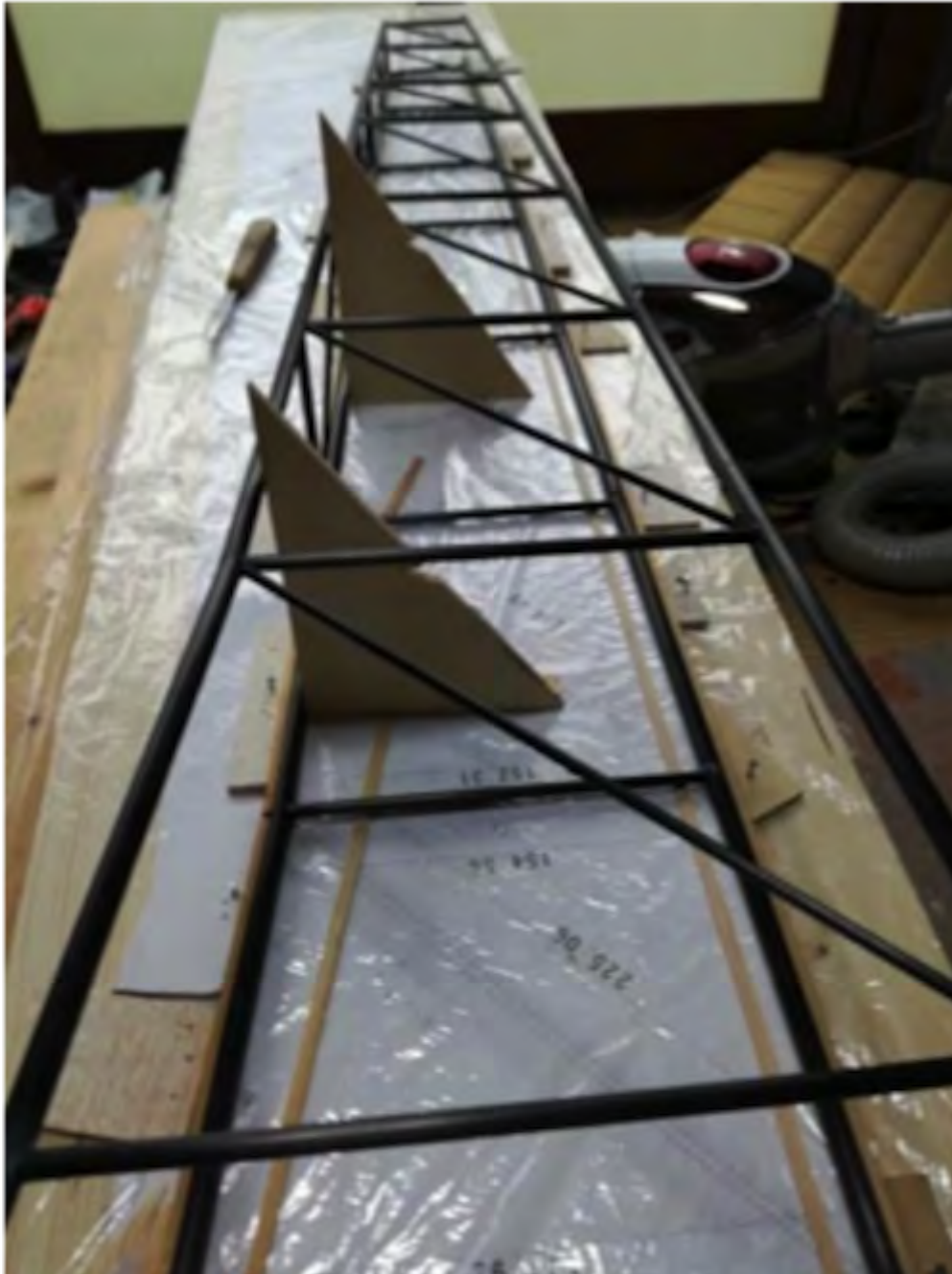
Photo 31: Making the rear fuselage side panels
