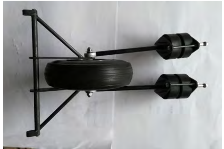
Photo 53: The completed main landing gear assembly
