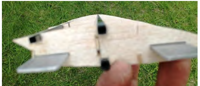
Photo 49: Completed outer wing rib assembly
