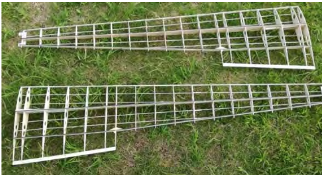
Photo 49: Completed outer wing rib assembly
