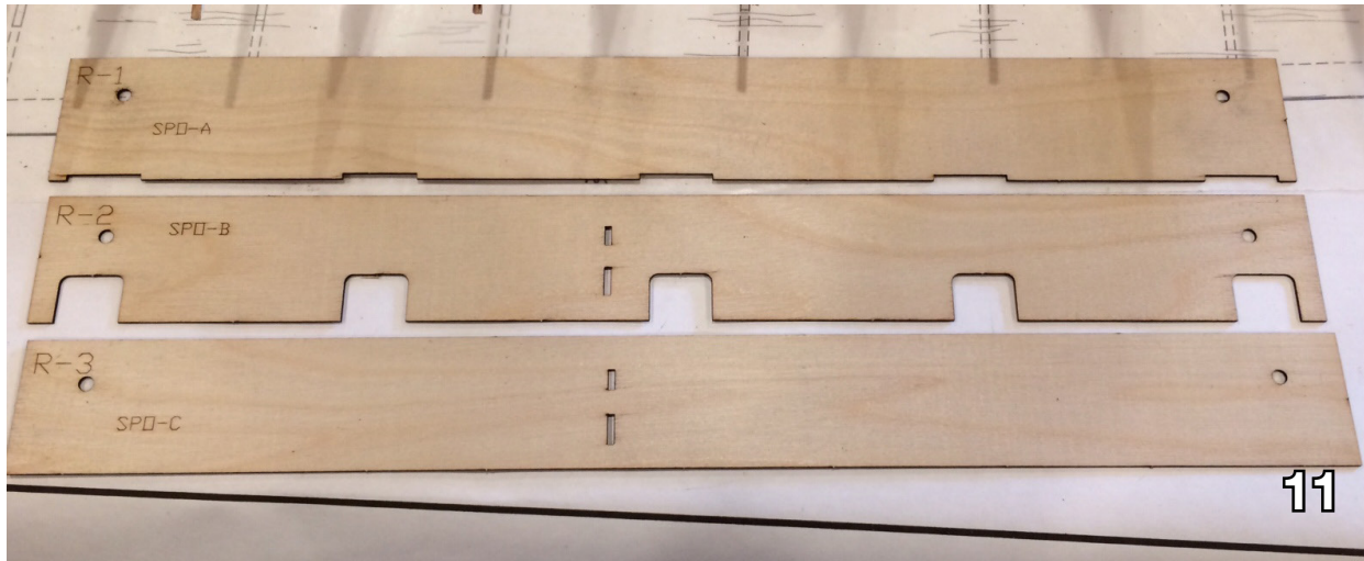
11. Spoiler assembly hinge cutouts, cut with laser.
