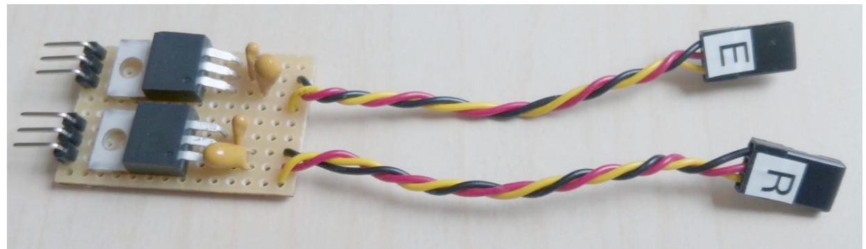
Two LM 2940 regulators on the same board
