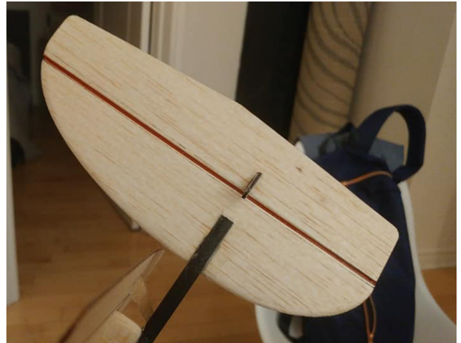
Vertical fin and rudder hinged and mounted.
