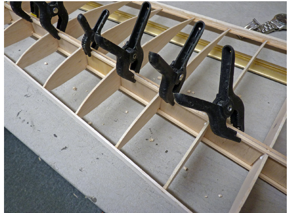
Figure 6. Sub spars added to form H-beam.
