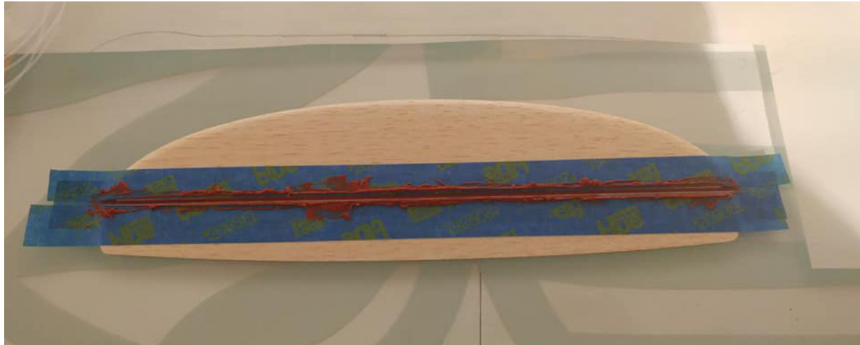
Making the flexible elevator hinge.
