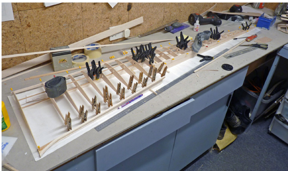
Figure 4. Top spar and a few ply web plates added.
