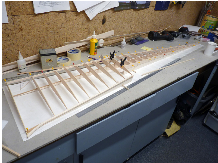
Figure 3. Wing laid up on jigg supports.
