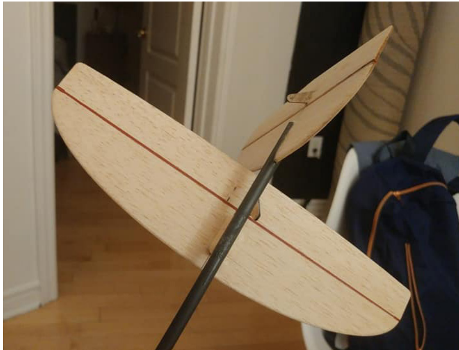
Stabilizer/elevator mounted to boom.
