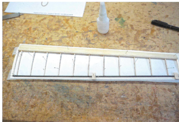
The Swift wing details: a spar and D-box close-up, first, second and third wing panels.
