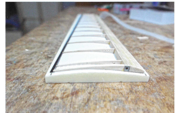
The Swift wing details: a spar and D-box close-up, first, second and third wing panels.
