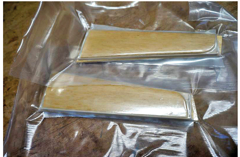
Vacuum bagged wing tips.
