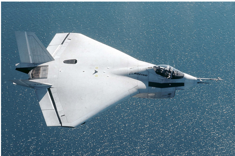
X-32B from above. No leading edge devices, shorter span.
