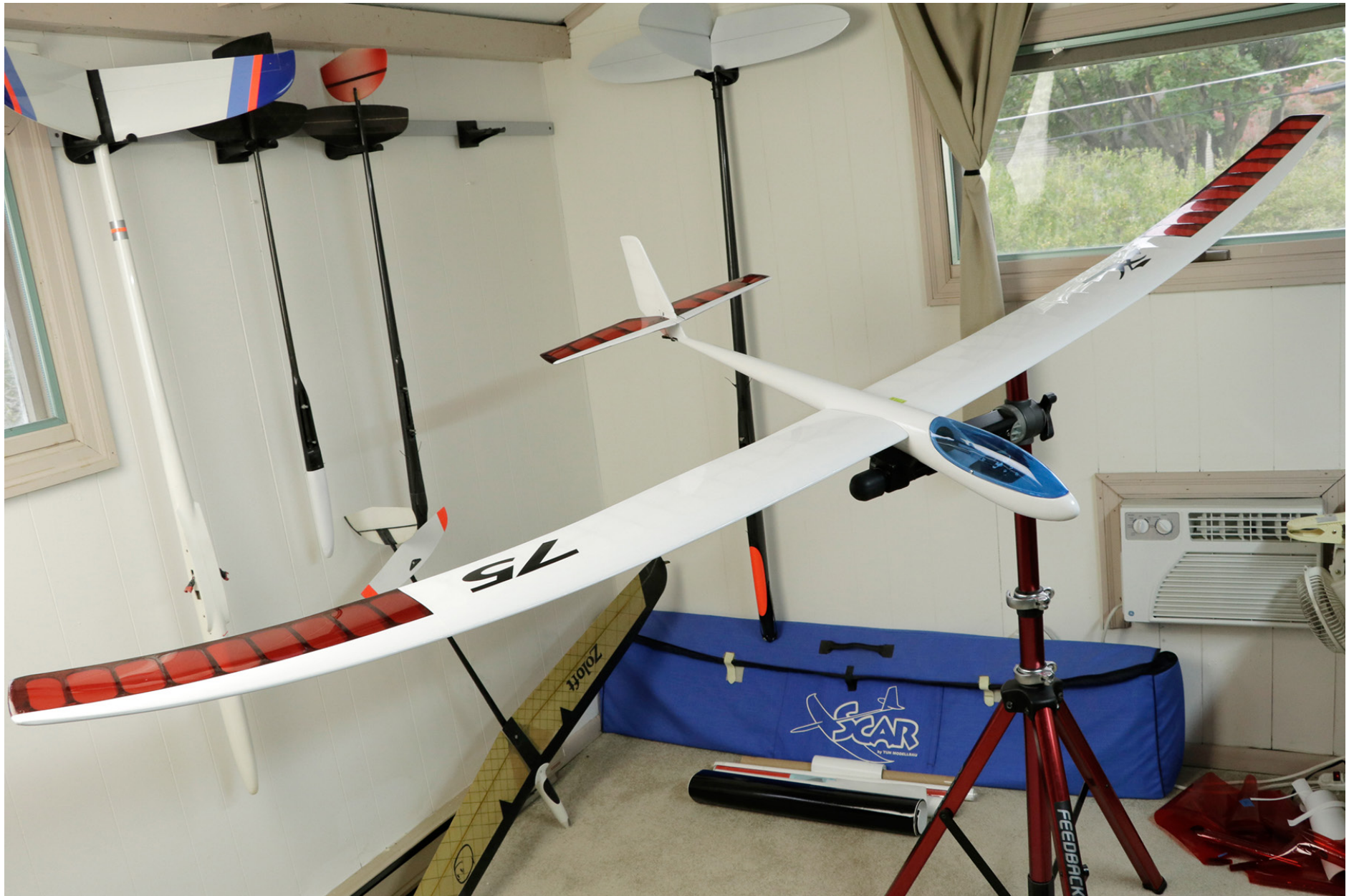
The plane completed and ready for a first test flight. I made the Hobie logo and numbers symbolizing the date of birth in Illustrator and cut out laser printed patterns onto sign vinyl.
