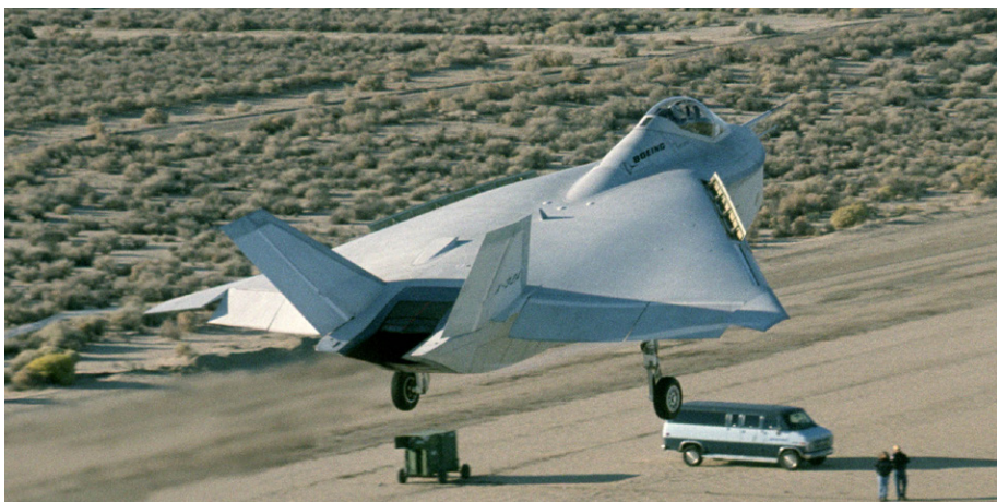
X-32A landing. Leading edge devices include leading edge flaps outboard and leading edge spoilers inboard. Note the contrail coming off the right wing tip in this photo.
