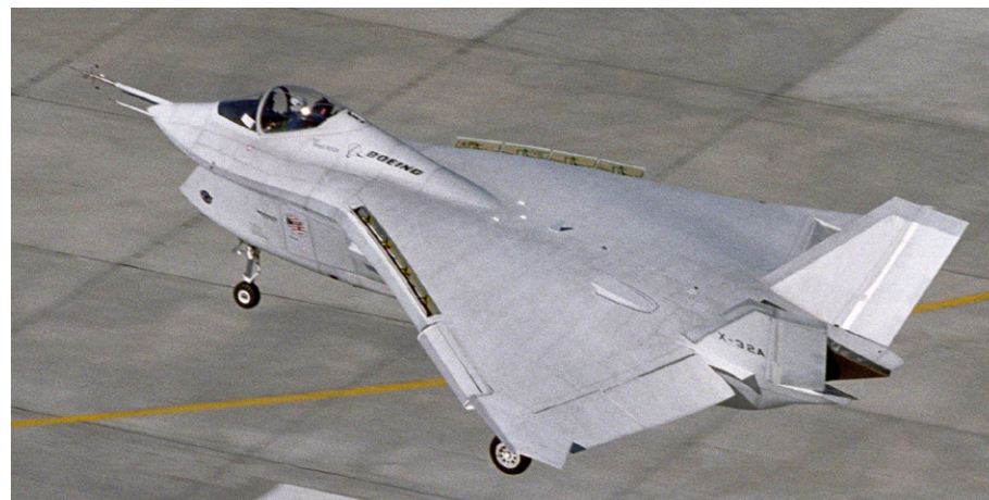
X-32A in landing mode. Leading edge devices include leading edge flaps outboard and leading edge spoilers inboard.
