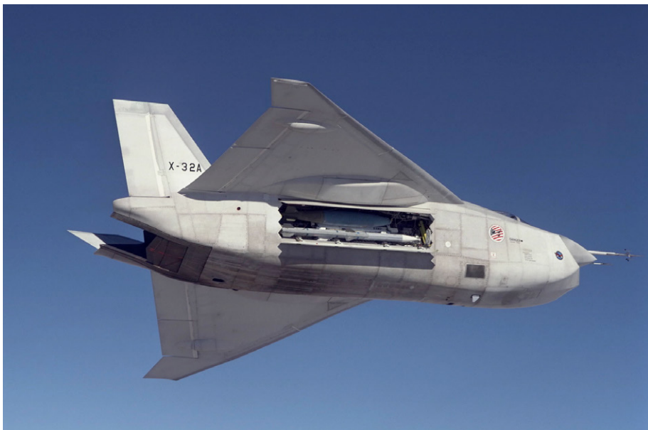
The X-32A with munitions store open.
