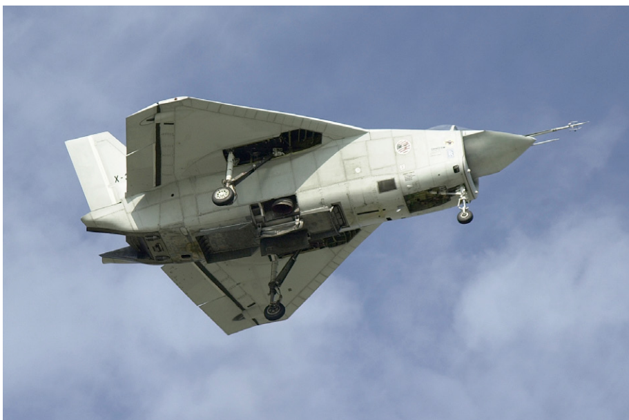
The X-32B while landing. Note shortened wing and VL nozzles.
