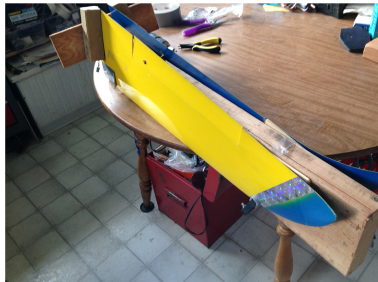
3: Clamping torsion onto Mini Blade wings to increase washout.
