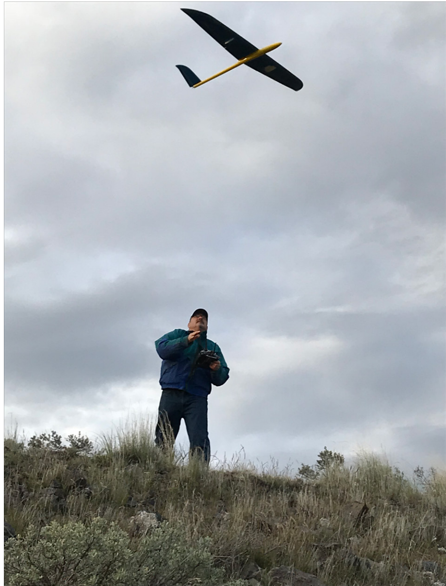
6: With just a couple degrees more washout the tip-stall misbehaviors are corrected. Flies great.
