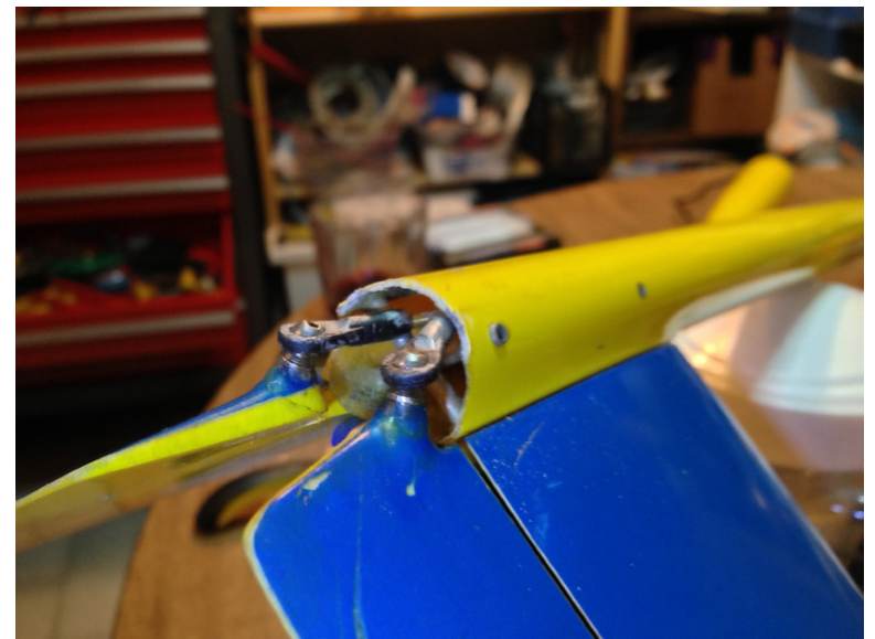
1. The X of V-tail mounting tubes were awkwardly far back, barely allowing space for ball-link connectors.
