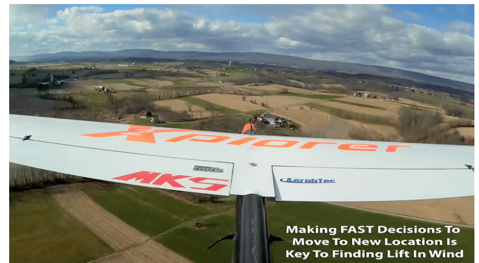
From Thermal Soaring Master Class 2: A tail-mounted camera shows flap position while searching for lift under windy conditions. In addition to verbal commentary, “subtitles” are often used to highlight specific points.
