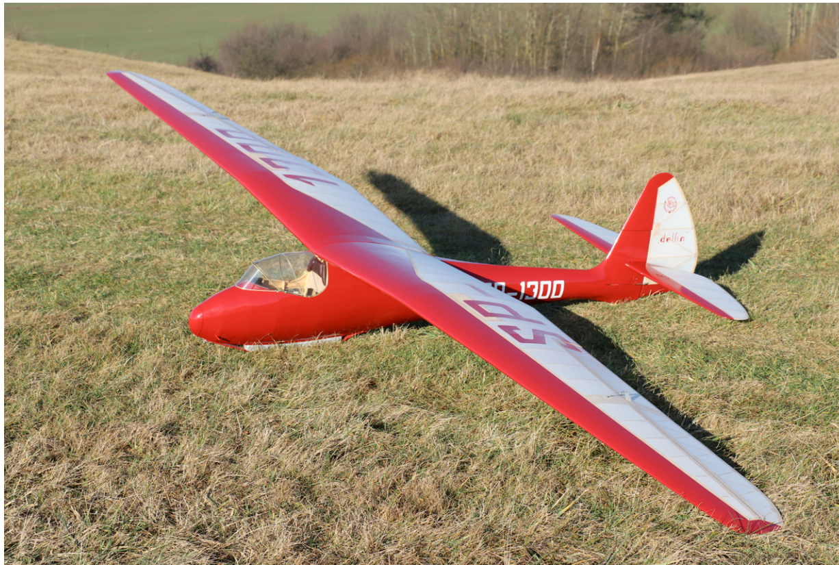
My WWS3 Delfin (Dolphin) model: 4,57 m / 15' span, 7.5 kg / 16.5 lbs. weight, NACA 4415-4409 airfoils
