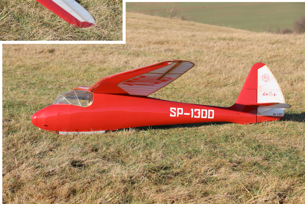
My WWS3 Delfin (Dolphin) model: 4,57 m / 15' span, 7.5 kg / 16.5 lbs. weight, NACA 4415-4409 airfoils
