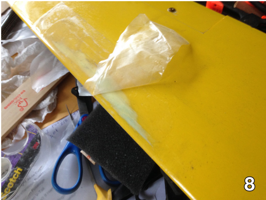
Image 8: Peeling the tape off the glass. The spackle smoothed the wing to nearly its original shape.
