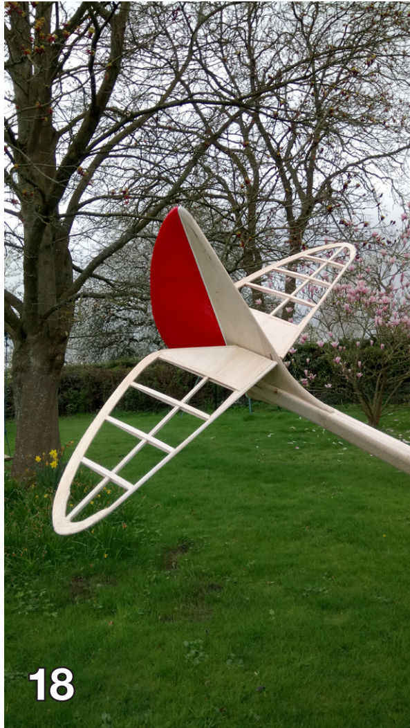
(18) All moving tailplane and rudder are similar built-up construction.
