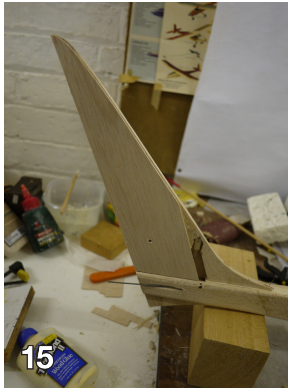
15 Once satisfied with the bellcrank alignment the vertical stabiliser can be sheeted in.
