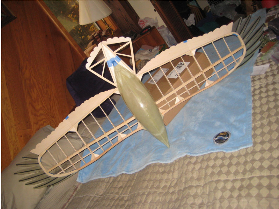
Bottom view of the balsa rib prototype.
