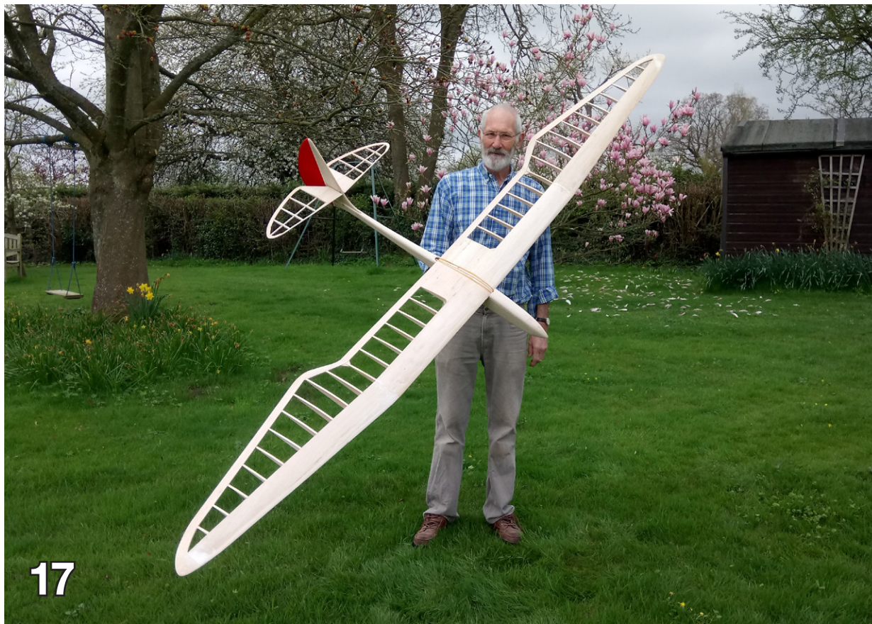
(17) Main parts ready for covering, except rudder which has already been covered.
