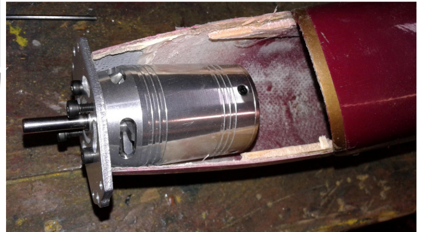
The HK Gliderdrive undergoing installation.
