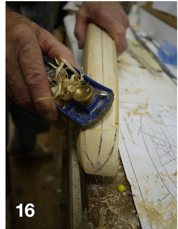
16 Fuselage is shaped using razor plane before final sanding, note we marked centre and outline shape lines for guidance.
