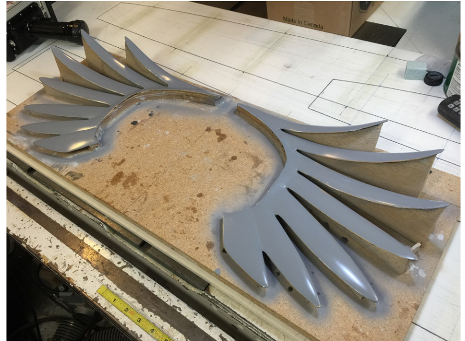
Molds for the tip feathers. Each feather is at a different angle.
