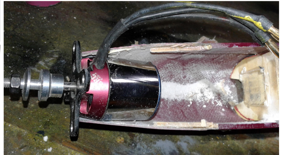
Fitting the eFlite Carbon Cub motor.
