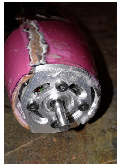
Motor mounted and nose wrapped with \frac{3}{4} oz. 'glass.
