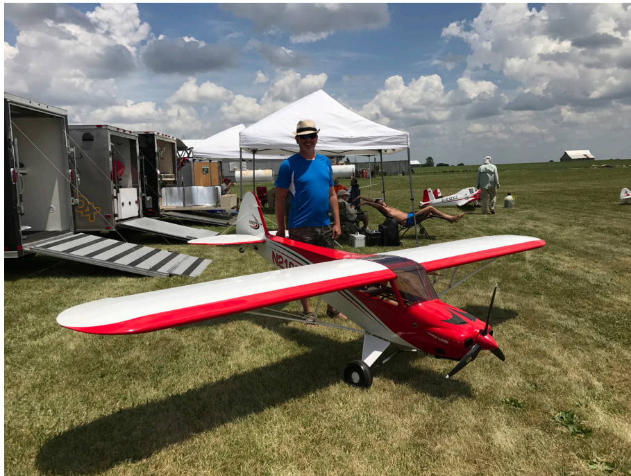
Peter George with his Aeroworks Carbon Cub powered with a DA-150, three blade prop and cans. Very quiet setup.
