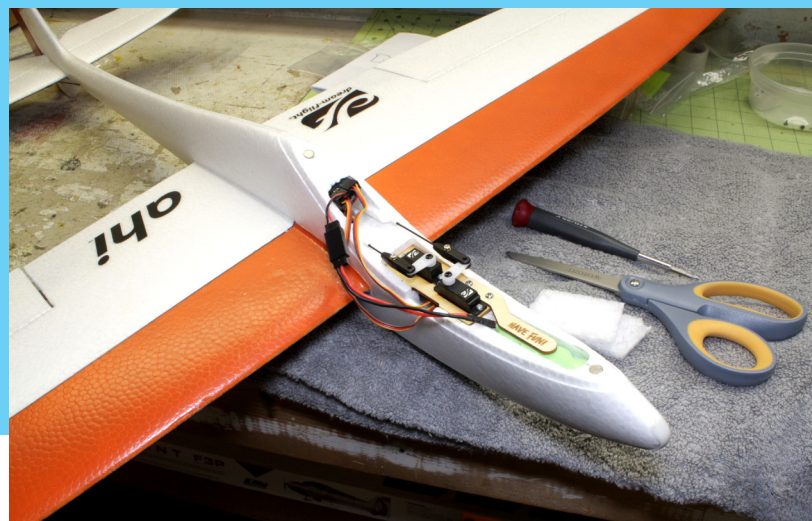
View showing the installed rudder and elevator servos, battery pack and battery hold-down.
