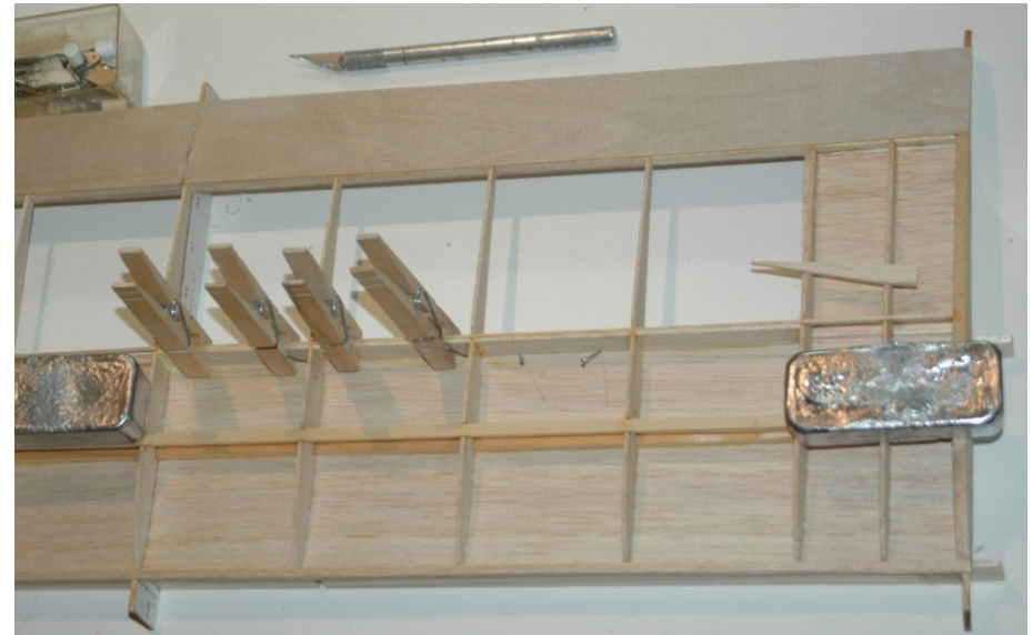
Figure W10: Installing shear webs at the back of the D-box
