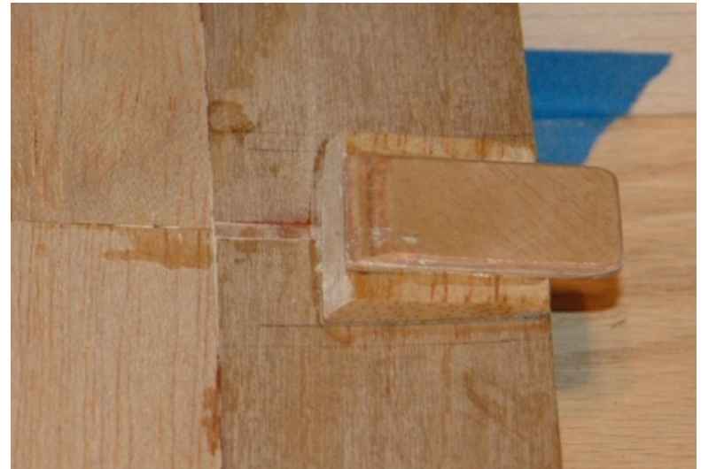
Figure F8: Rear wing mount tab
