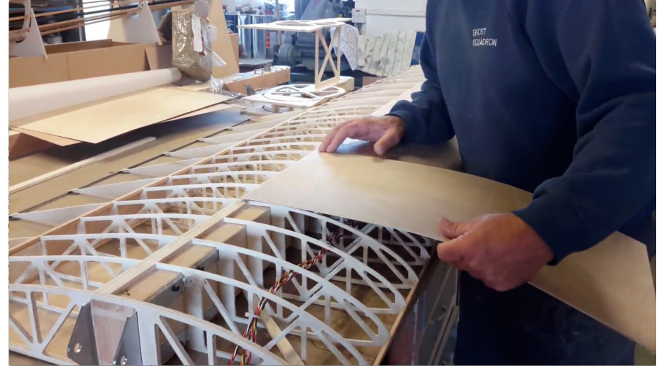
3 - Fixing the plywood to the top of the wing
