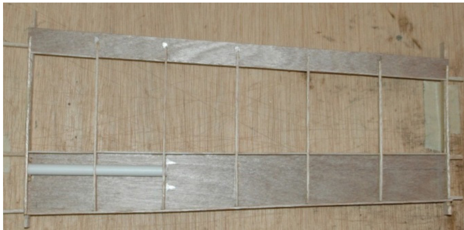
Figure T2: Tail frame ready to install control horn and top D-box skin.
