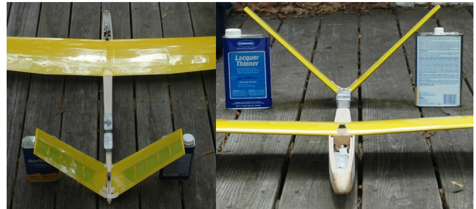
Figure F12: Gluing the tail pivot tubes to the fuselage
