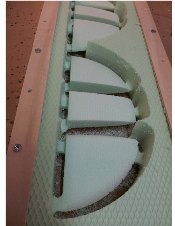
Wings finishing is milled three-dimensionally from Styrodur
