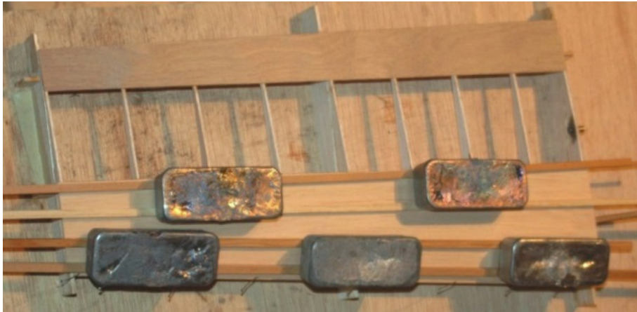
Figure W15: Clamping the top D-box skin in place
