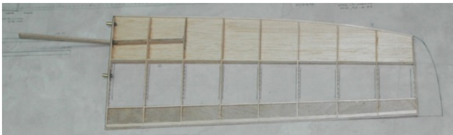
Figure W23: Tip panel frame ready for top D-box and trailing edge skins
