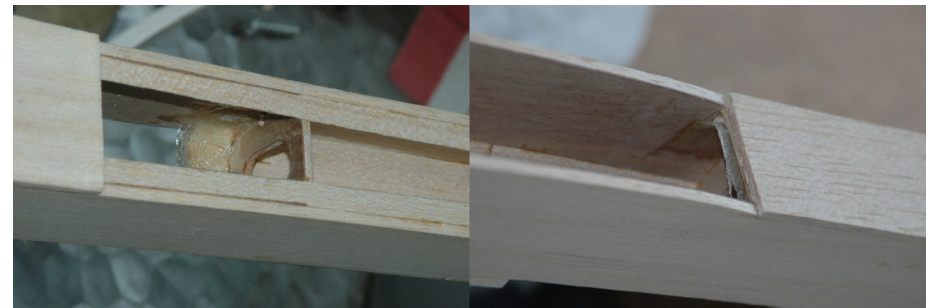
Figure F6: Applying fiberglass to the rear wing mount
