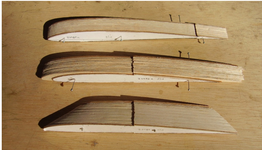
Figure W3: Wing rib stacks between master ribs
