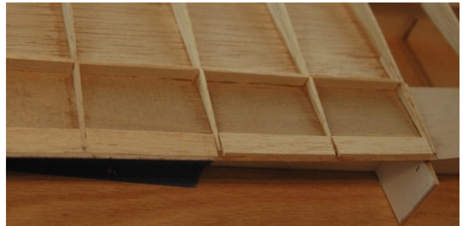
Figure W8: Trailing edge reinforcement — wedges on the left are shaped, on the right are as installed
