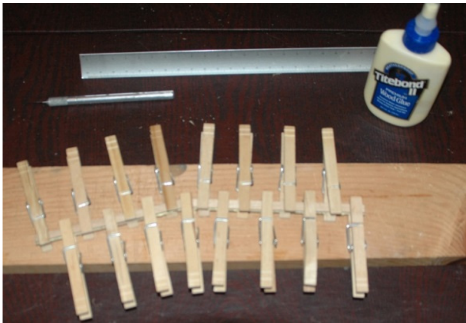
Figure W1: Laminating the tip joiner
