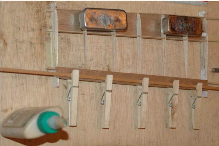
Figure T5: Closing the stab trailing edge
