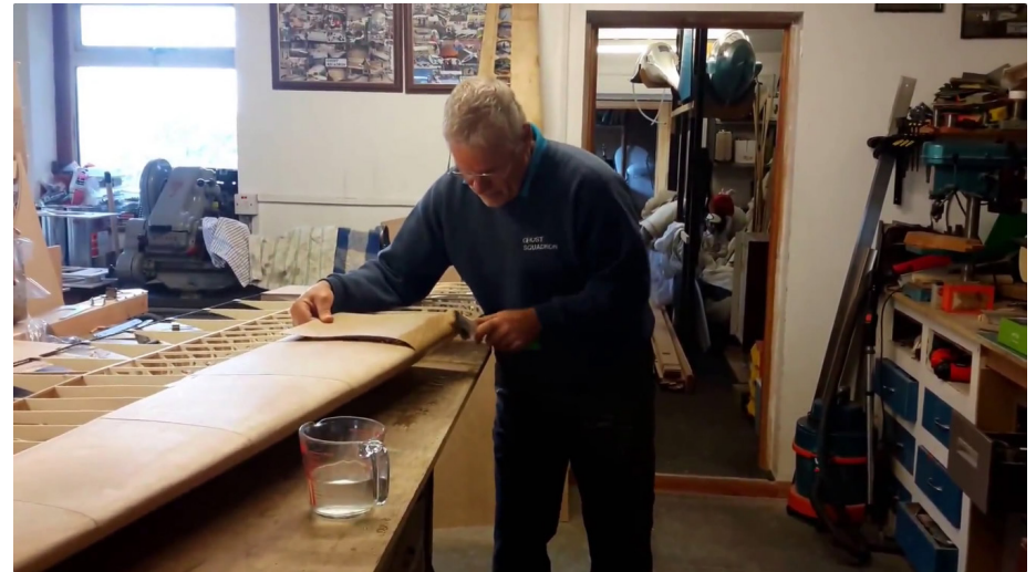
5 - Bending the panel around the Leading Edge and fixing the sheet to the underside
