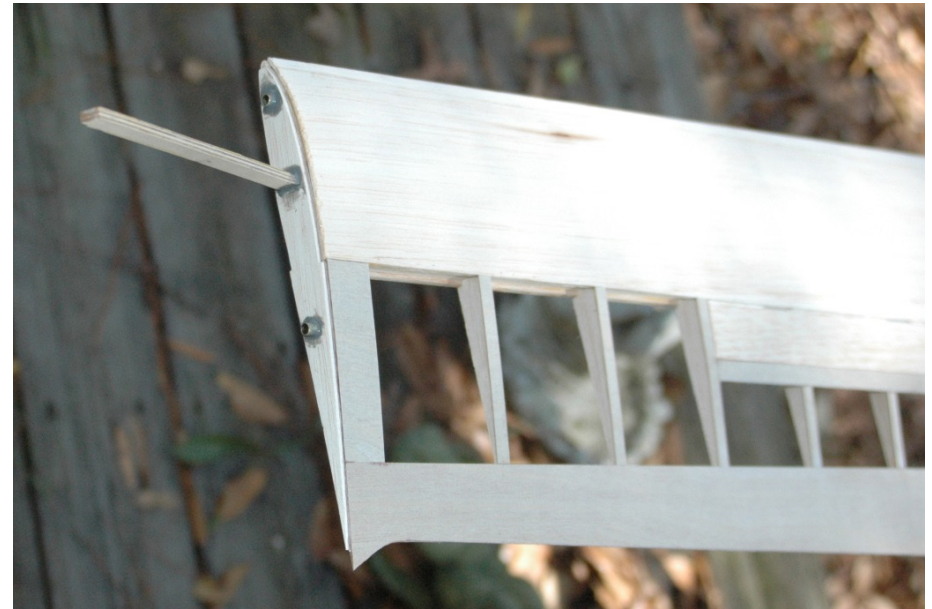
Figure W16: Assembling the tip joiner, first tip rib and guide pins
