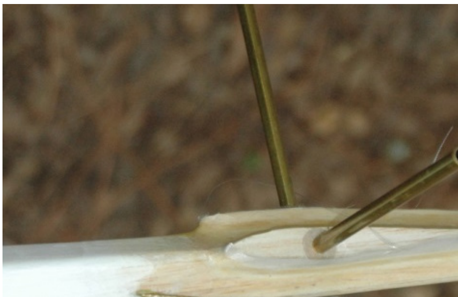
Figure F14: Tail Fairing Final Shaping and Glassing
