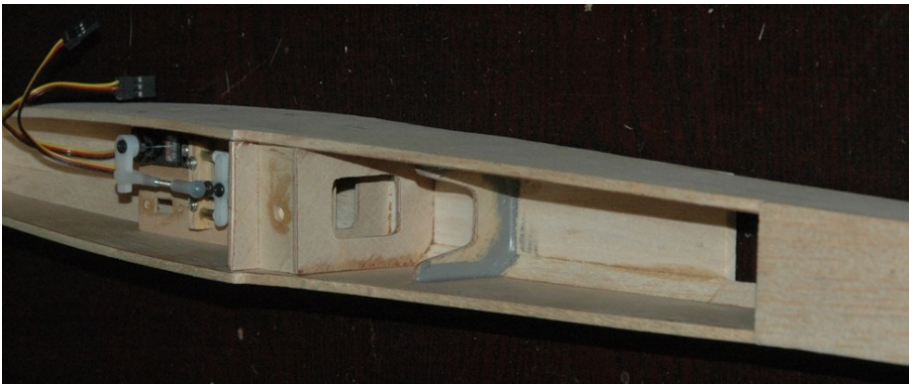
Figure F5: Mid-fuselage bulkhead installation
