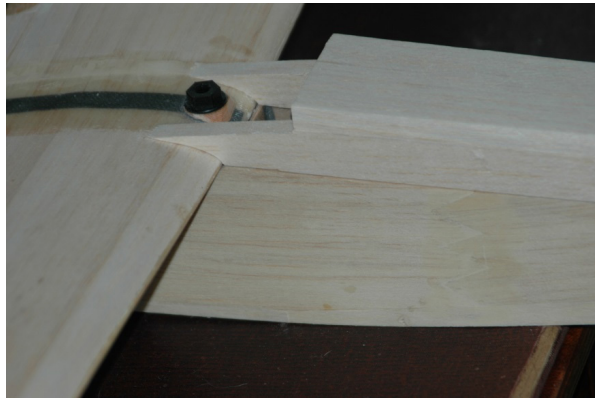
Figure F16: Fitting hatch cover to wing
