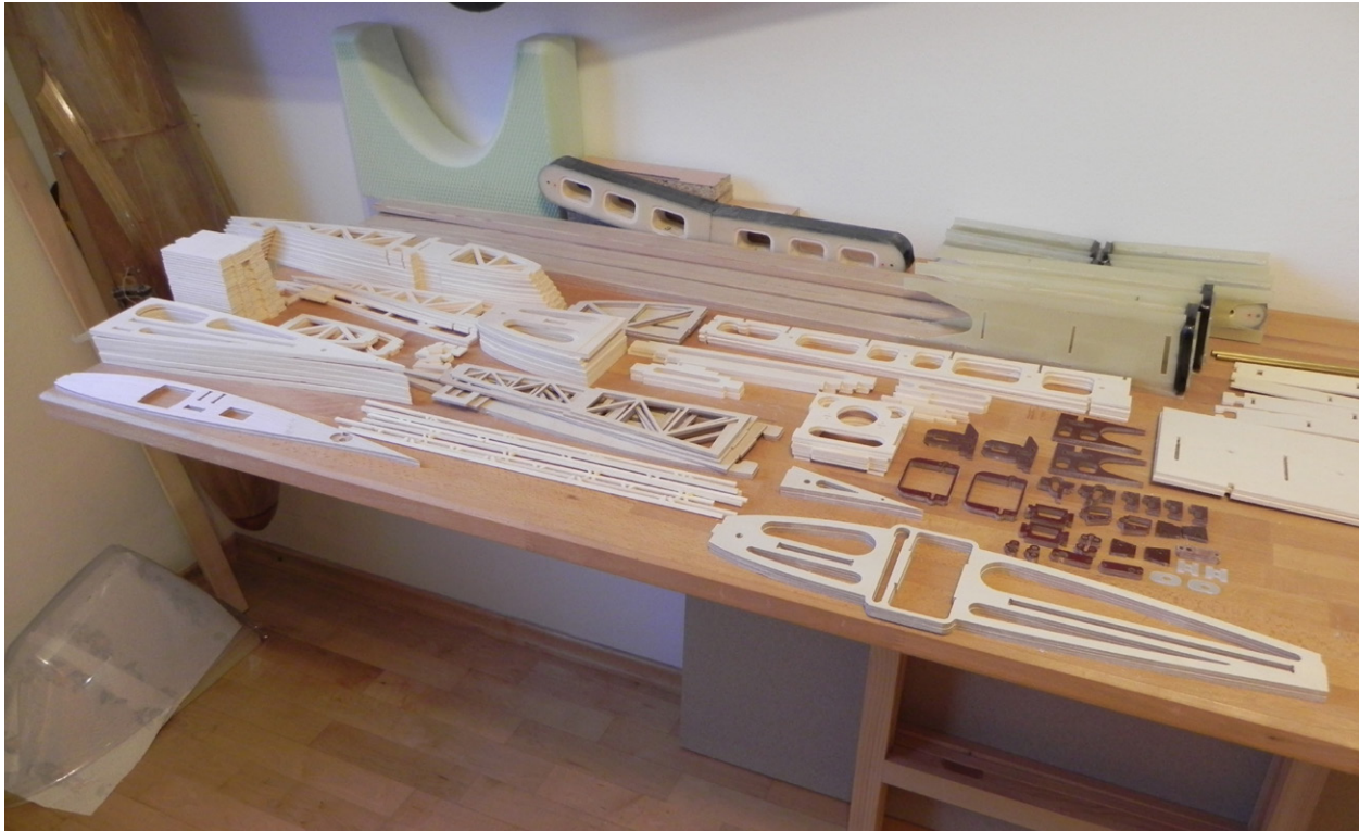
Parts of the wing with bayonets and their bushings
