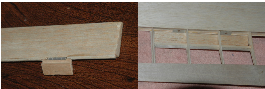
Figure W19: Spoiler installation details
