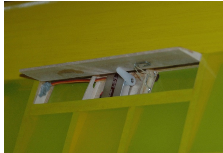
Figure W20: Installed spoiler with rubber band closing spring. Note that the servo wire is sealed with RTV where it enters the spoiler box.
