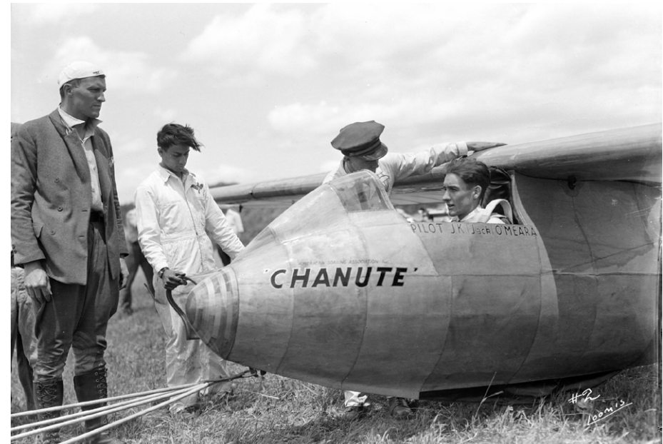
Below right: (1932) Note the change of the forward fuselage contour compared with the D-17. The Chanute sported an enclosed cockpit. Loomis, NSM.
