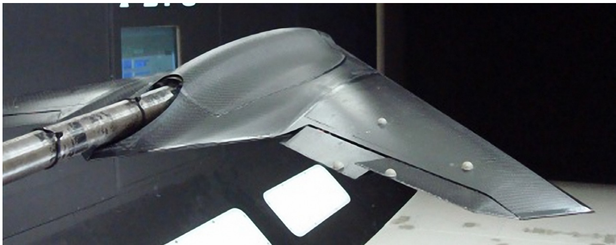
Wind tunnel model displaying a differential flap deflection.
