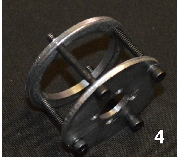
Completed motor mount.
