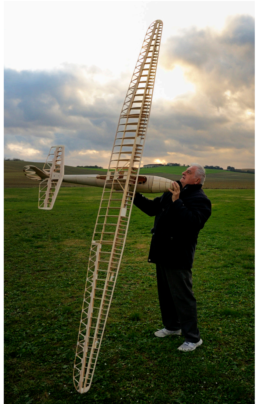
Completed skeleton ready for covering.
