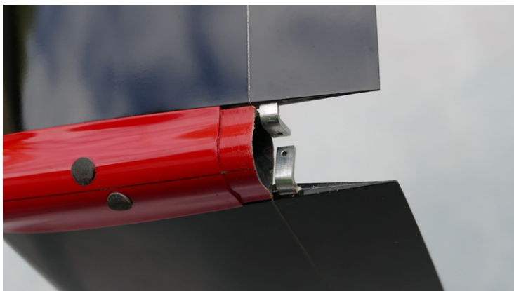
Above: The tails in place with the unusual control horns going up
