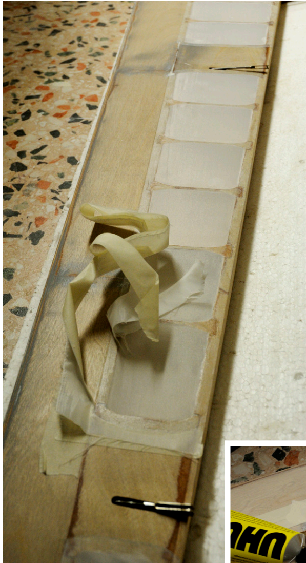
Covering the wing and horizontal tail
