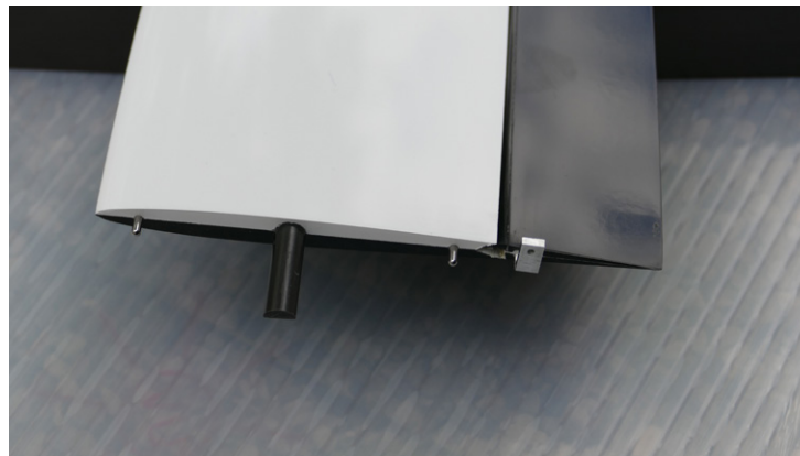
The tail root with joiner and aluminium horn
