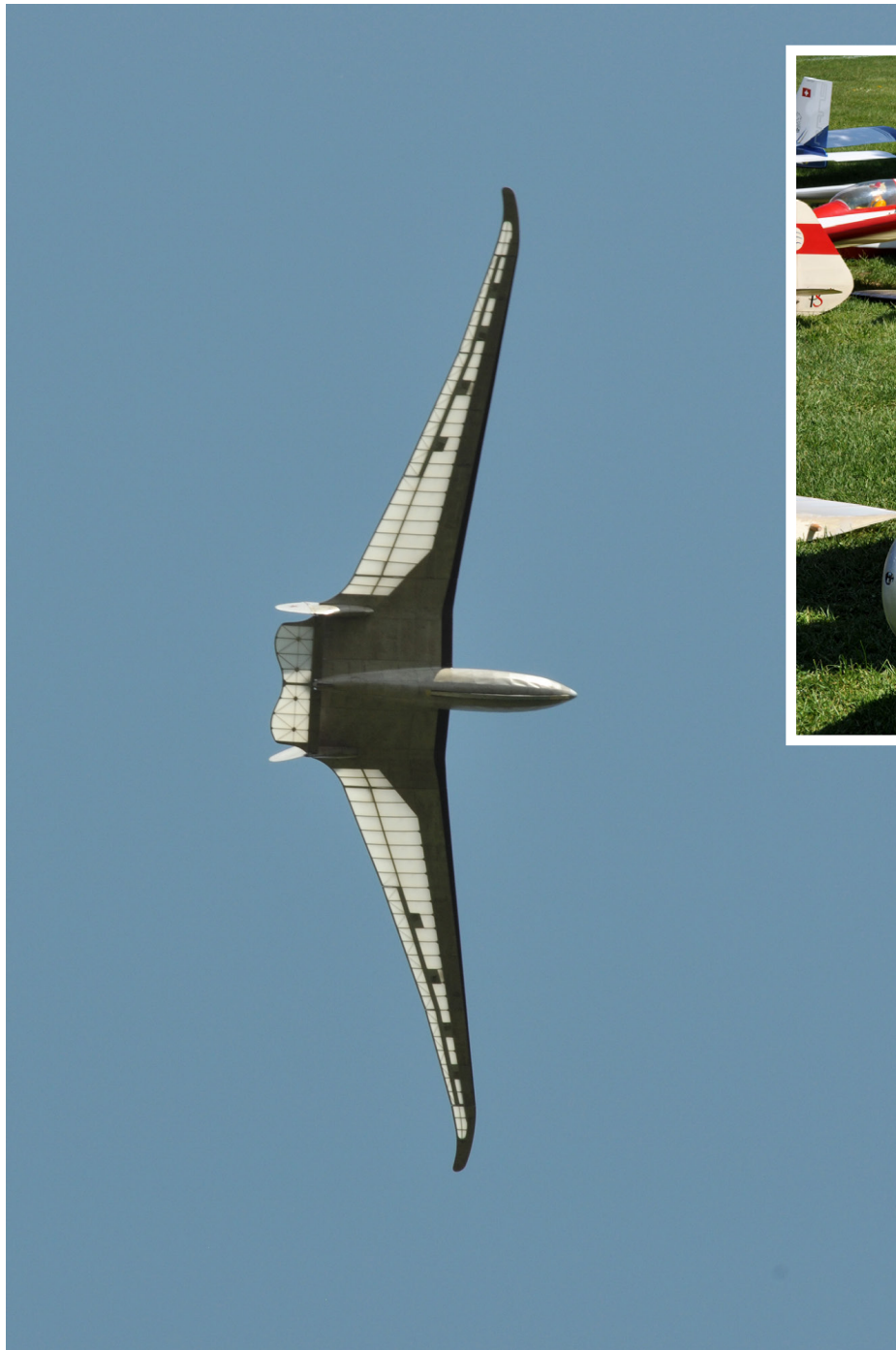
Left: The half scale Beljajev BP3 in flight. The BP3 is making a left turn in the photo; notice the inboard rudder is deflected in the direction of the turn while the outboard rudder remains in neutral. This is similar to the control action of the Fauvel series. Above: Builder Markus Frey getting the Beljajev BP3 for flight.
