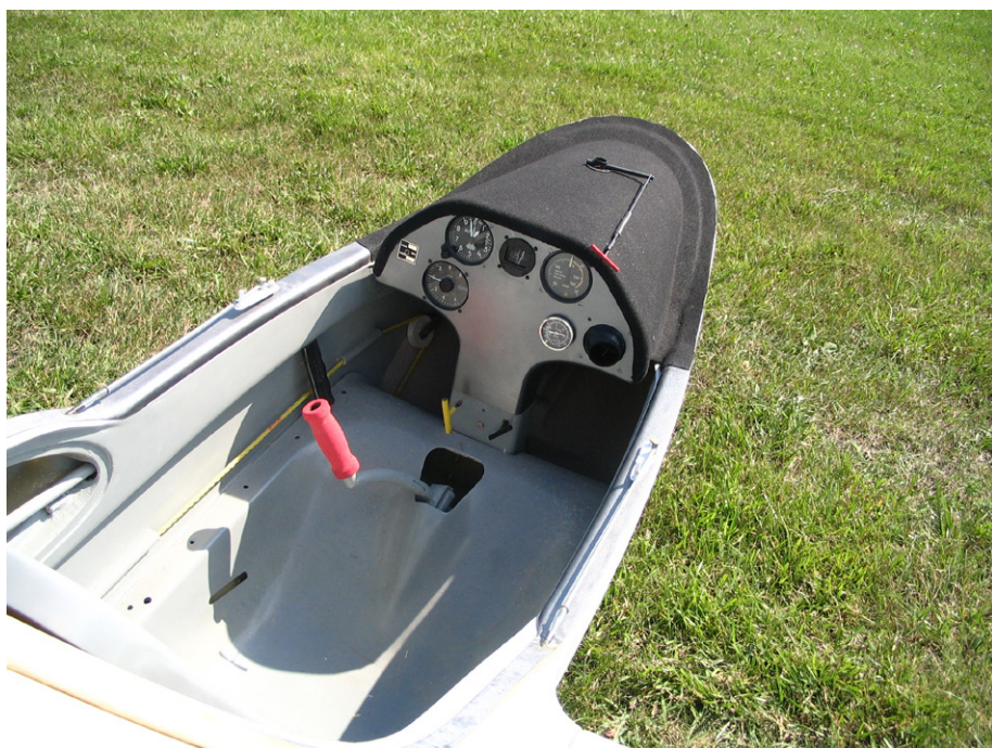
Left above and left: Cockpit interior. The small wheel on the left side cockpit wall moves a weight fore and aft for high speed and low speed CG trim. Above top: Jim and the Pioneer III. Above: Flying field assembly.
