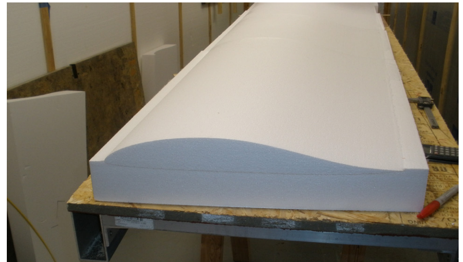
Upper: Wing "guts." Aileron cutout at rear, composite spar in place, elevator cutout at forefront. Above: Wing tip core.
