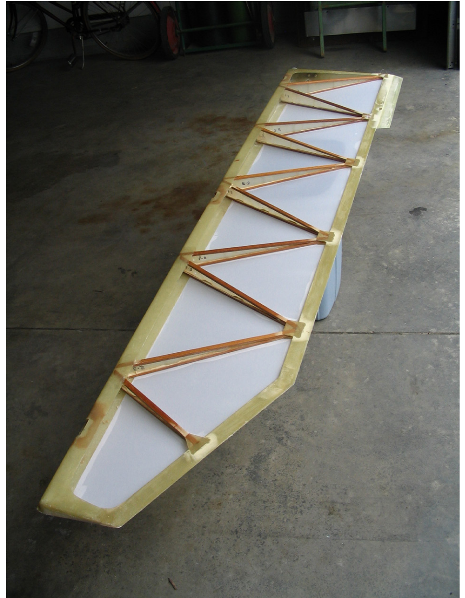
Above left: Interior details of the wing showing the aileron control system. Left: Open spoiler. Note the composite rib structure. Above: Elevator under construction.
