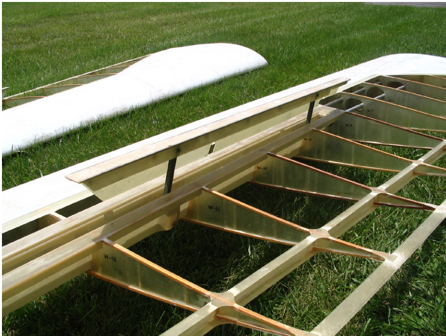
Above left: Interior details of the wing showing the aileron control system. Left: Open spoiler. Note the composite rib structure. Above: Elevator under construction.
