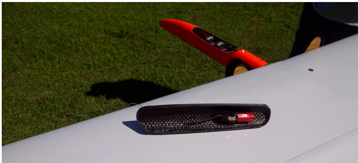
The batteries are taped in and the transmitter is Velcroed to the inside of this Supra's canopy with the antenna wire coming out the top. This configuration has, surprisingly, survived many a hard "landing" without separating from the sailplane or coming apart.
