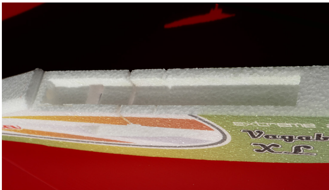
The fuselage with the radio compartment already done
