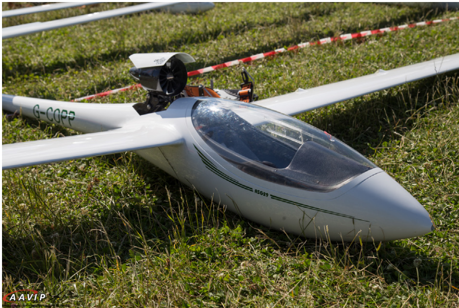
This page and opposite: This scale ASG 29/18m featured a Schubeler ceflix 500 retractable EDF self launch system
