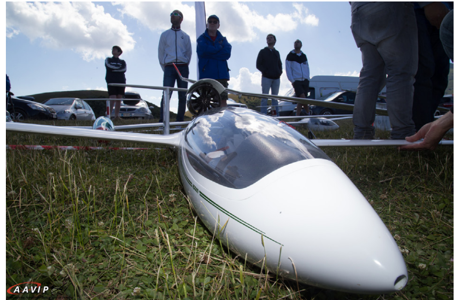
This page and opposite: This scale ASG 29/18m featured a Schubeler ceflix 500 retractable EDF self launch system
