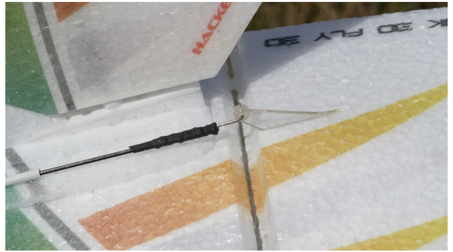
Close picture on the rudder control horn and rod end
