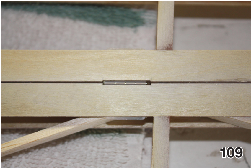
109. Hinge dry fit showing relief in wing and aileron for the center of the hinge.
