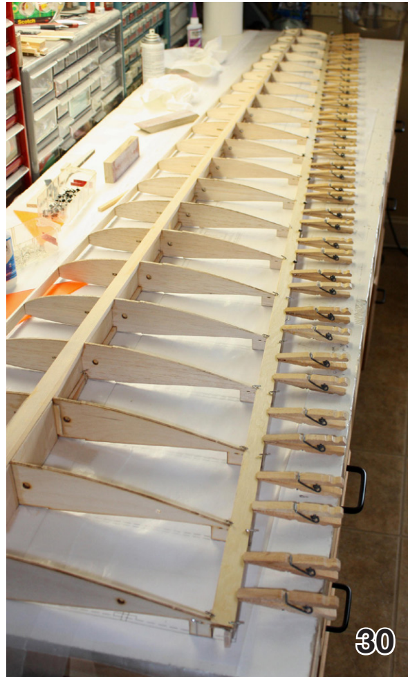
30. This photo shows the entire trailing edge glued up and being held in place with pins and clamps.
