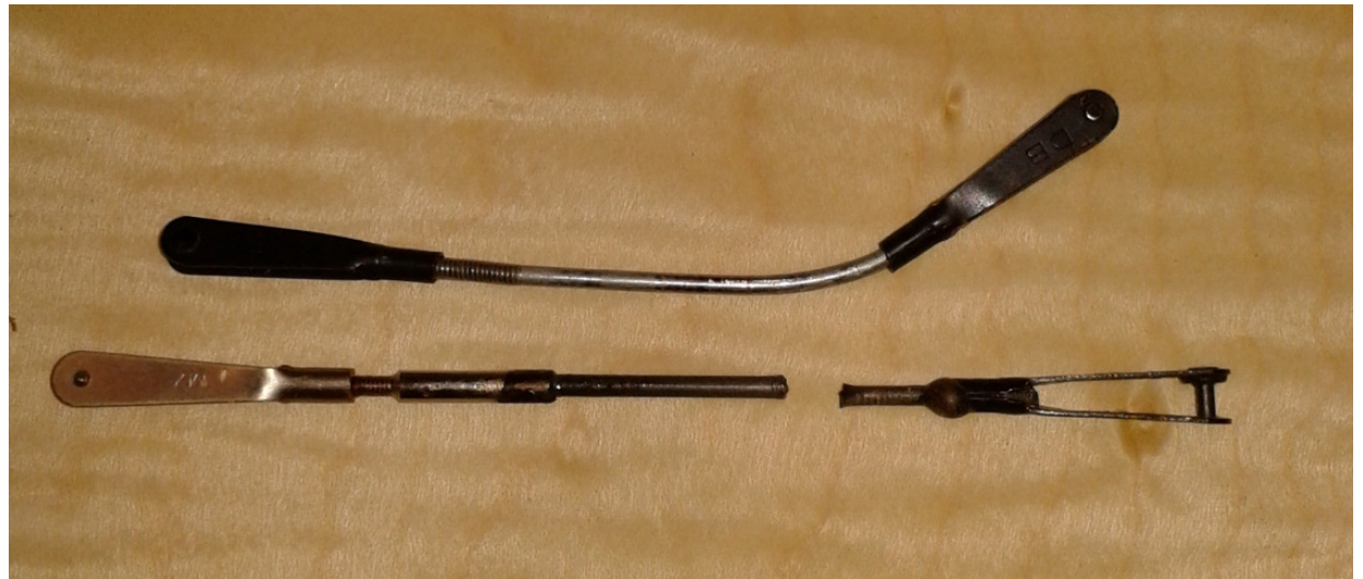
Bent and broken clevis rods.
