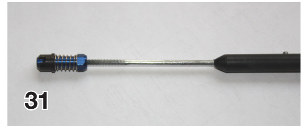
31. The Sullivan S591 4-40 aluminum ball connector at the elevator end.
