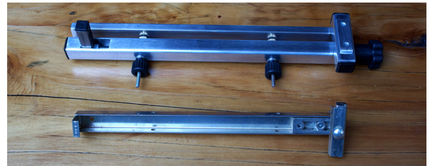
Bill Wilson's rip fence compared with the supplied Dremel product.
