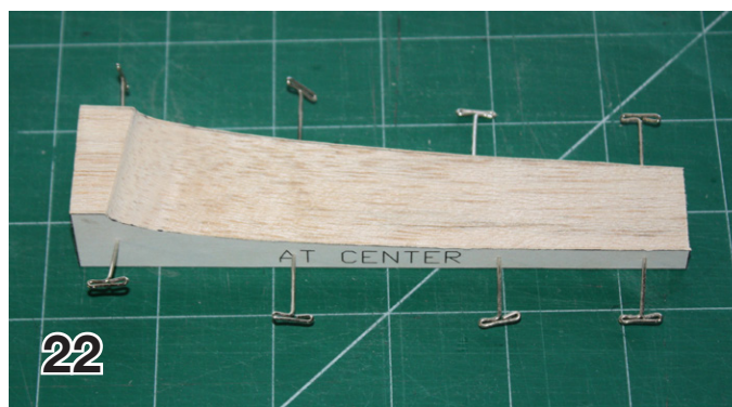
22. Finished right side stabilizer mount.
