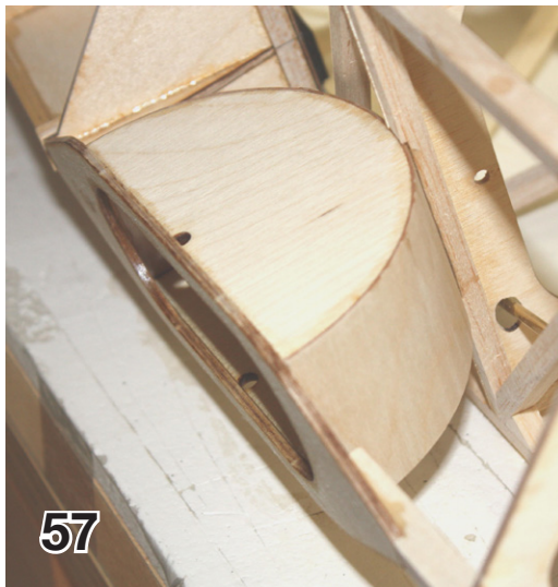
57. View of top of wheel well glued to fuselage former F6.
