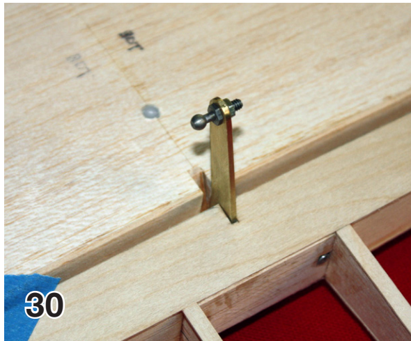
31. The Sullivan S591 4-40 aluminum ball connector at the elevator end.
