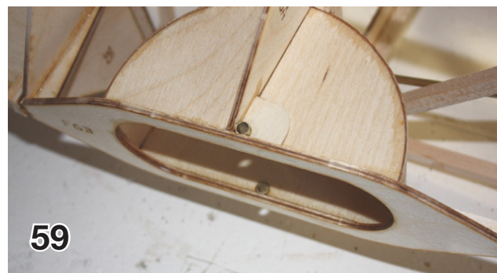
57. View of top of wheel well glued to fuselage former F6.
