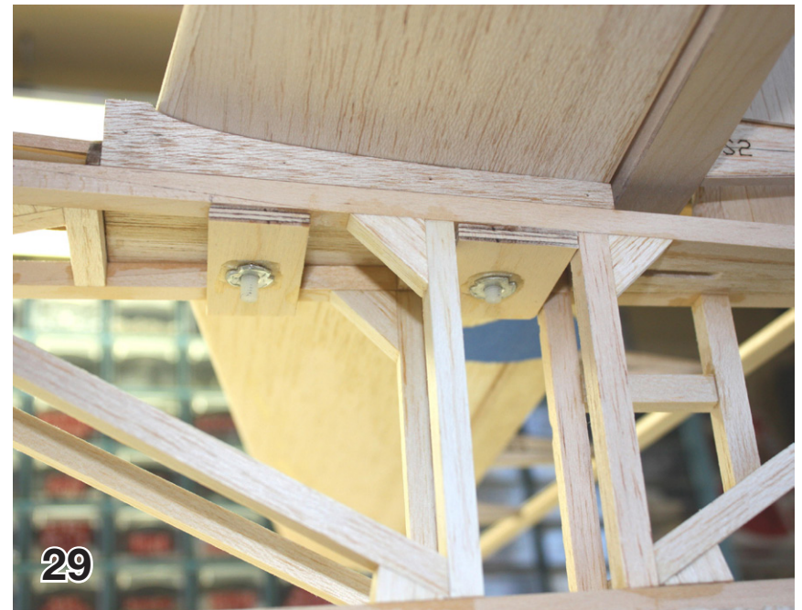
29. View of mounted stabilizer from below.
