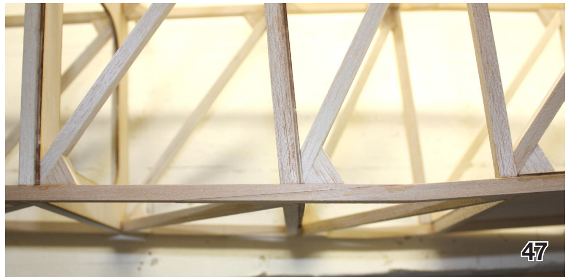
47. View of the right side of the fuselage. The cockpit floor assembly excess longeron length has been trimmed off at the scarf joint.
