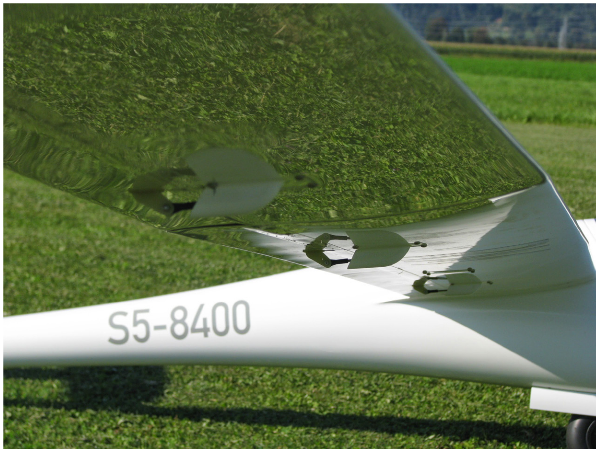
The drives on the control surfaces are in the classical version. Of course, it is possible to build in the RDS connections on the wings and wing flaps.
