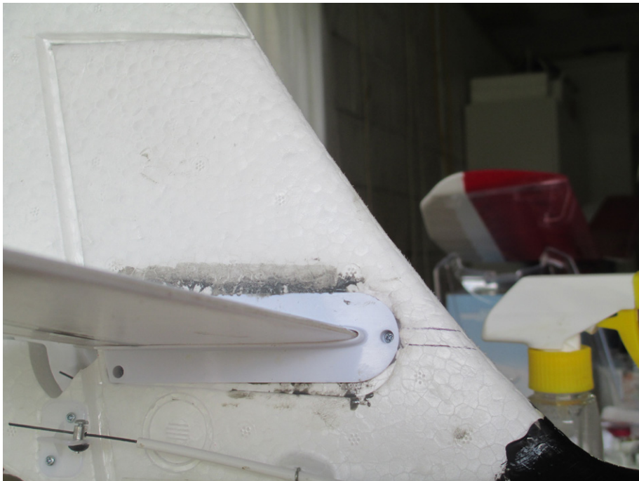
Adjustment to horizontal tail mounting angle to achieve recommended decalage.
