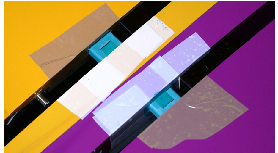
The risky step of the gluing of the green connectors in the wing root. I used PVA release agent everywhere it was needed, in addition to some thin tape to protect the fuselage and the root of the wing.
