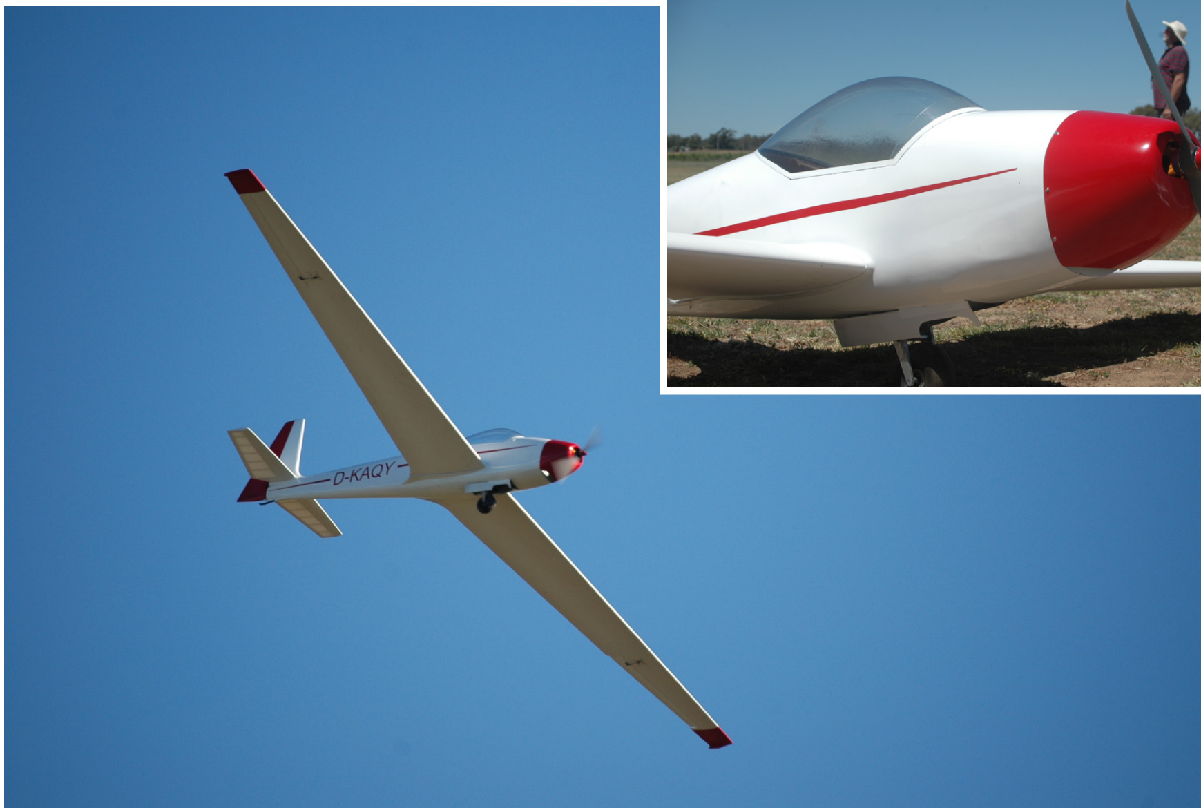
Pilot: Neil Spencer and co-builders Henryk Kobylanski, Shane Williams and Andy Smith, Airframe: scratch-built ASK14 5m, HQ3014 airfoil, 6364 motor with 18x12 prop on 10s
