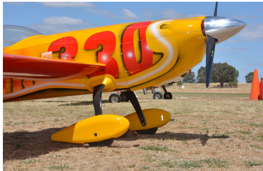
Pilot: Simon Bishop, Airframe: 2.6m Comp Arf Extra 330sc with DA120
