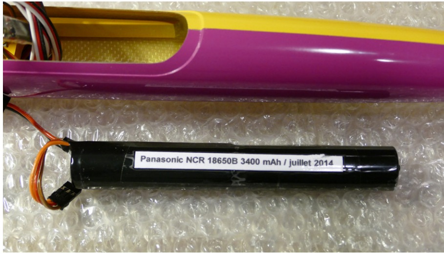
The Lilon 2S format 18650 battery gives a nice flying time despite the very power demanding servos.
