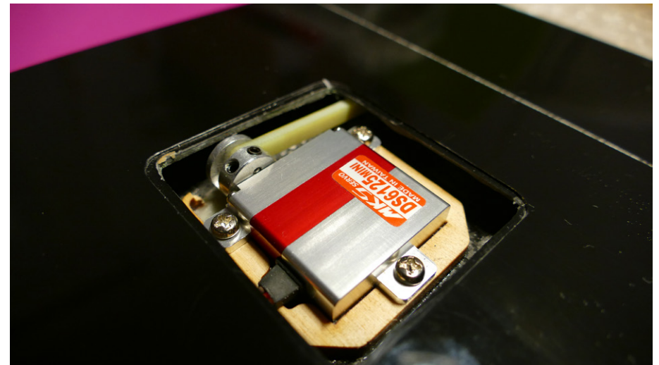
Rotmilan_21: The servo and LDS system in place in the wing. No slop at all !
