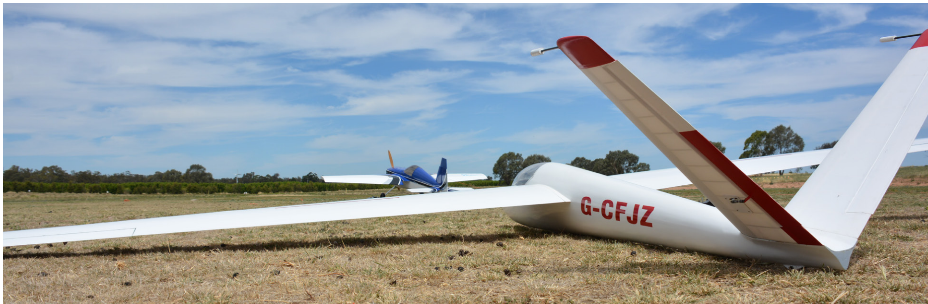
Pilot: Shane Williams with David Hobby's tug , Airframe: SHK Scratch Built 5.7m, 12kg, HQ3013 airfoil
