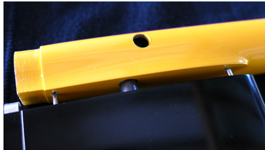
Simple tail plane mounting without any tube, just holes in the fuselage, and where joiners are shifted.
