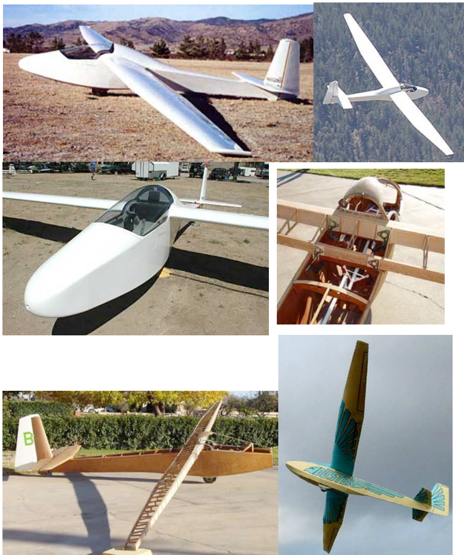
Some pictures of BJ-1B Duster. Developed from BJ-1 DynaMite Somewhat increased span, more reclined seating position.
