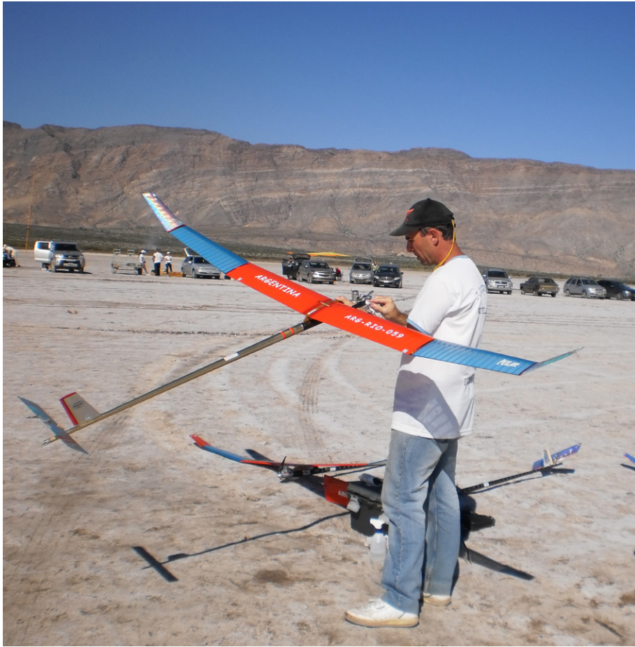
Readying the model for flying. Note the stabilizer tilt, the position it takes when dethermalizing.
