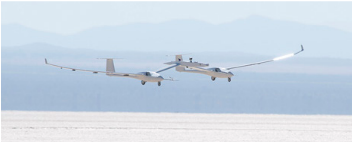
The one-third scale twin-fuselage towed glider glides in for landing on Rogers Dry Lake after its successful first test flight.
