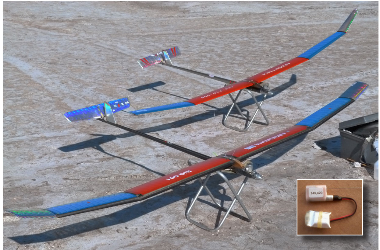
Two of Fernando's F1C models. The beacon mentioned in the test is shown in the inset. Powered by an 70mAh LiPo battery, it will transmit a signal for 15 days. The model in the background is the one which was temporarily lost.
