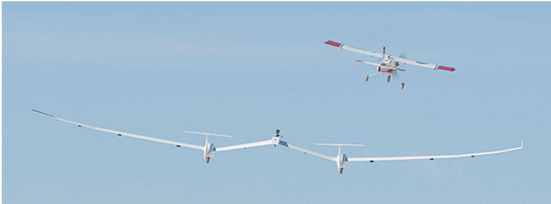
One of NASA Armstrong's DROID small unmanned research aircraft tows the twin-fuselage towed glider into the blue sky on its first test flight.
