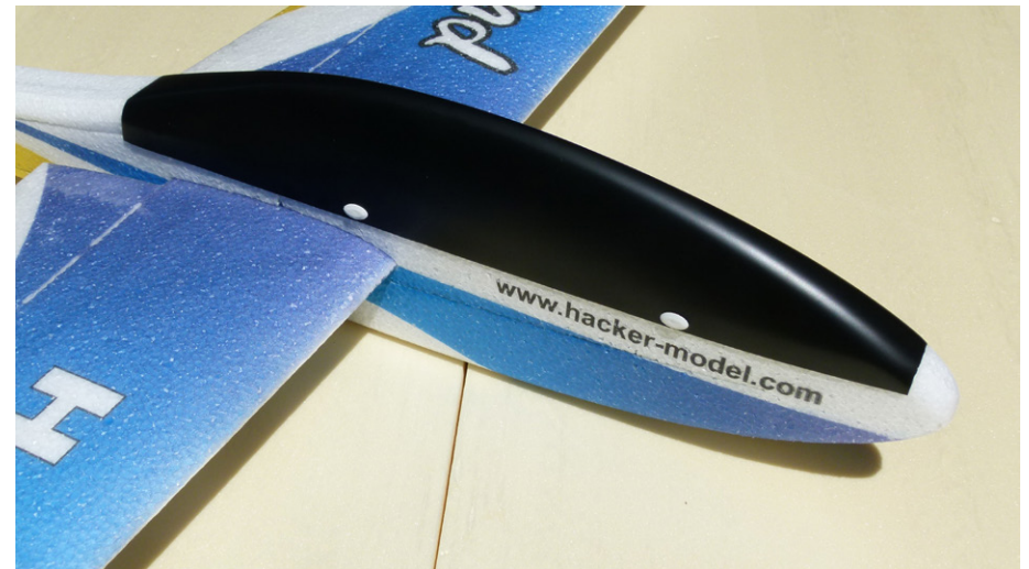
The canopy is locked with four plastics clips. These clips are glued on the canopy to not loose them.
