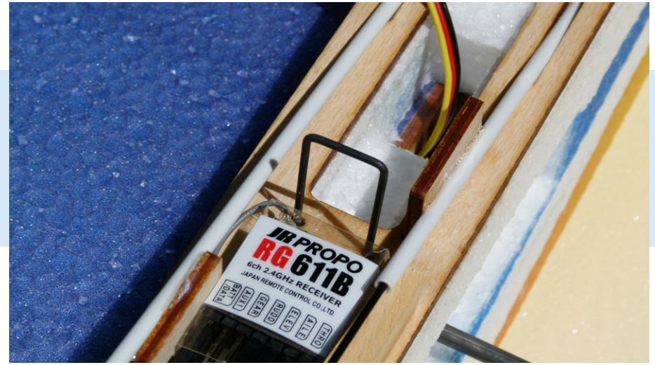
The wing lock system is brilliant. This is an inverted U-shape piano wire that passes behind the root of each wing. Simple and efficient.
