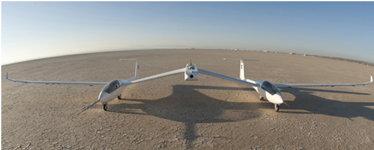
The one-third-scale twin fuselage towed glider rests of the cracked bed of Rogers Dry Lake at Edwards Air Force Base prior to its first flight Oct. 21, 2014 in this photo shot with a 16-mm. fisheye lens.
