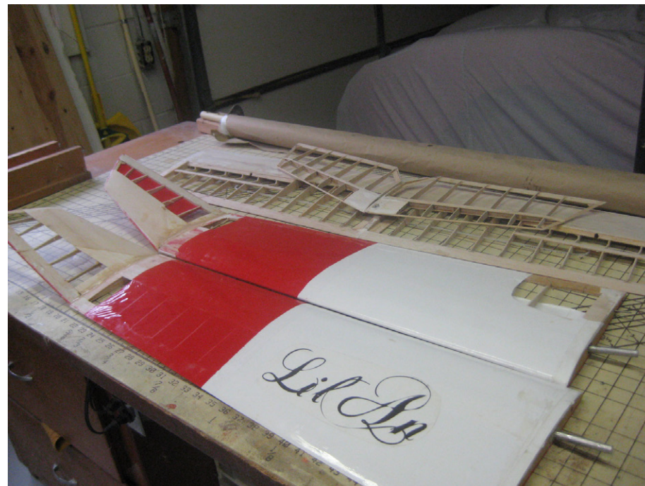
Photo 10: Wing repaired complete, waiting for recovering.
