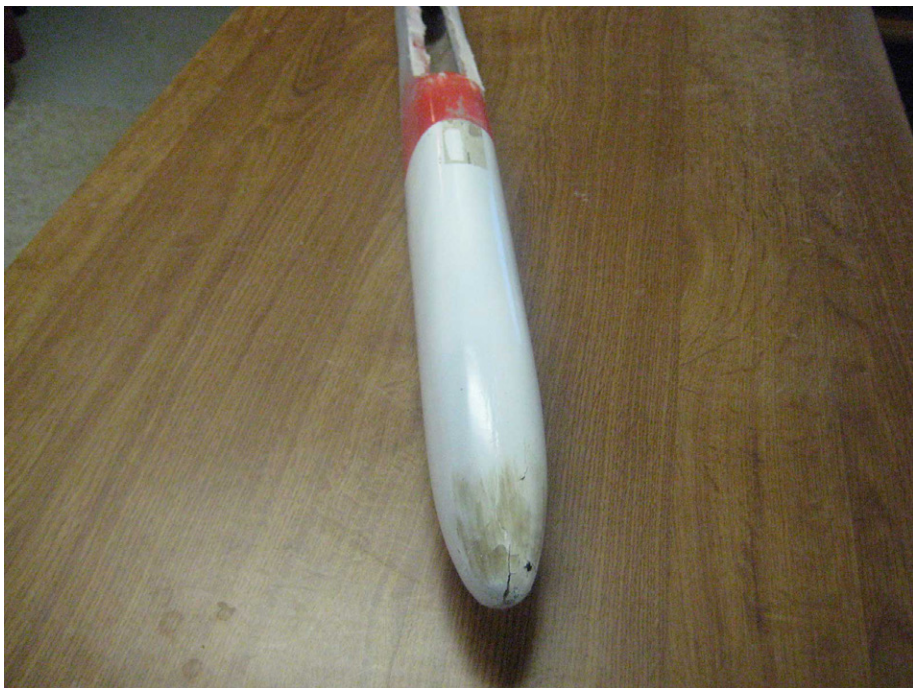
Photo 7: Nose cone damage.
