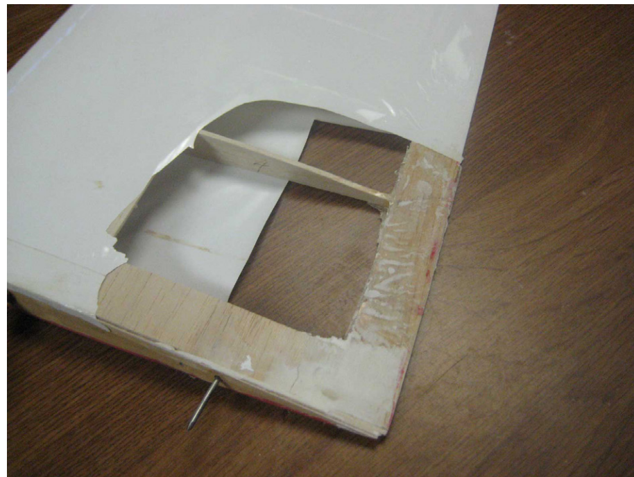
Photo 8: Right wing panel root repair.
