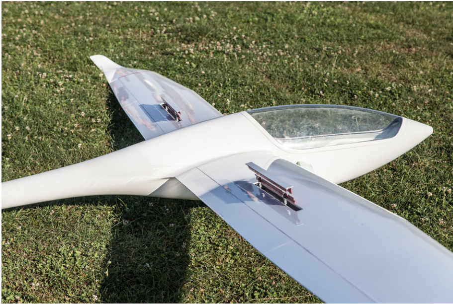
Spoilers 500mm from German manufacturer Schambeck < http://www.klapptriebwerk.de >.
