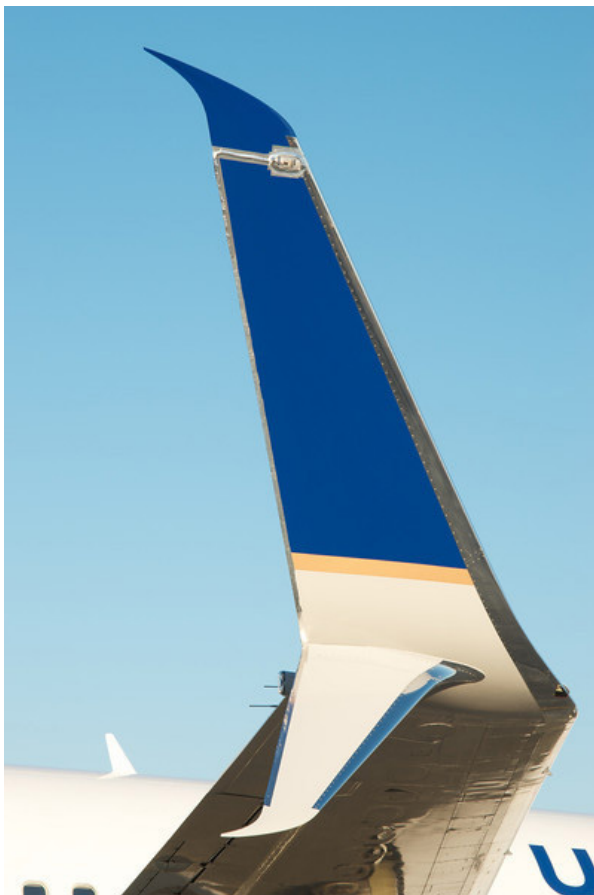
A pre-certified Split Scimitar Winglet installed on a United Boeing 737-800 during the testing phase that began July 2013.
