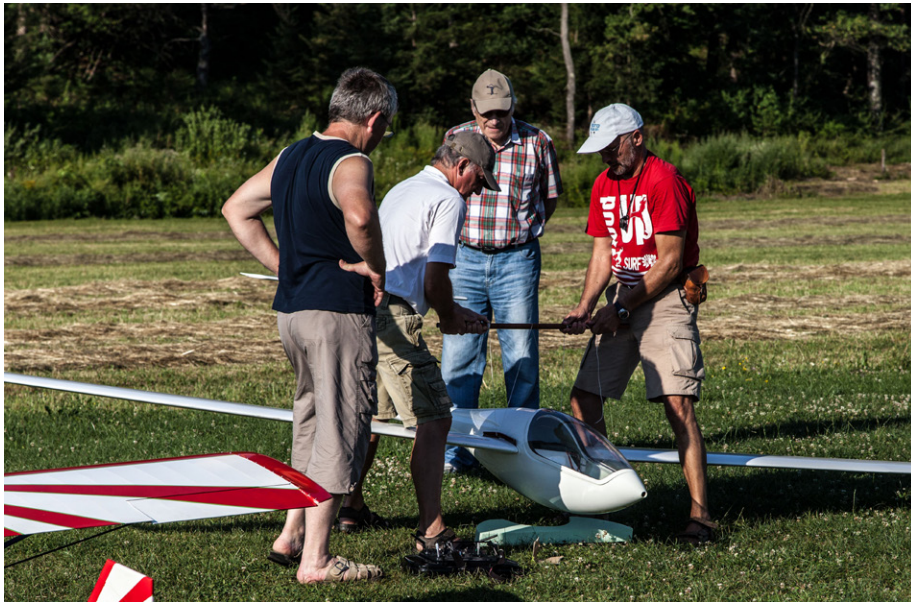
Checking center of gravity before first flight.
