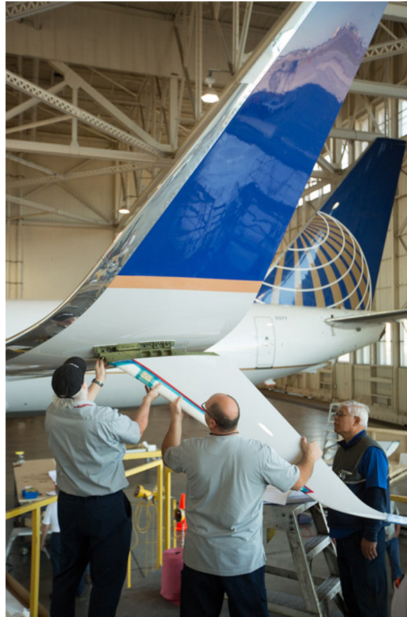
Retrofitting Blended Winglets to Split Scimitars involves adding strengthening spars, aerodynamic “scimitar tips,” and a large ventral strake.
